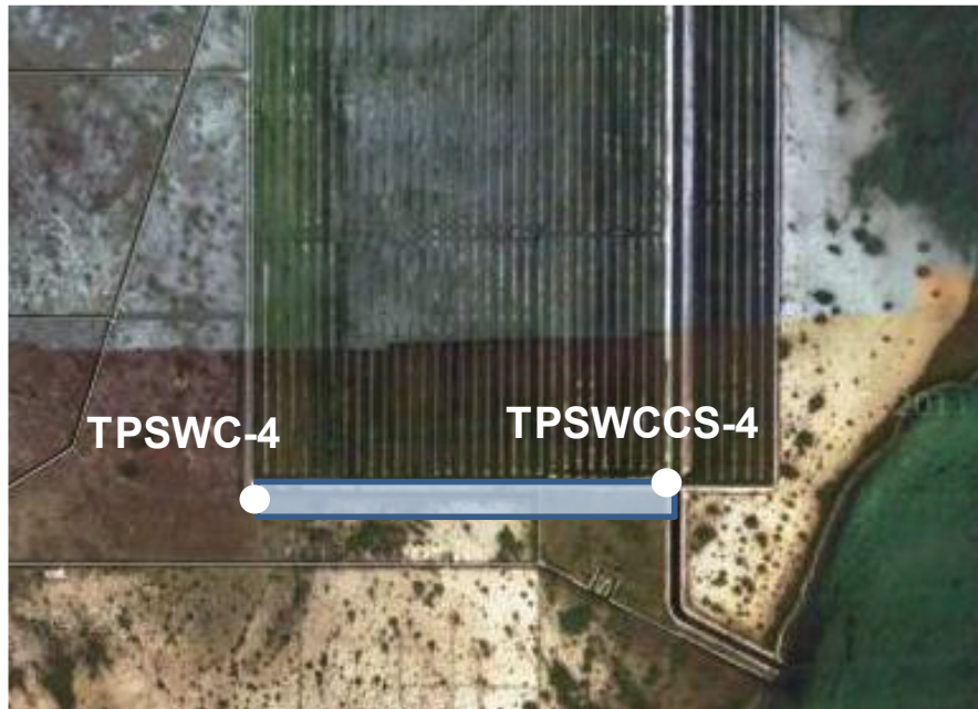
Figure 5.4-4. Locations of TPSWCCS-4 and TPSWC-4 Monitoring Stations; Conceptualized Seepage from Southern Collector Canal into the CCS is Shown.
