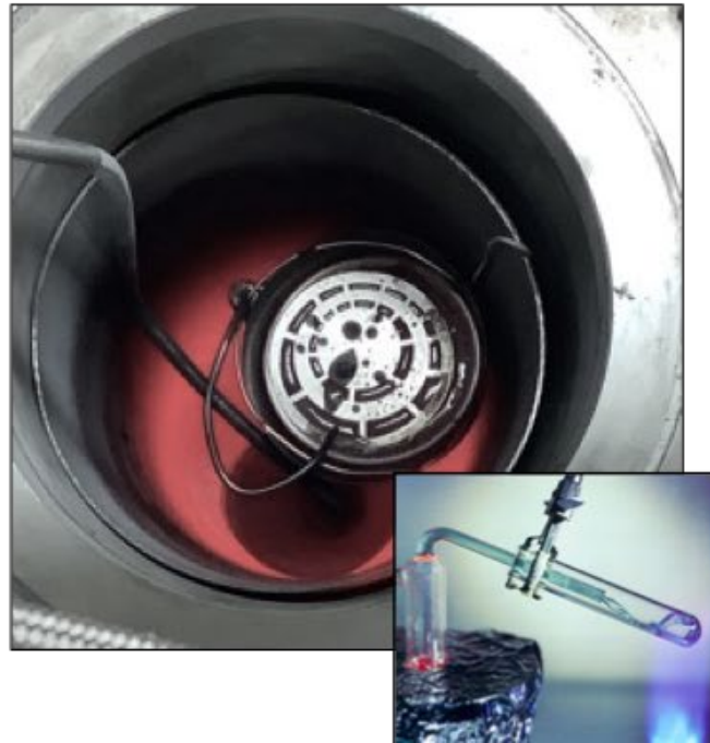
Liquid Fluoride Salt Coolant Flibe (2LiF-BeF 2 )
