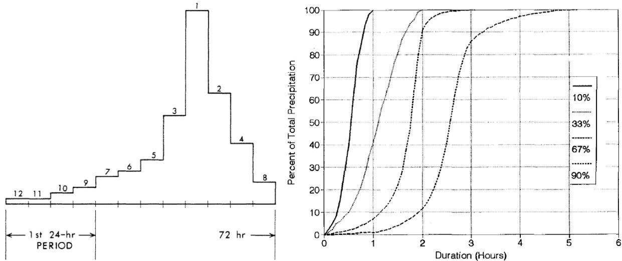
**Figure 9-2 Example Temporal Distribution for a Watershed-Scale 72-h PMP Event Provided in HMR No. 52 (Left; Hansen et al. 1982) and Example Temporal Distributions for Middle-Loaded Local-Scale Storms Provided in HMR No. 57 (Right; Hansen et al. 1994)**
