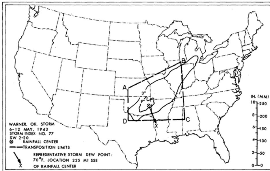
Figure 4-1 HMR Transposition Limit Map for May 1943 Warner, OK, Storm (from HMR No. 51)
