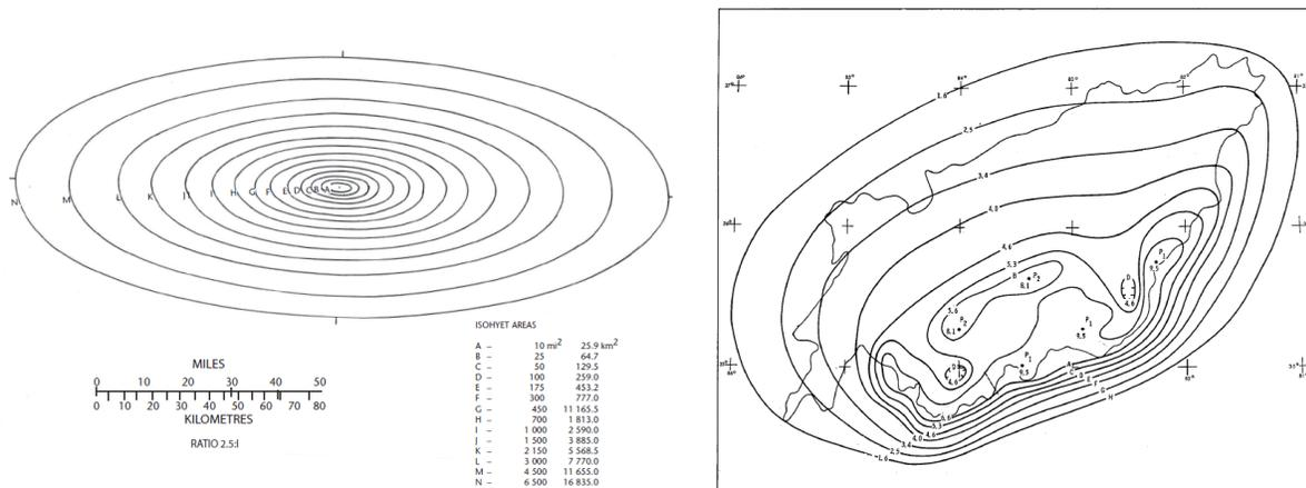
**Figure 9-1 Standard Isohyetal Spatial Distribution Pattern Recommended in HMR No. 52 (left; Hansen et al. 1982 as Included in WMO 2009) and Example Probable Maximum March Isohyets Provided in HMR No. 41 (right; Schwarz 1965)**
