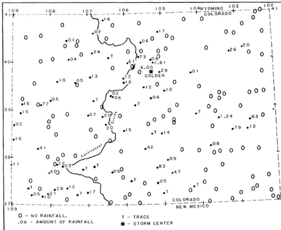
**Figure 3-1 Map of Precipitation Gauge Data for June 1948 Golden, CO, Storm (from HMR No. 55A)**
