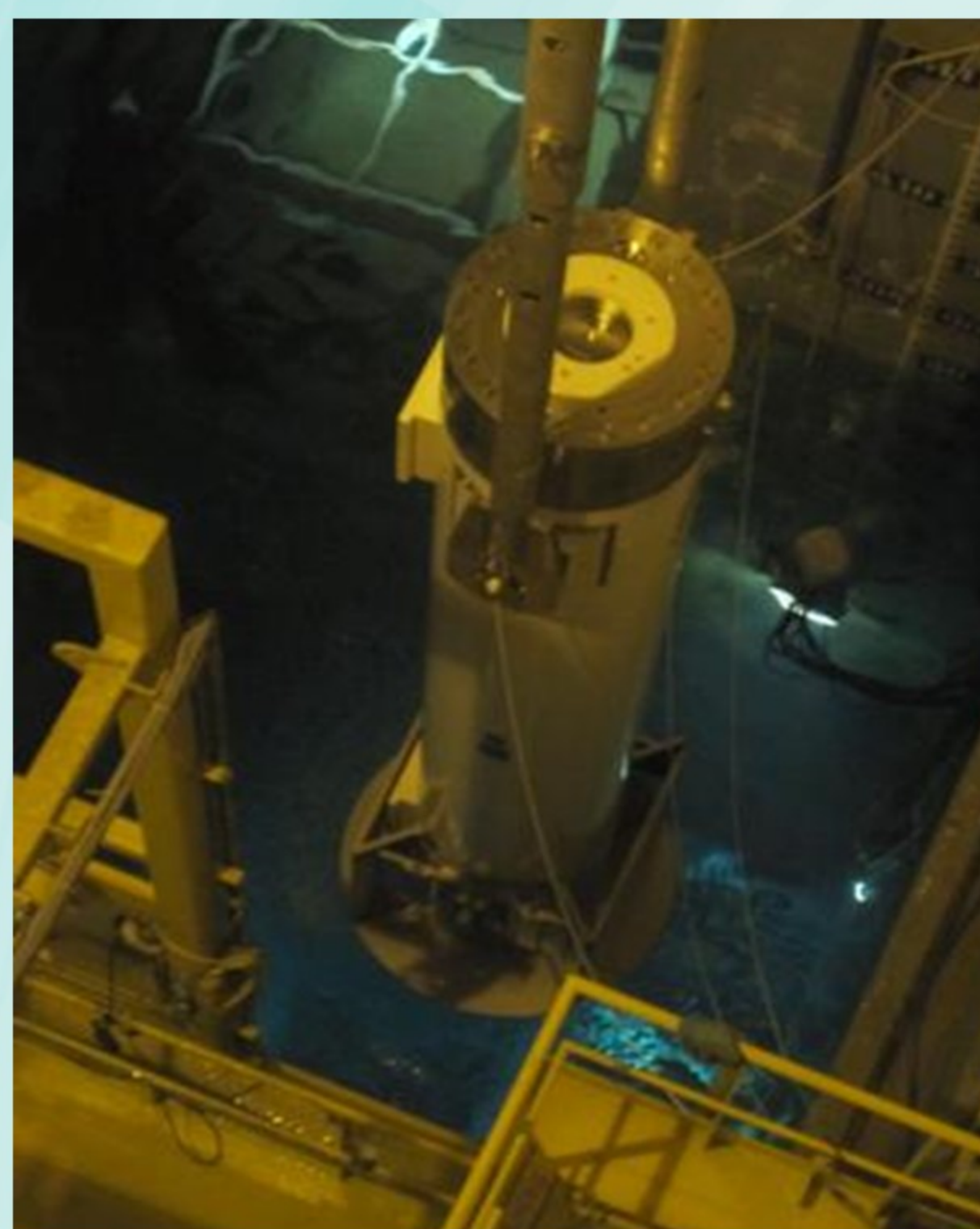
Lifting operation for irradiated materials transport cask
