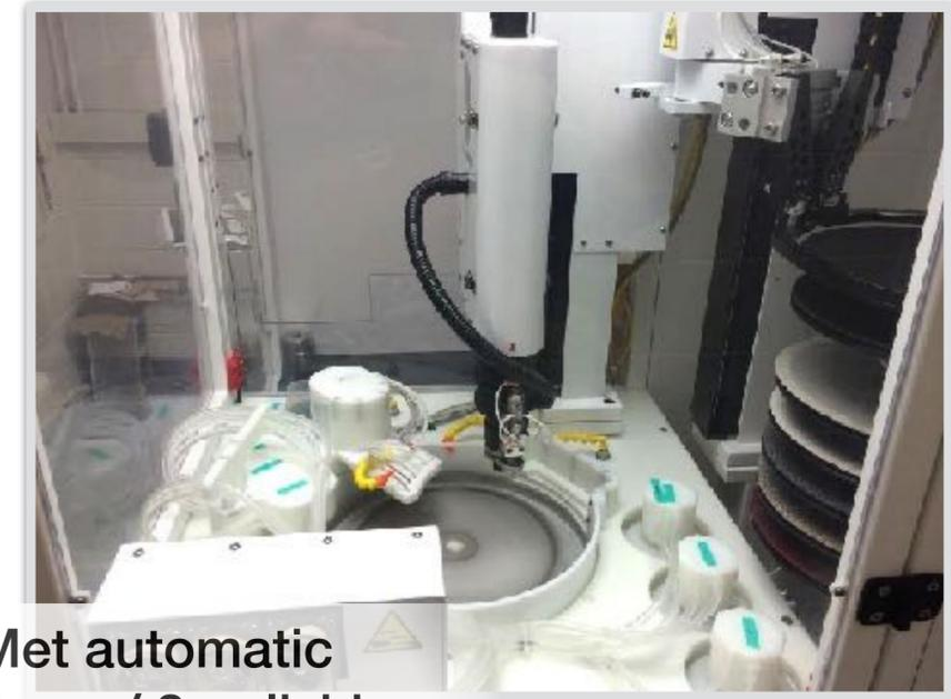
RoboMet automatic polishing w/ 8 polishing pads, ultra sonic cleaning, two etching stations.
