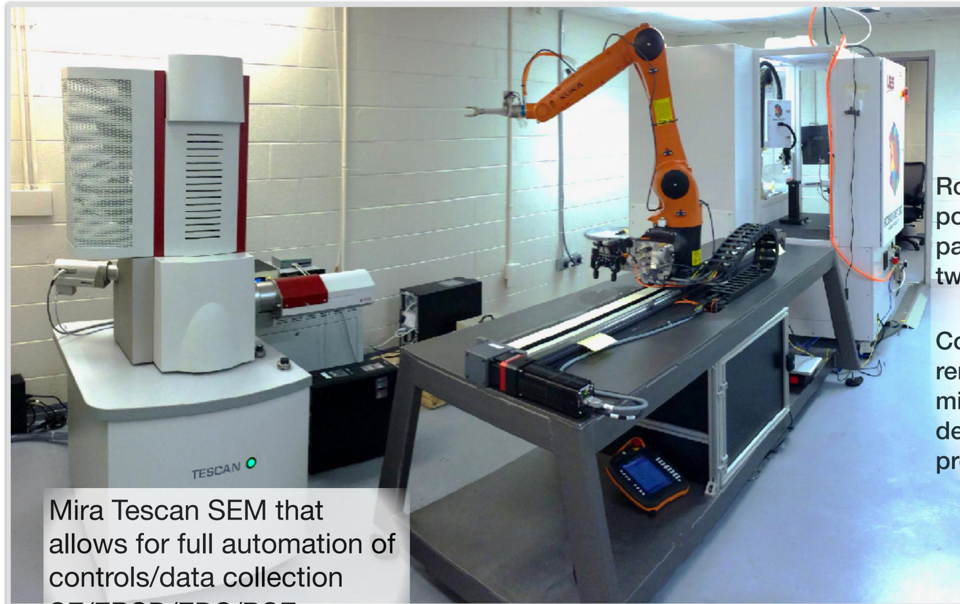
Mira Tescan SEM that allows for full automation of controls/data collection SE/EBSD/EDS/BSE...
