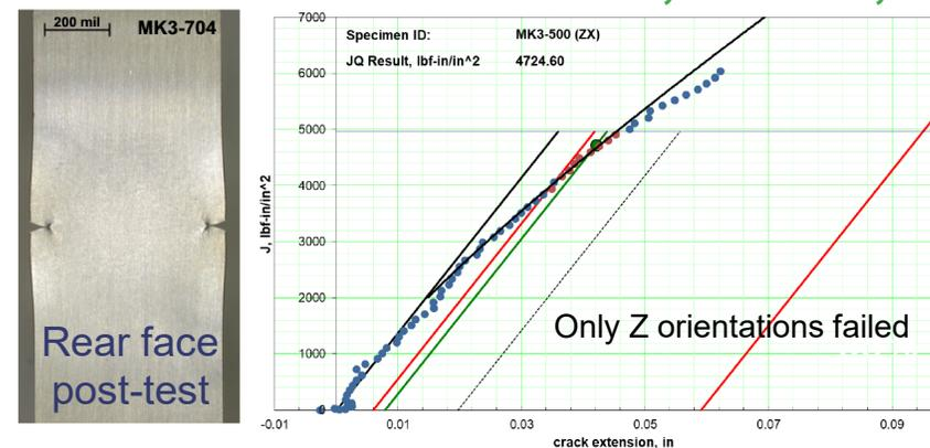
Maximum J-integral capacity was exceeded, thickness and initial ligament  $< 10 J_Q/\sigma_Y$
