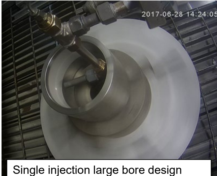
Single injection design for use with carbide nozzle • 1.8 in minimum bore, 0.5" standoff
