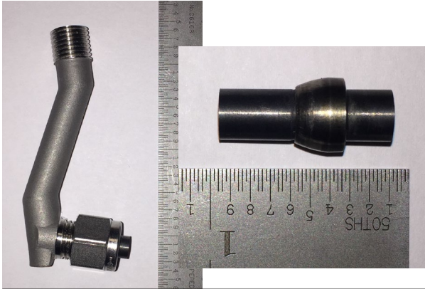
Single injection design for use with carbide nozzle • 1.8 in minimum bore, 0.5" standoff
