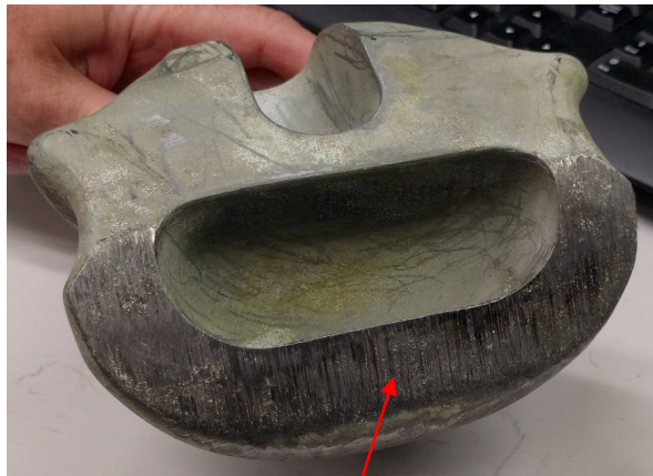
Surface wear due to adhesive/abrasive wear
