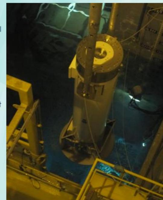
Lifting operation for irradiated materials transport cask
