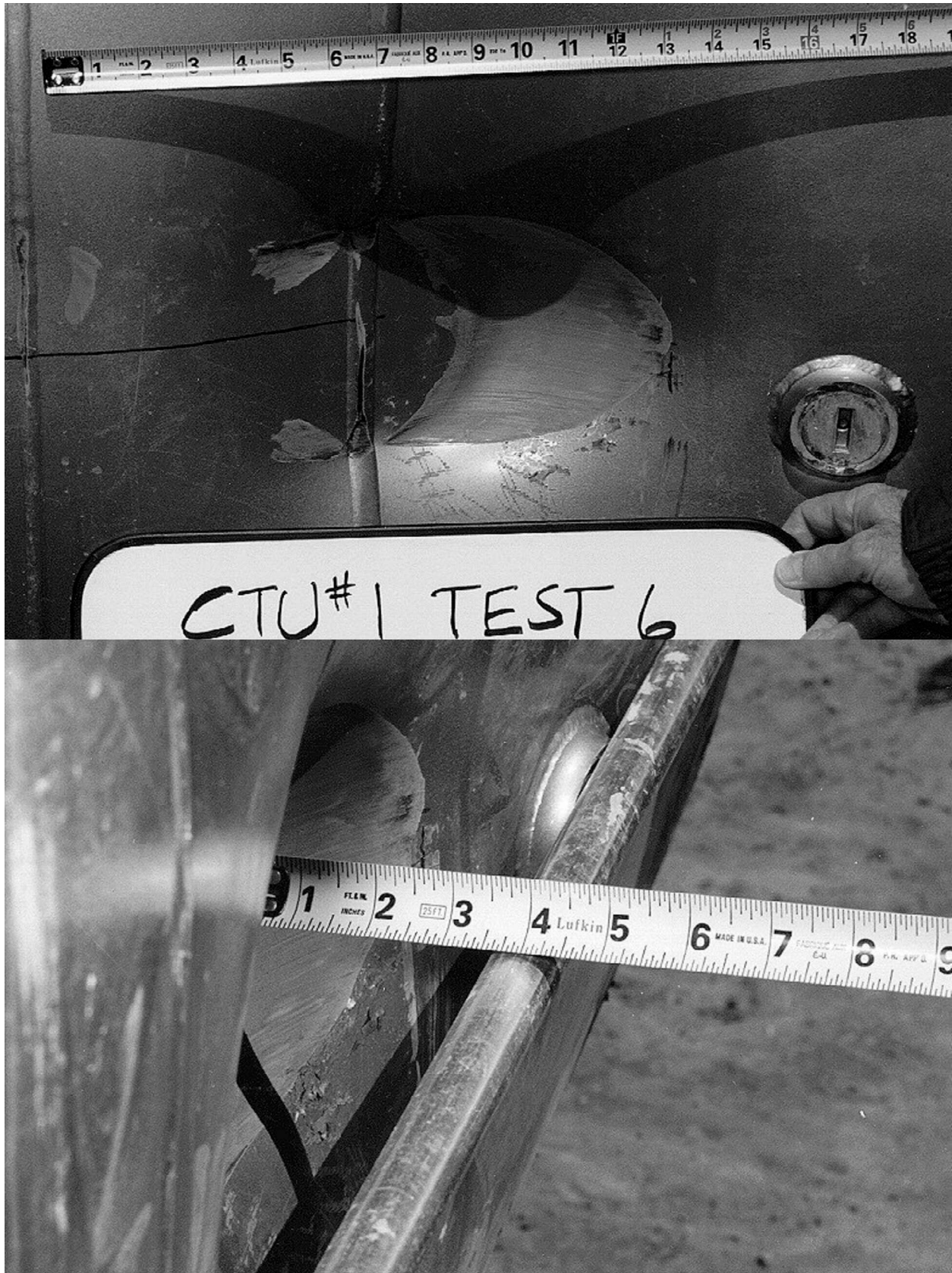
Figure 2.10.3-68 – CTU Puncture Drop Test 6; Close-up Views of Damage; ~3½" Deep
