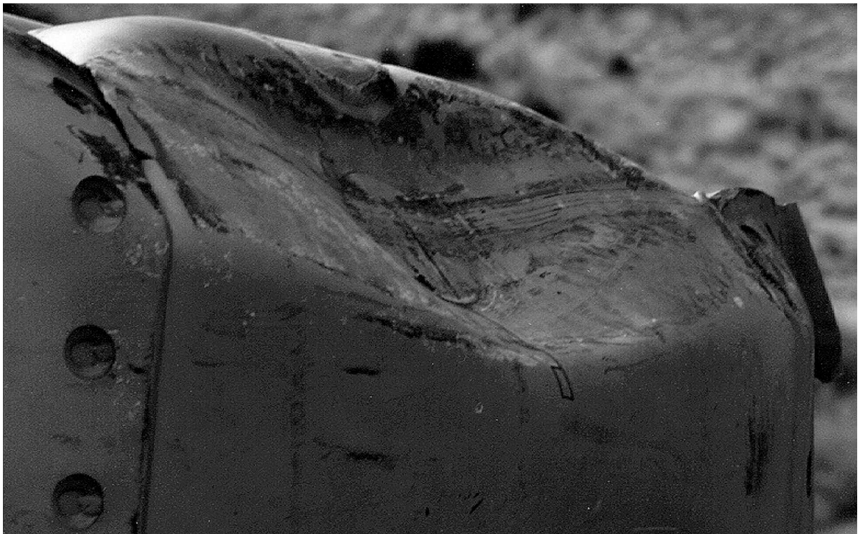
Figure 2.10.3-29 – ETU Puncture Drop Test 9; Bottom Corner Damage; ~3" Deep Dent
