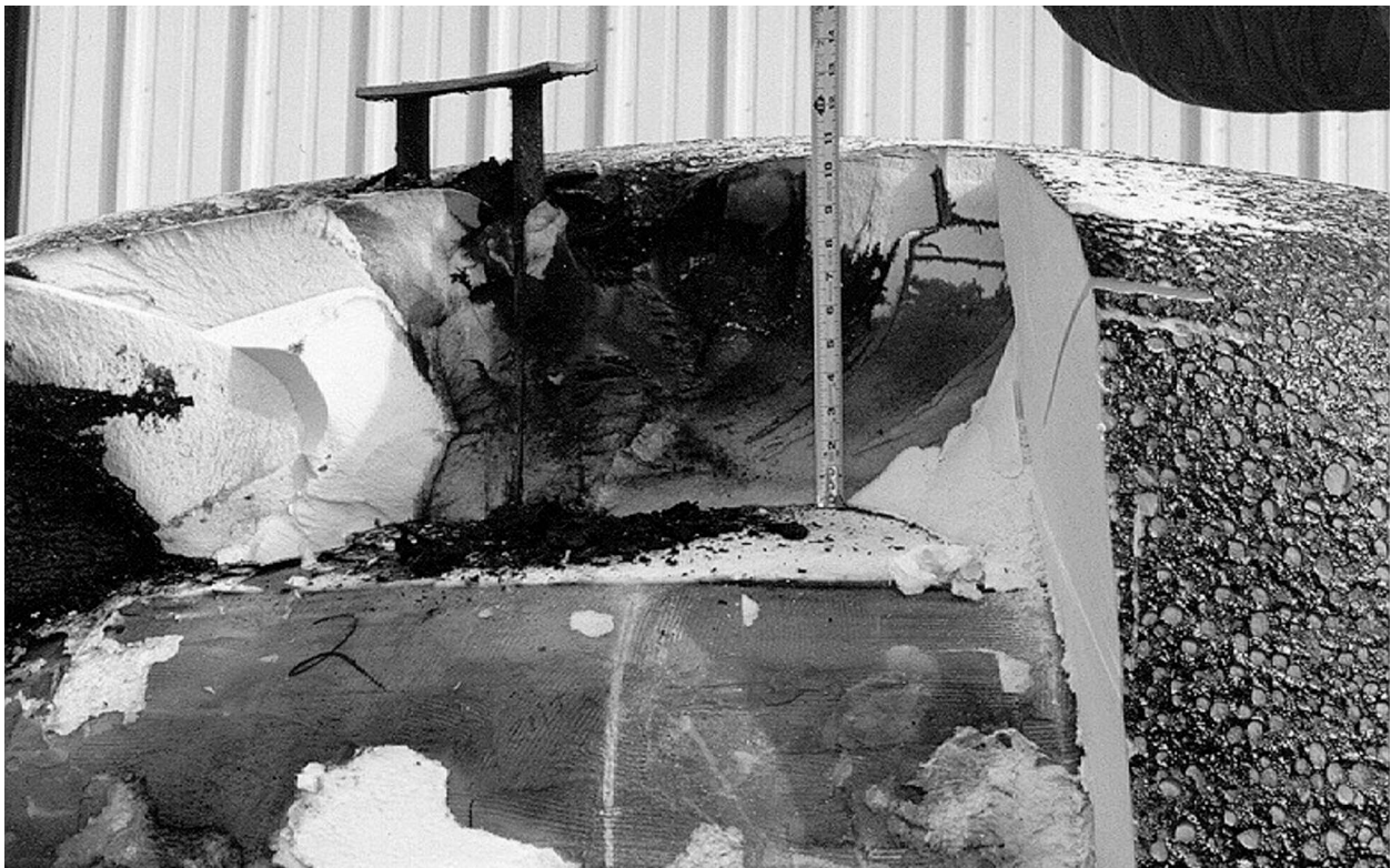
Figure 2.10.3-44 – ETU; Residual Foam in OCA Lid Top (~11")
