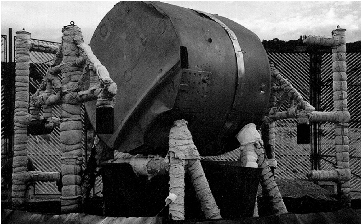
Figure 2.10.3-33 – ETU Fire Test 11; Side 2 View Showing Tests 3, 4, 5, 6, 8, & 9 Damage
