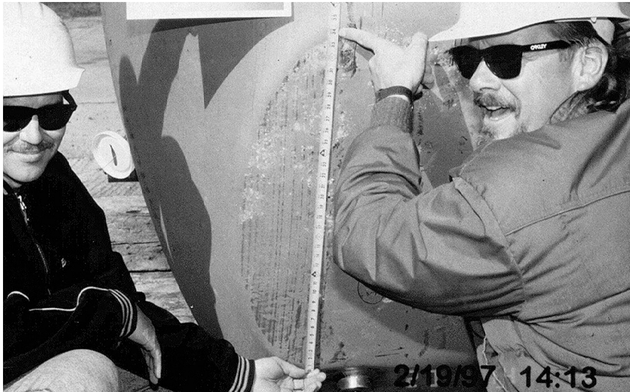
Figure 2.10.3-18 – ETU Free Drop Test 4; Top-End Damage; ~34" Wide Flat
