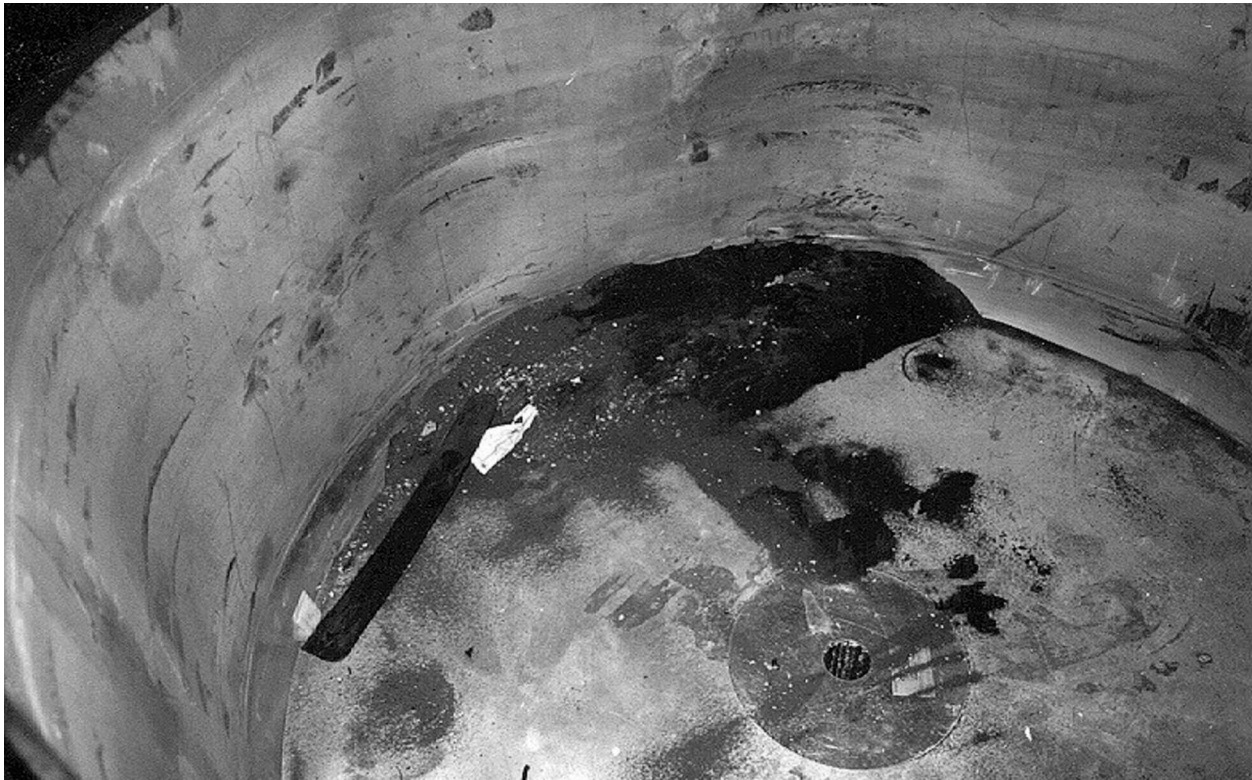
Figure 2.10.3-50 – ETU; View of Debris Inside ICV Body Cavity After Payload Drum Removal
