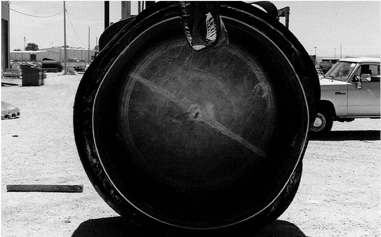
Figure 2.10.3-89 – CTU; End View of OCV Cavity Showing Deformed Lower Seal Flange
