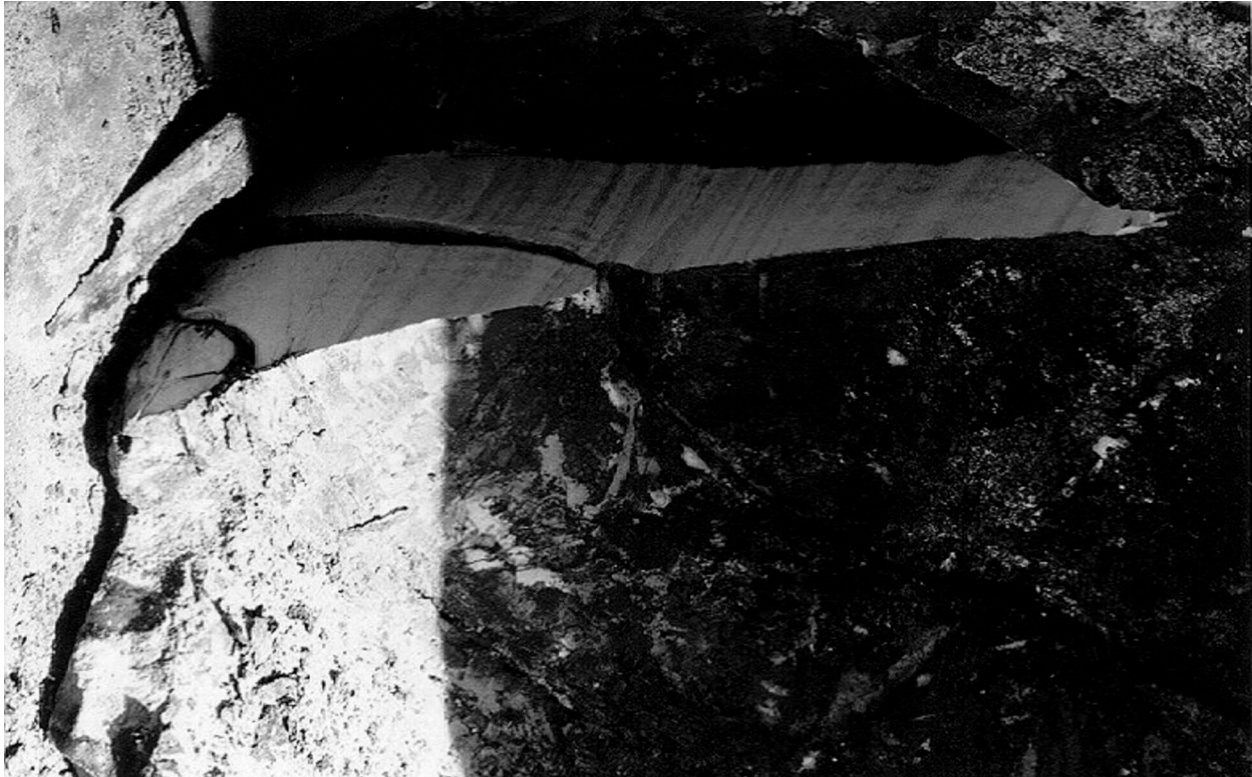
Figure 2.10.3-90 – CTU; Residual Foam in OCA Lid Side; Aligned with Test 1, 2, & 4 Damage
