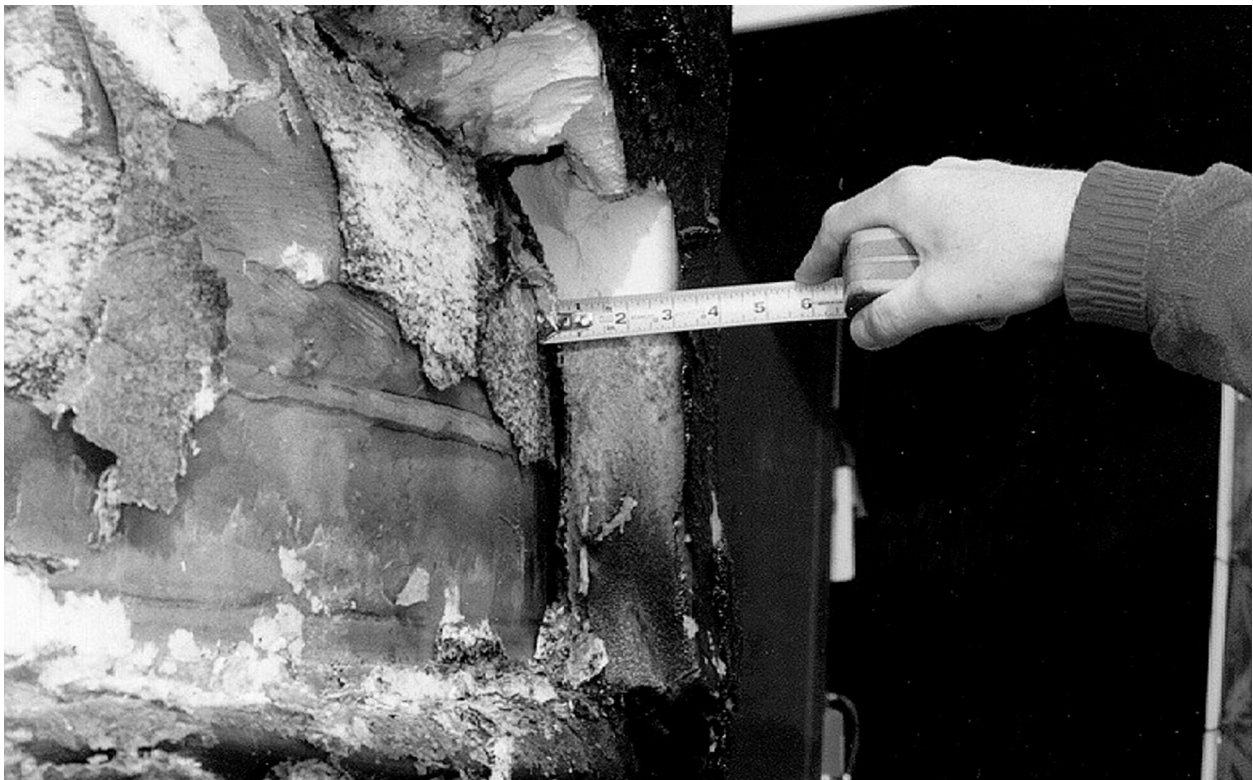
Figure 2.10.3-42 – ETU; Residual Foam in OCA Lid Side; Aligned with Test 1, 2, & 7 Damage
