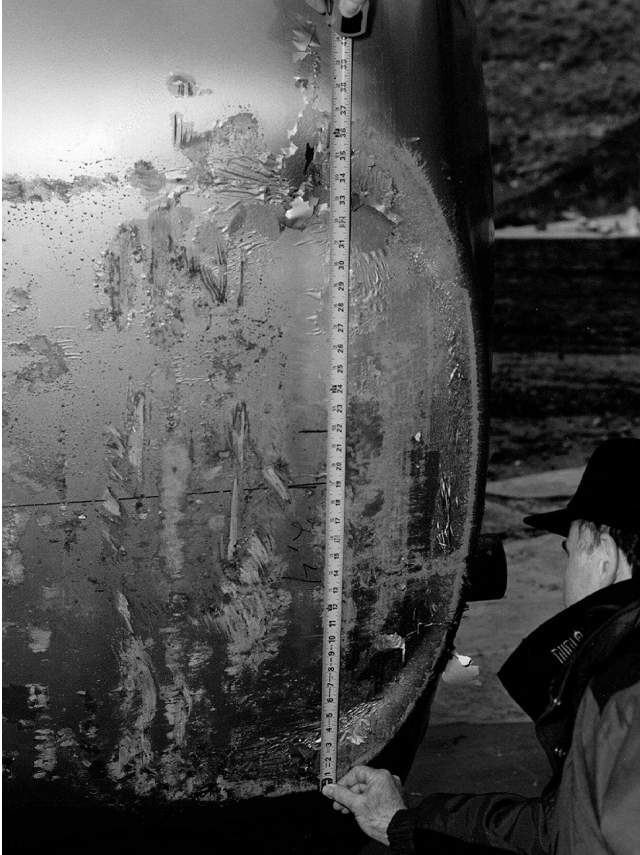
Figure 2.10.3-58 – CTU Free Drop Test 2; Lid-End Damage; ~37" Wide Flat
