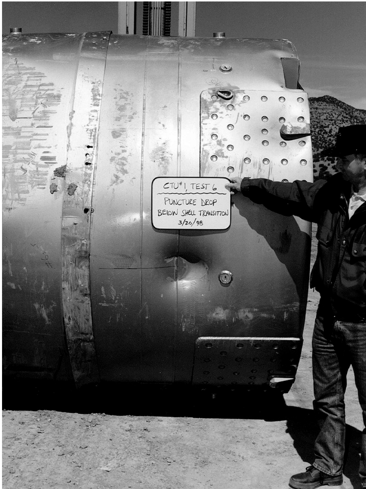
Figure 2.10.3-67 – CTU Puncture Drop Test 6; Overall View of Damage
