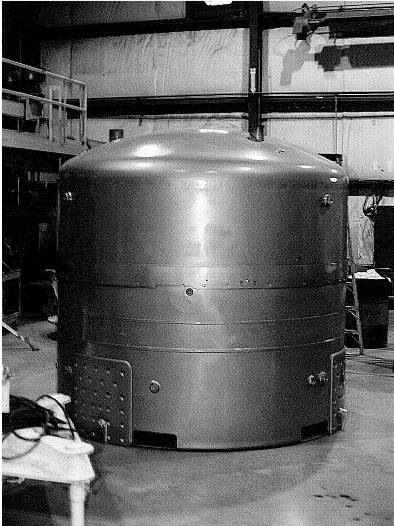
Figure 2.10.3-55 – CTU; Certification Test Unit (TRUPACT-II Unit 107) After Final Assembly
