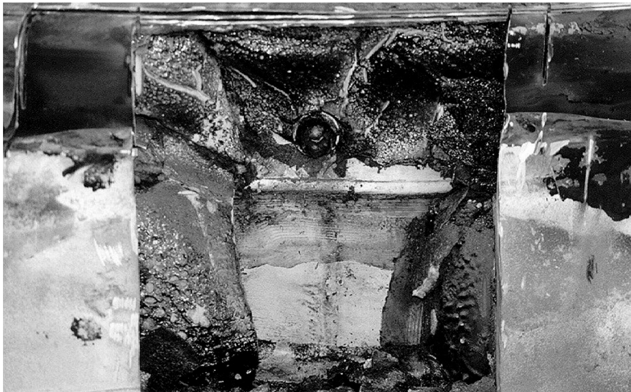
Figure 2.10.3-85 – CTU; OCV Vent Port Region After Removing Excess Foam Char
