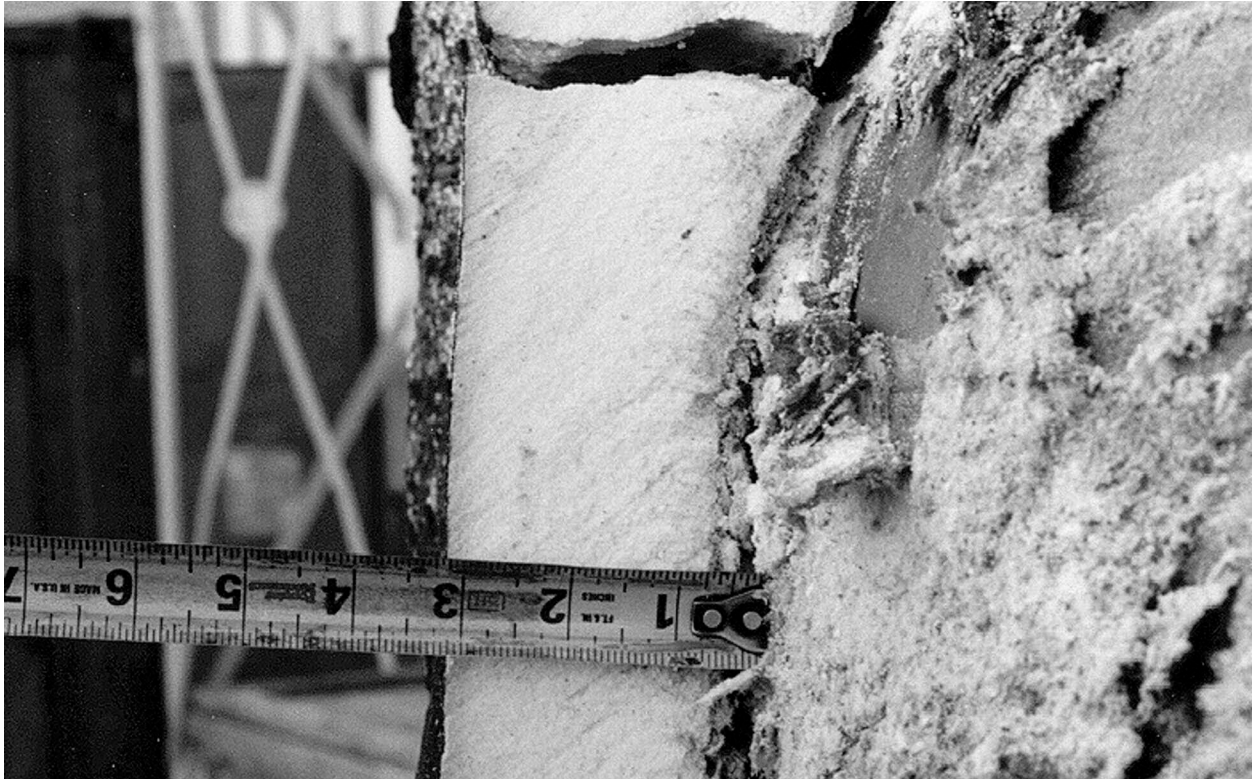
Figure 2.10.3-80 – CTU; Residual Foam in OCA Lid Side; Aligned with Test 1, 2, & 4 Damage
