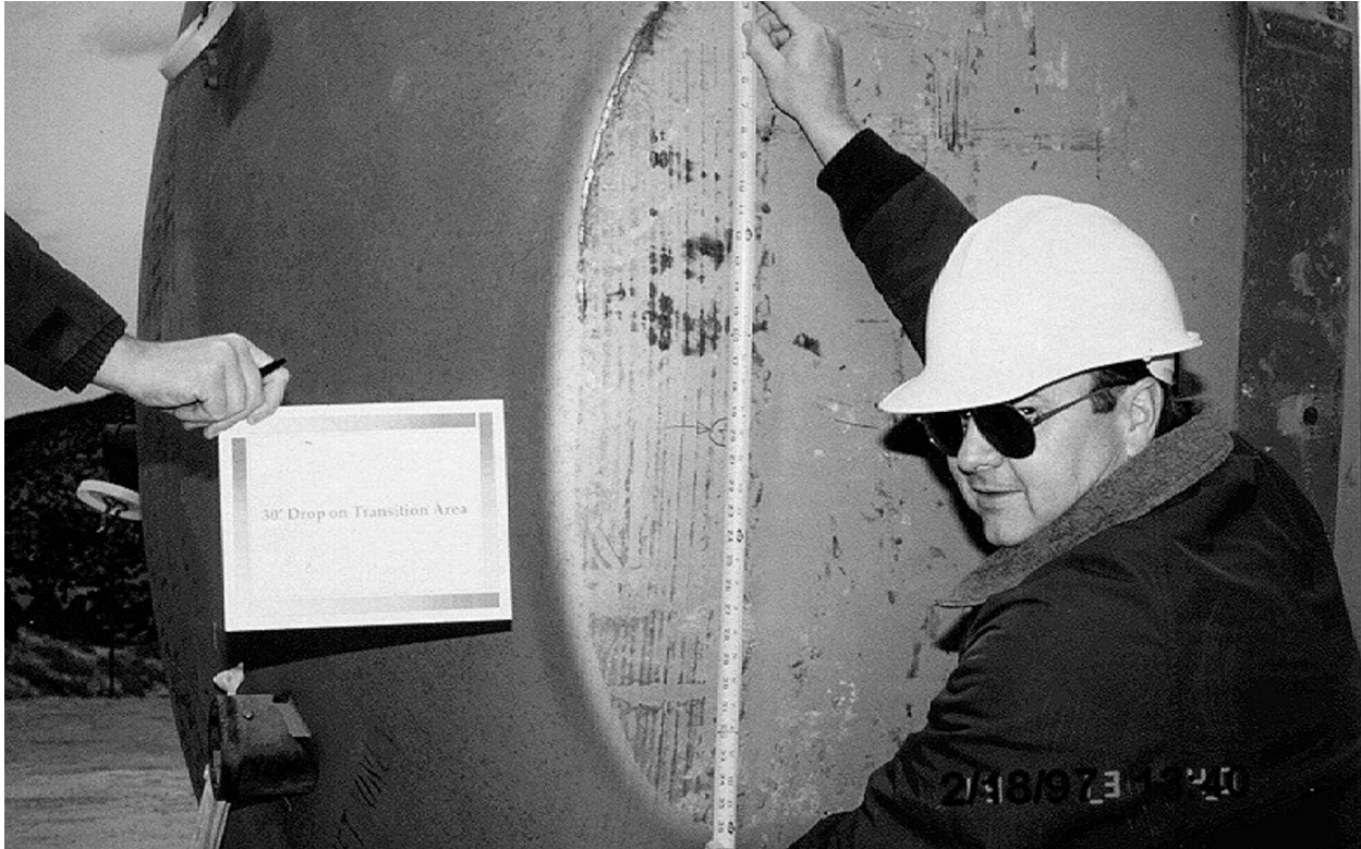
Figure 2.10.3-14 – ETU Free Drop Test 2; Top-End Damage; ~36" Wide Flat
