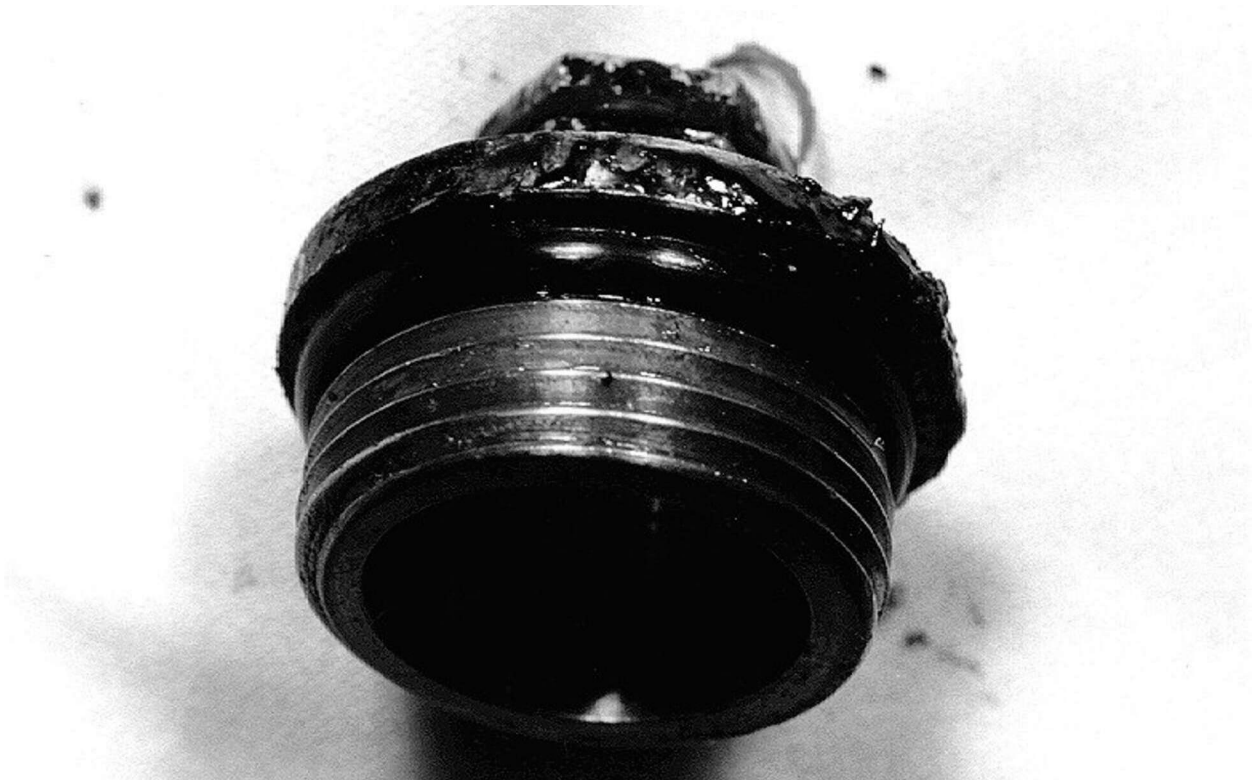
Figure 2.10.3-46 – ETU; View of OCV Vent Port Cover (As Removed; Not Cleaned)
