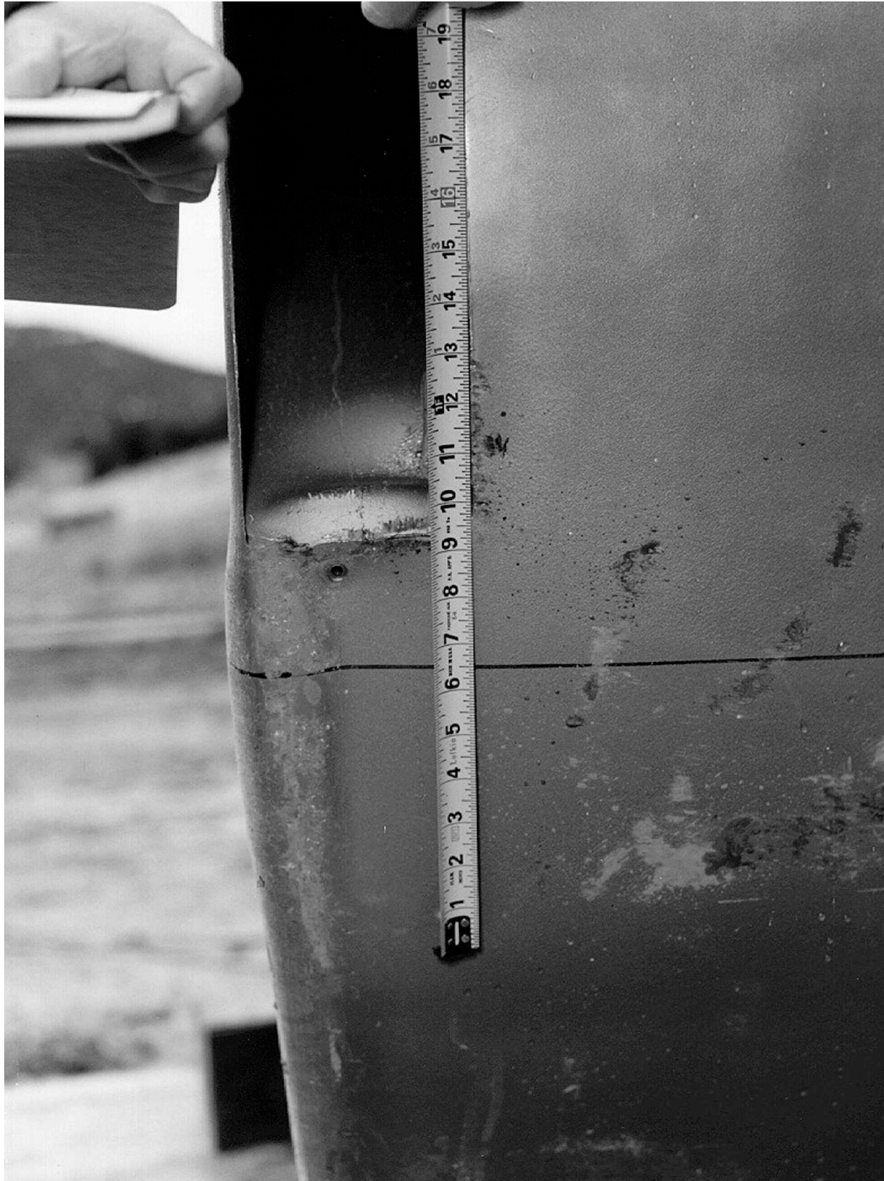
Figure 2.10.3-57 – CTU Free Drop Test 1; Bottom-End Damage; ~13" Wide Flat
