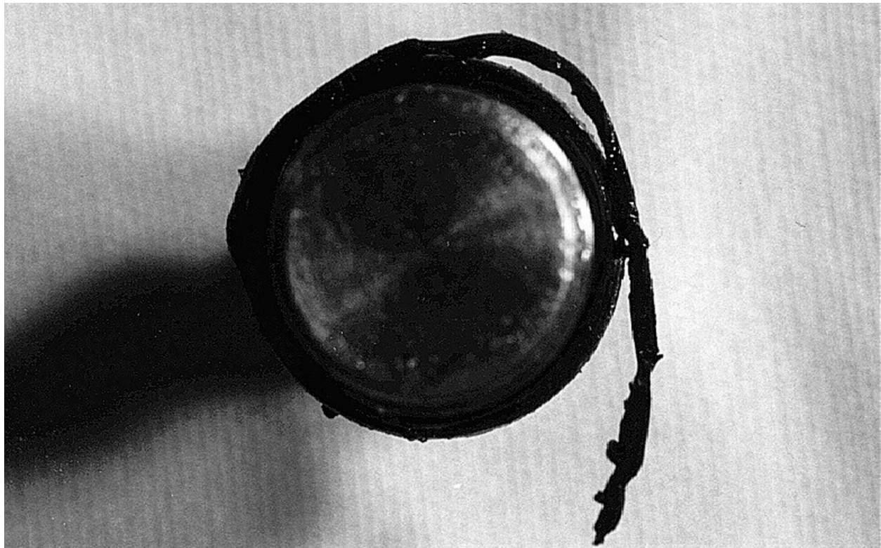
Figure 2.10.3-47 – ETU; View of OCV Vent Port Plug (As Removed; Not Cleaned)
