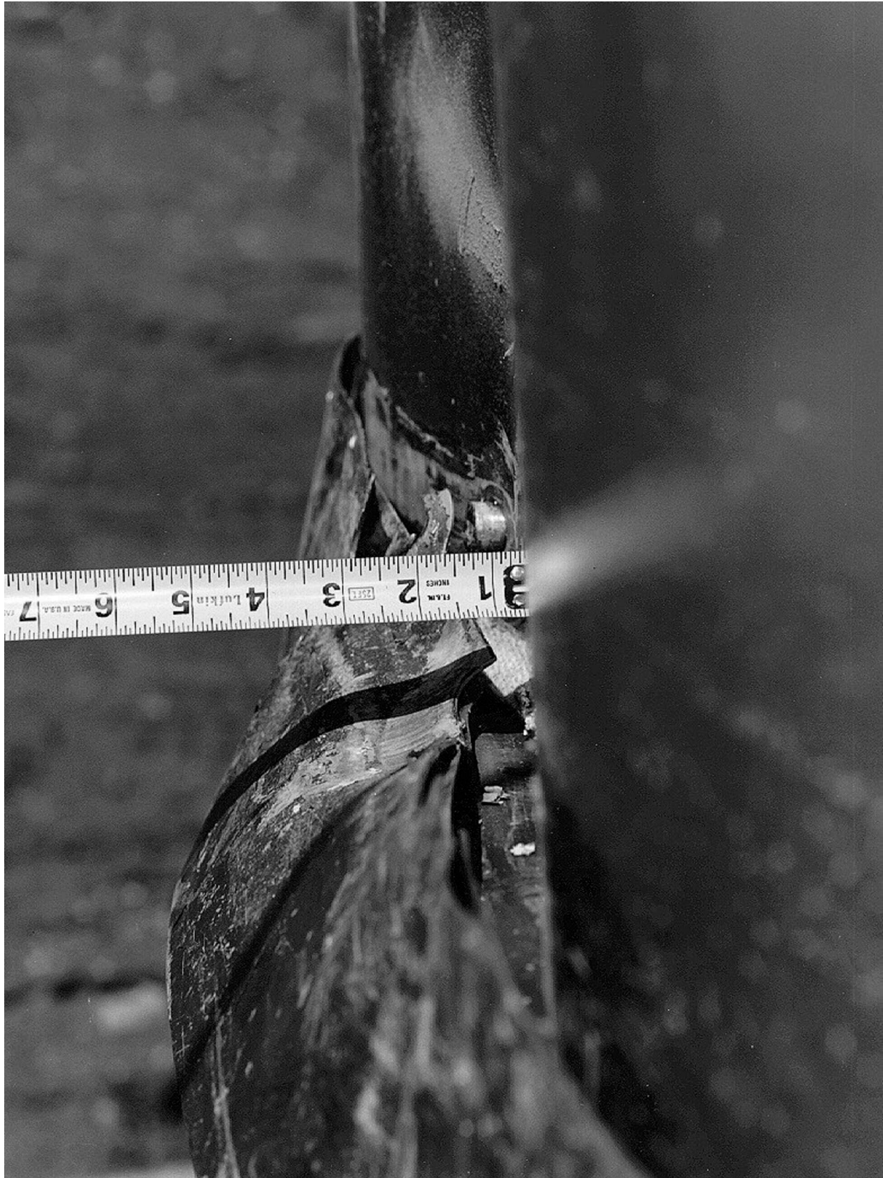
Figure 2.10.3-64 – CTU Puncture Drop Test 4; Close-up Profile View of Damage; \sim 3\frac{3}{4} " Deep
