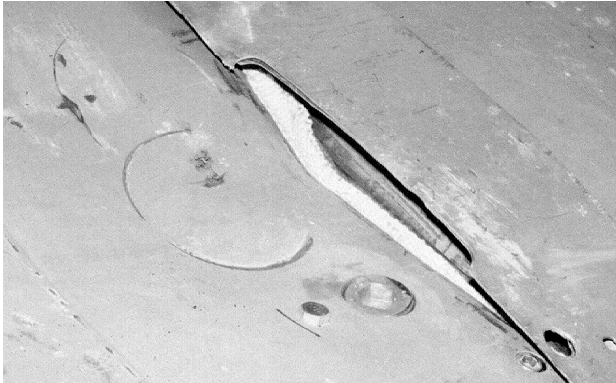
Figure 2.10.3-27 – ETU Puncture Drop Test 8; Close-up View of Damage; ~2½" Deep Dent
