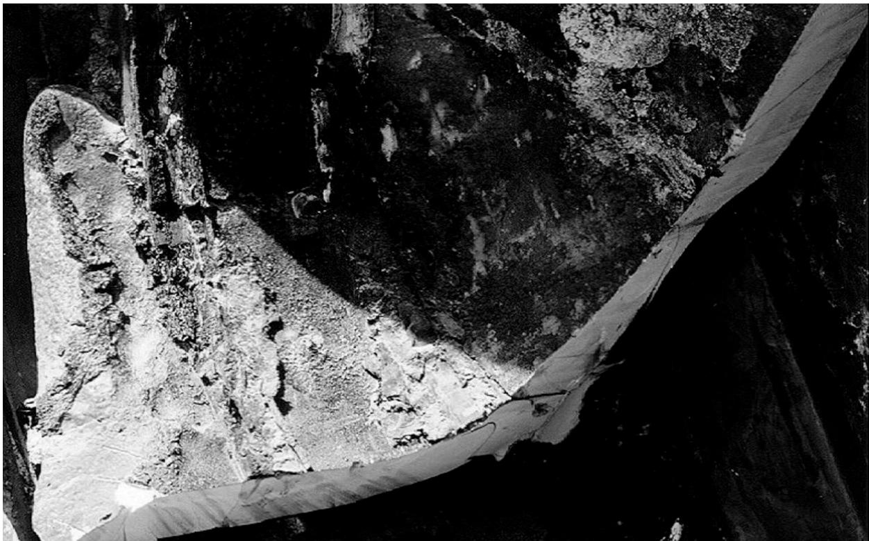
Figure 2.10.3-91 – CTU; Residual Foam in OCA Body Side; Remote from Test Damage
