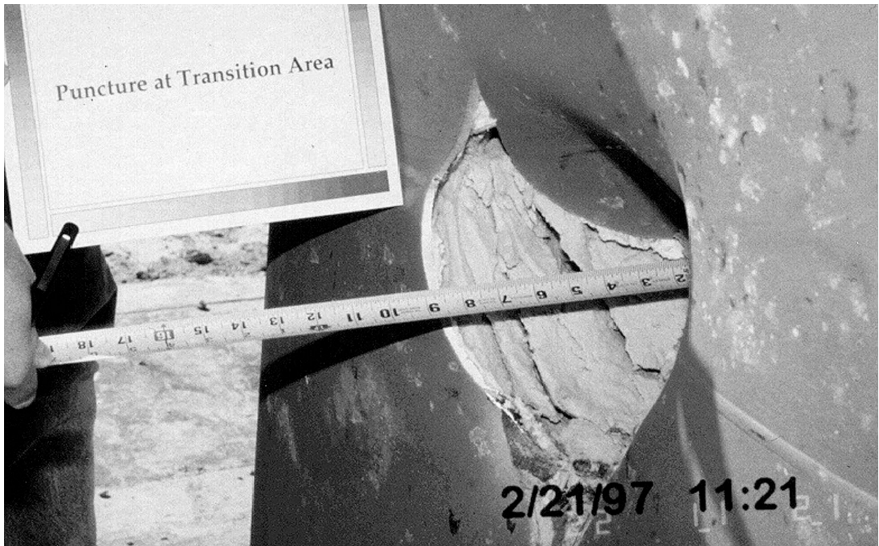
Figure 2.10.3-25 – ETU Puncture Drop Test 7; Radial Penetration ~8" Deep
