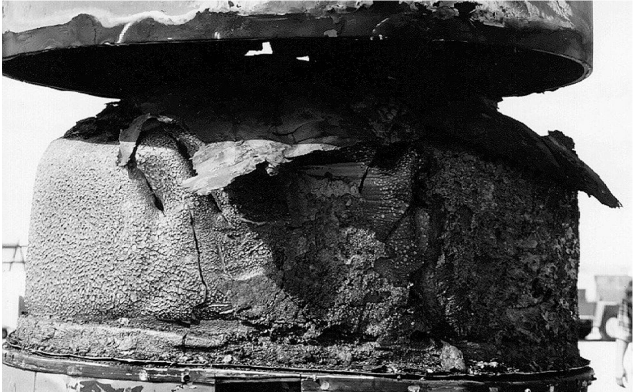
Figure 2.10.3-41 – ETU; Removal of the OCA Lid Outer Shell (Note Crumbling Foam Char)
