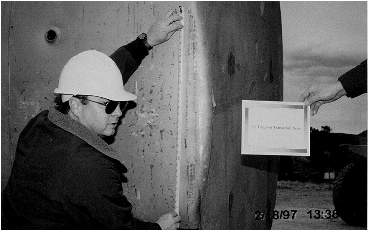
Figure 2.10.3-15 – ETU Free Drop Test 2; Bottom-End Damage; ~33" Wide Flat
