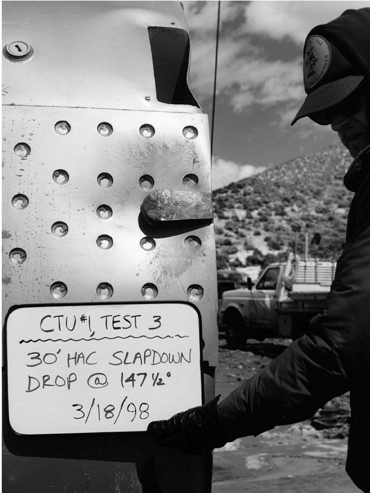
Figure 2.10.3-61 – CTU Free Drop Test 3; Bottom-End Damage
