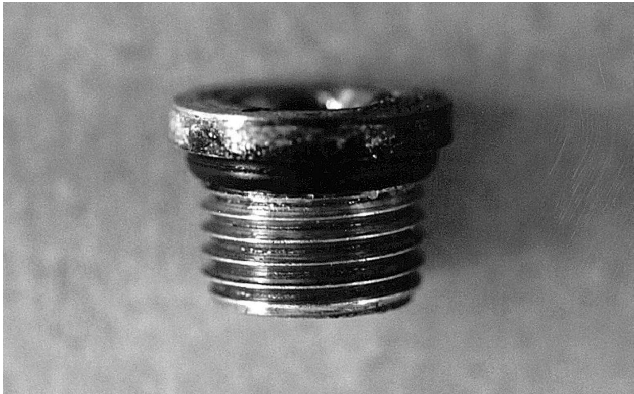
Figure 2.10.3-84 – CTU; Close-up of OCV Seal Test Port Plug (As Removed/Not Cleaned)
