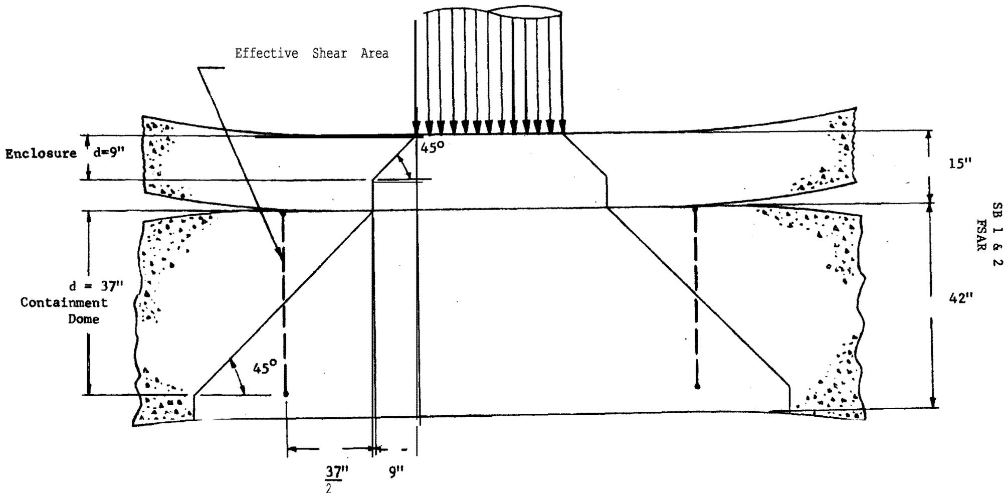
FIGURE 24 SCHEMATIC FOR EFFECTIVE SHEAR AREA - CONTAINMENT
