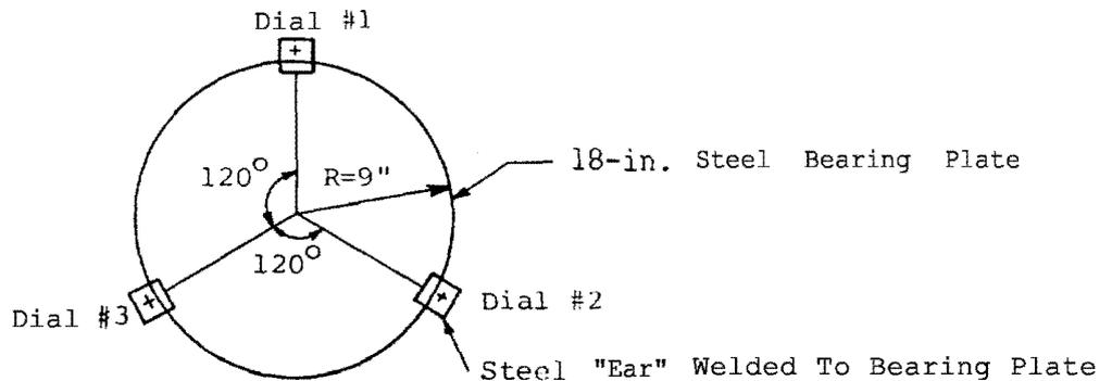
Dial indicators #1, #2, and #3 monitored displacement of "ears" attached to circumference of bearing plate.
