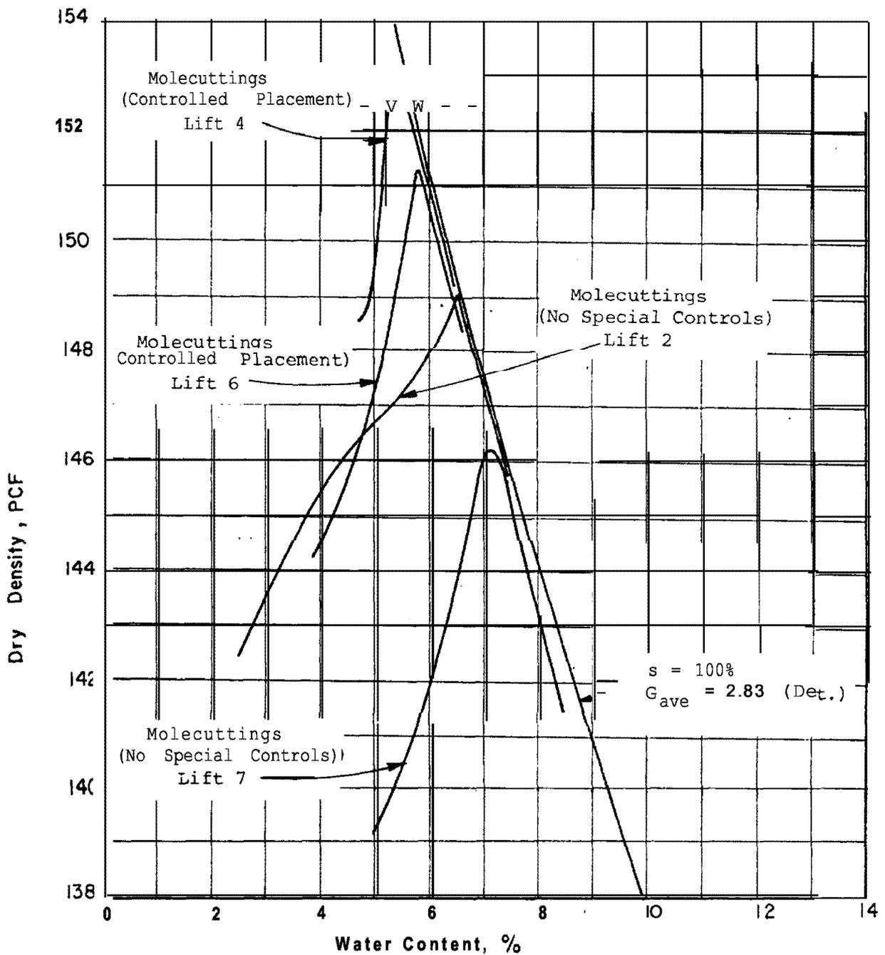
NOTE: 1. Compaction test performed in accordance with ASTM D1557, Method C, except the plus 1/2-in. material was discarded and no limitation placed on the percent retained on the 1/2-in. sieve.
