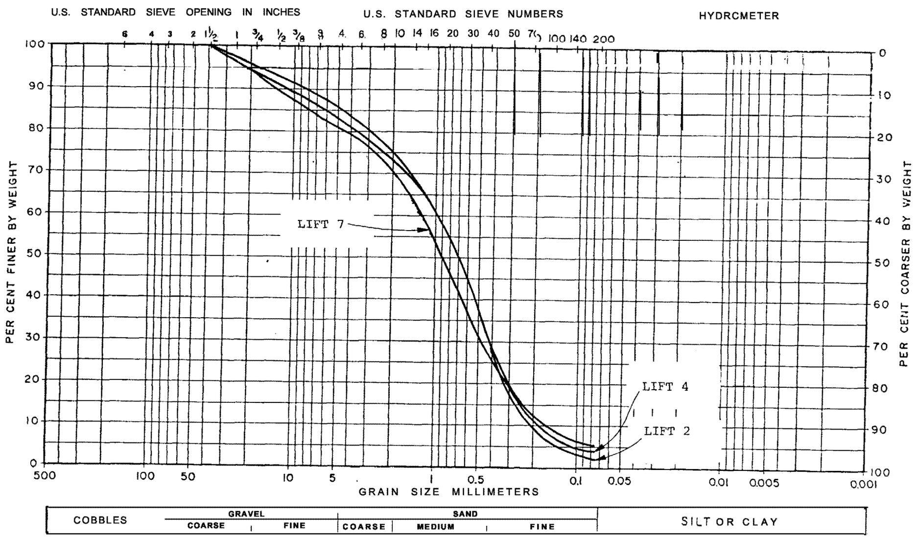
Grain-size analyses performed by Pittsburgh Testing Labs.
