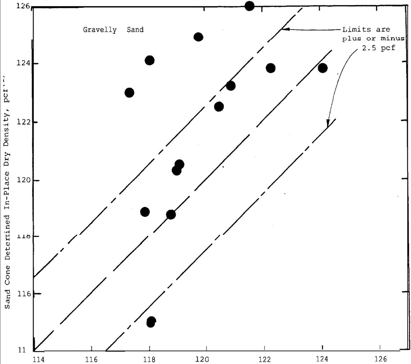
Nuclear Density Meter Determined In-Place Dry Density, pcf <sup>(2)</sup>
