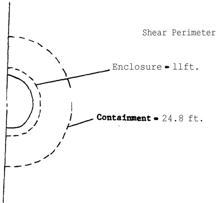
Figure 12 Impact Area and Shear Perimeter at 5 Feet From Nose
