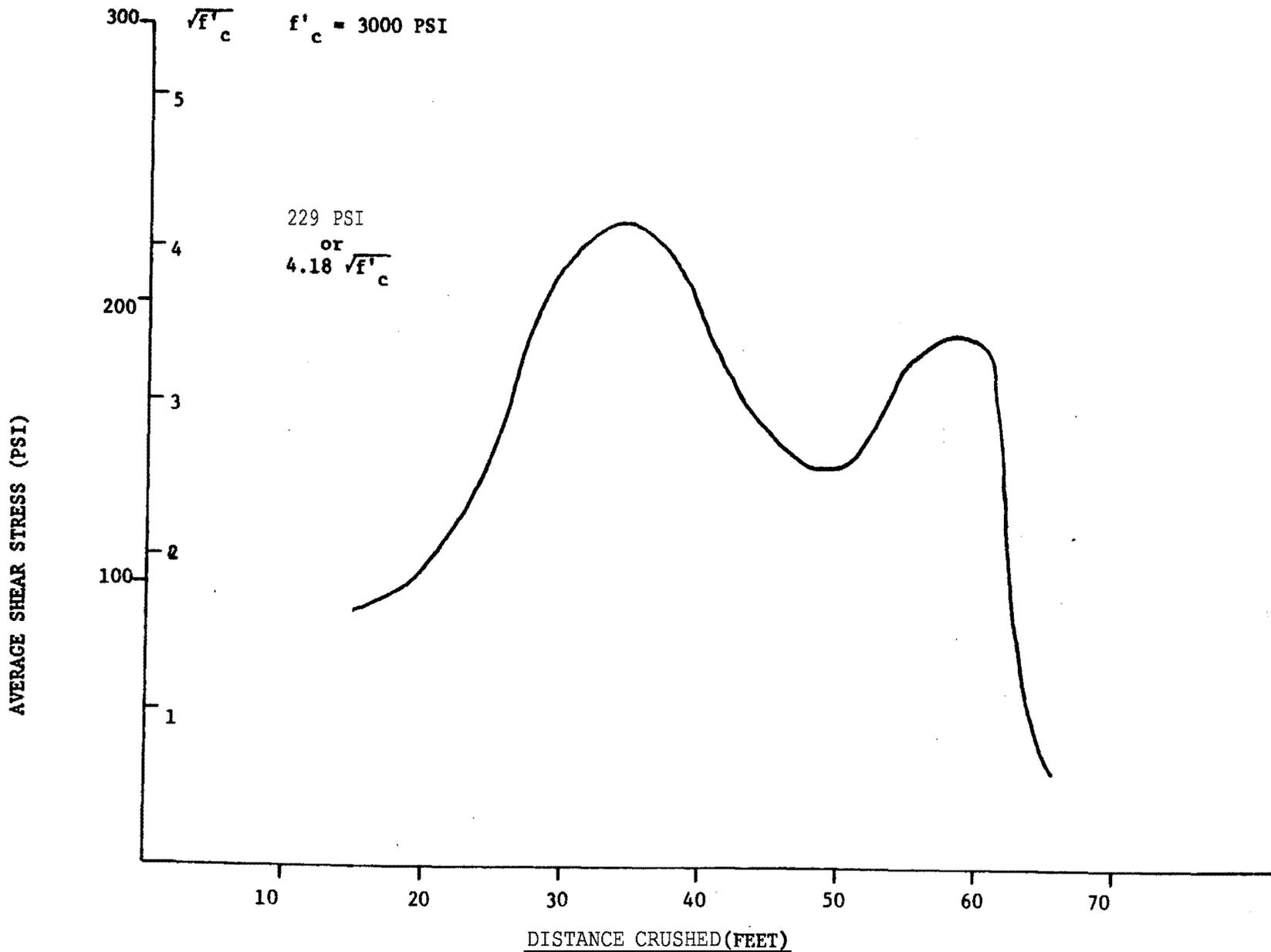
Figure 25 AVERAGE SHEAR STRESS-DISTANCE CRUSHED RELATIONSHIP FOR CONTAINMENT
