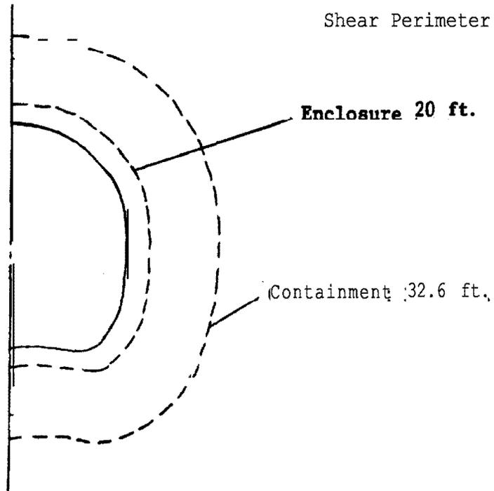
Figure 15 Impact Area and Shear Perimeter at 15 Feet From Nose
