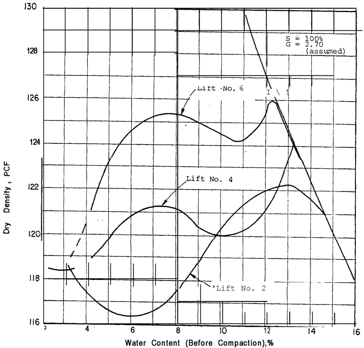
NOTE: Compaction test performed in accordance with ASTM D1557, Method D, by Pittsburgh Testing Labs.
