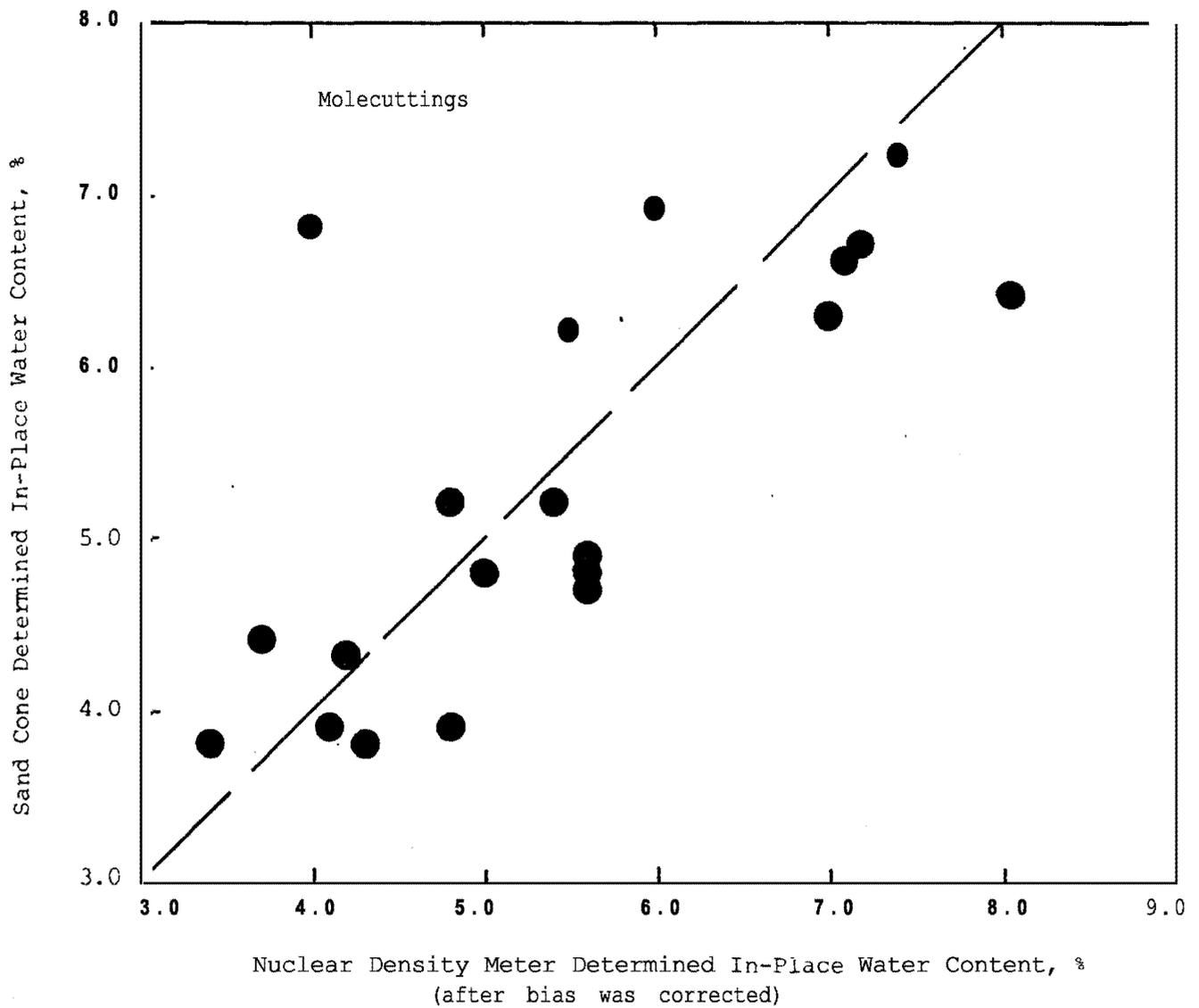
NOTES: 1. In-place water content is based on 8-in. deep nuclear test.
