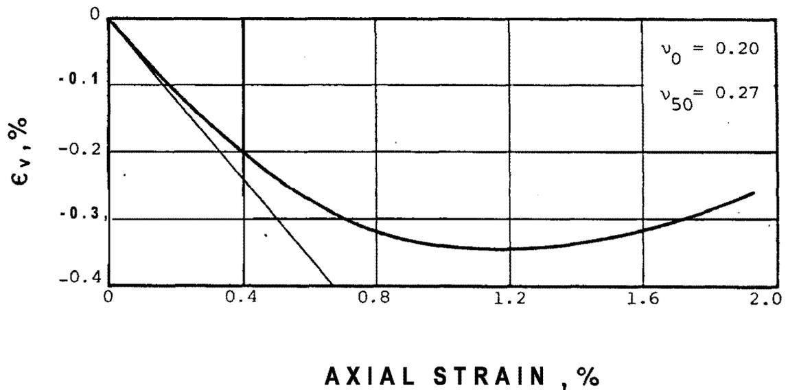
TEST S6 95% Compaction  $\bar{\sigma}_{3C} = 6.0 \text{ kg/cm}^2$
