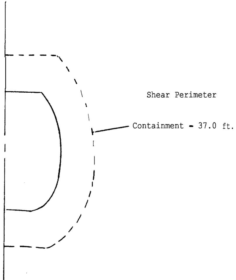
Figure 16, Impact Area and Shear Perimeter at 19.0 Feet From Nose
