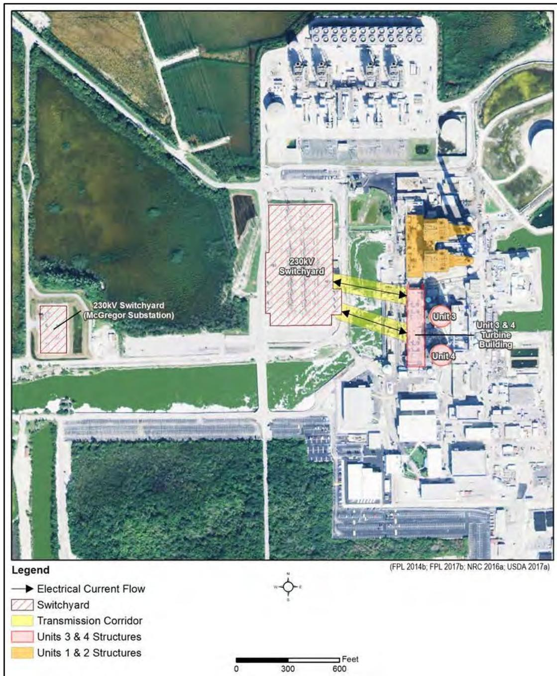
**Figure 3-6 Turkey Point In-Scope Transmission Lines (FPL 2018f)**
