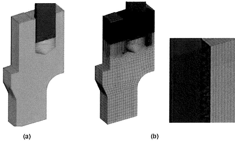
Figure 2: (a) Finite Element Model Showing Bolt and Flange Connection and,
