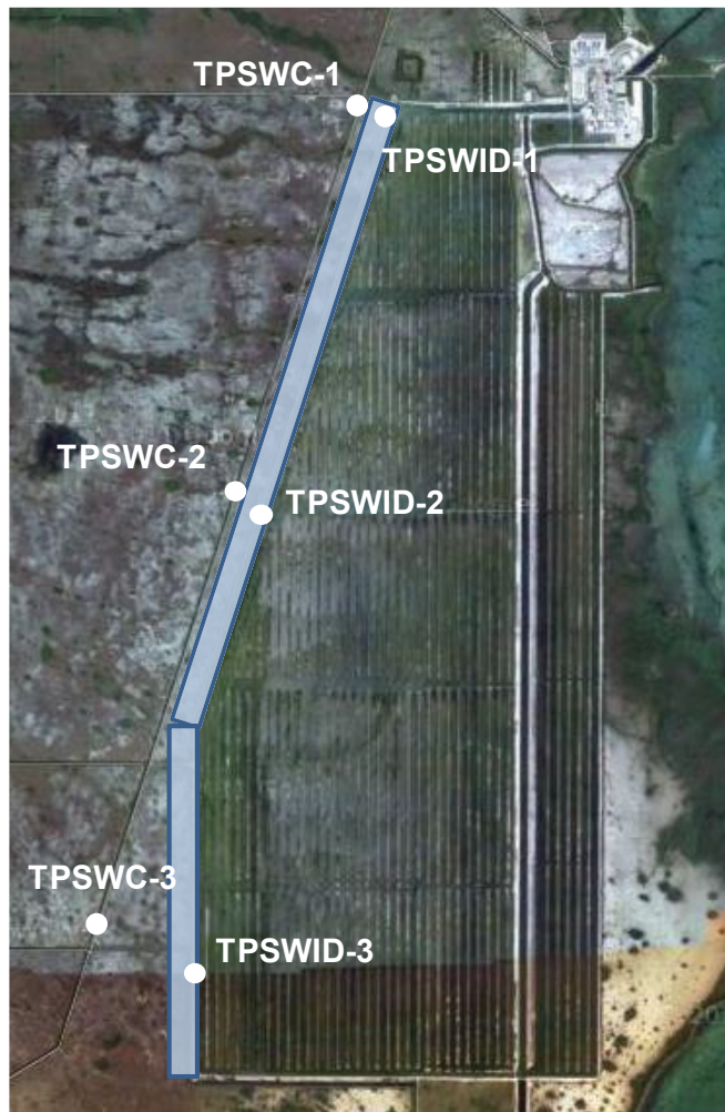
Figure 5.4-3. Locations of L-31E and ID Monitoring Stations; Conceptualized Seepage from L-31E into the ID is Shown.
