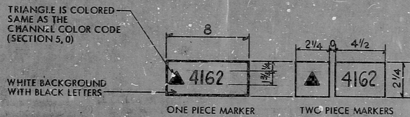
DETAIL B TYPICAL MARKERS FOR CABLE TRAY PLAN POINTS EXCEPT REACTOR BLDG - SEE NOTE 1, (THIS SHEET)
