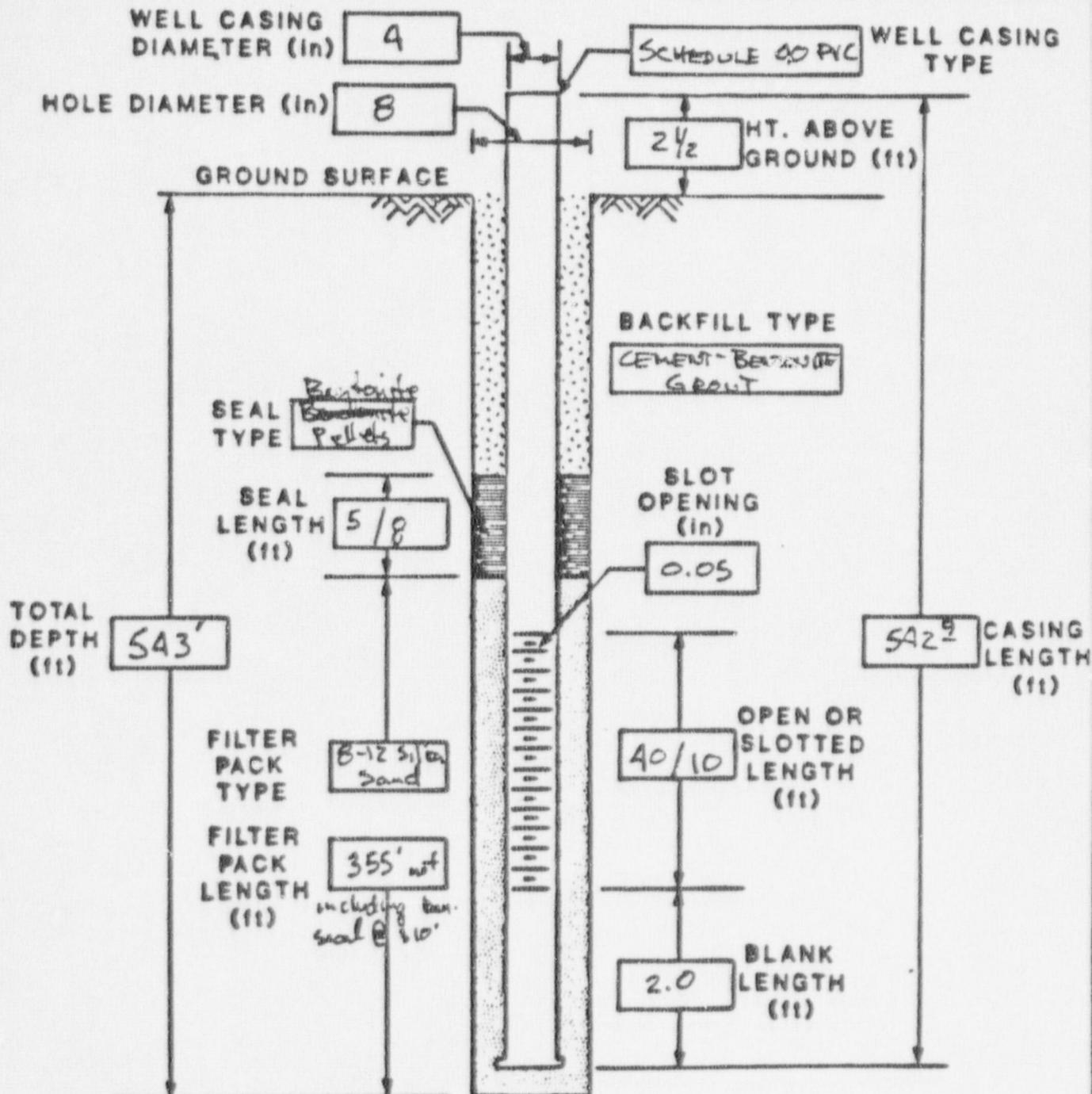
COMMENTS: Two screened intervals used at 541 to 501 and 280 to 220 feet depths, two seals used at 310 to 305 and 171 to 180'
