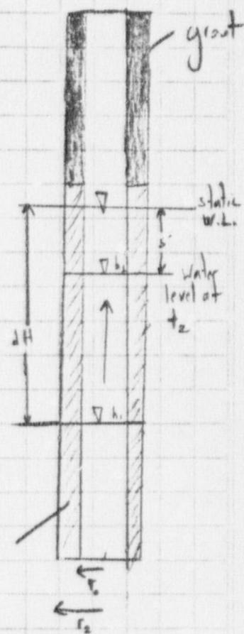
Of course if the static water level was located above the gravel pack, then the volume component in the gravel pack should not be included in the estimate of "V".
