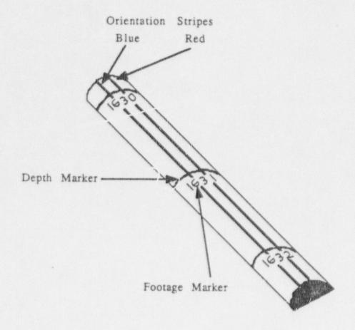
Figure 4. Example of Core Markings.
