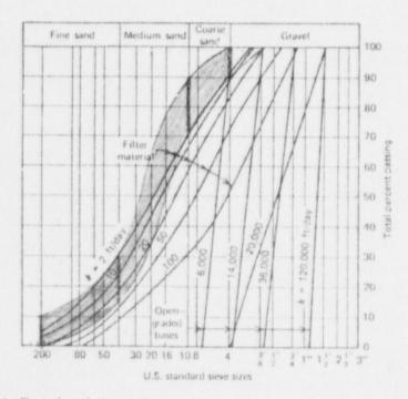
FIG. 6.9 Typical gradations and permeabilities of several open-graded aggregates and several filter materials. (FHWA Guidelines for the Design of Subsurface Drainage Systems for Highway Structural Sections, Figure No. 4).
