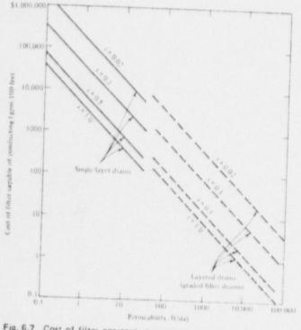
Fig. 6.7 Cost of filter aggregate per seepage unit (1 gpm conducted 100 ft). (After Cedergren and Lovering, Highway Research Record, No. 215, HRB, 1960, p. 3.)
