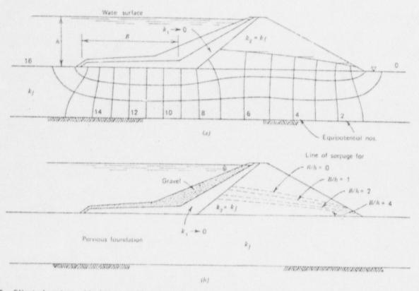
Fig. 15. Effect of upstream blanket on position of line of seepage. (a) Typical flow net (B/h = 2). (b) Position of line of seepage for various values of B/h.
