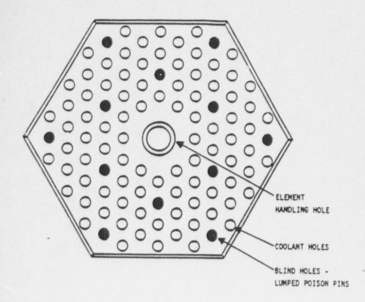
Figure 2-2 Defueling Element Top View (Dowels Not Shown)
