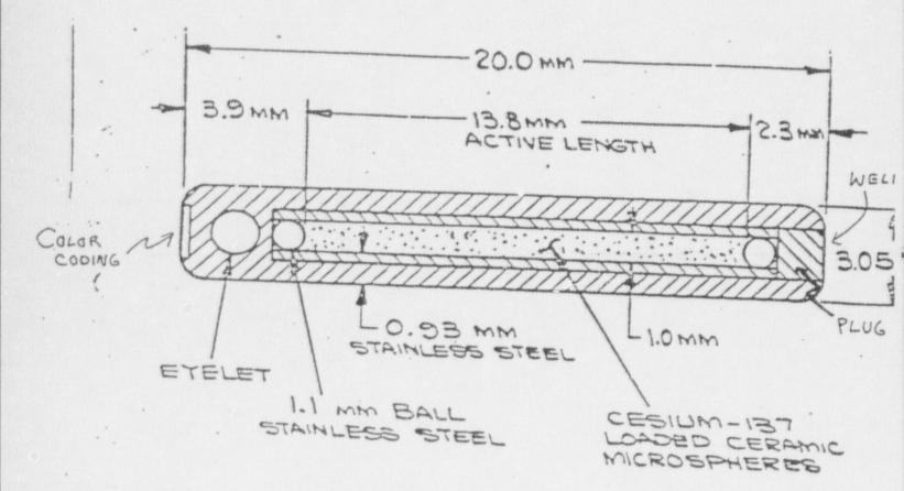
. Schematic Diagram of Modified 3M Cesium-137 Source. Series 6500
