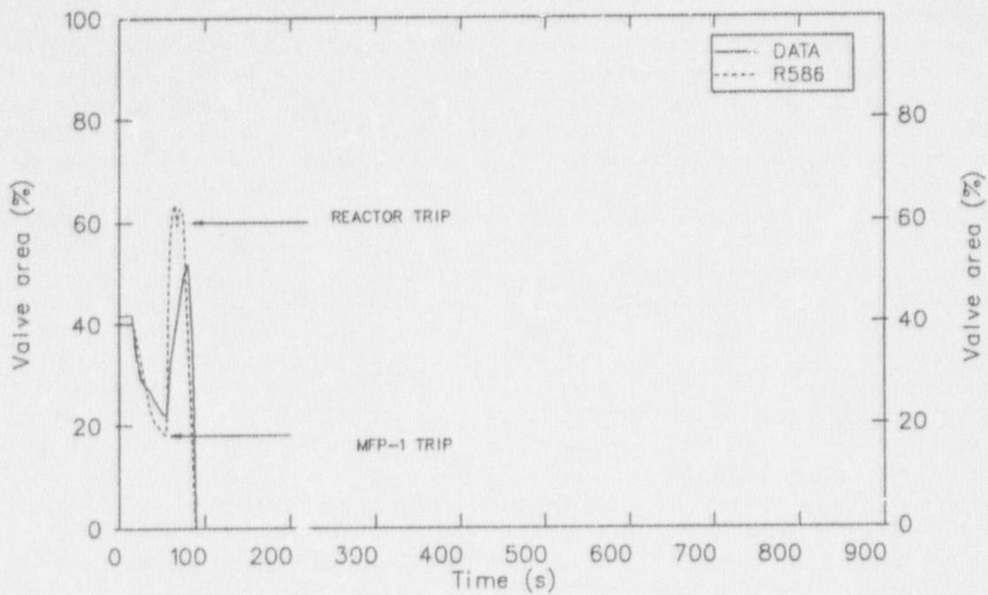
Figure 3. OTSG A main feedwater control valve area in the R586 calculation of the Davis-Besse LOFW transient.
