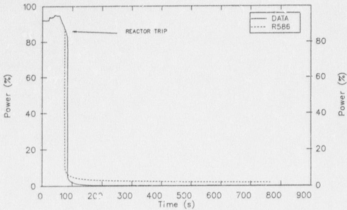
Figure 9. Reactor power in the R586 calculation of the Davis-Besse LOFW transient.
