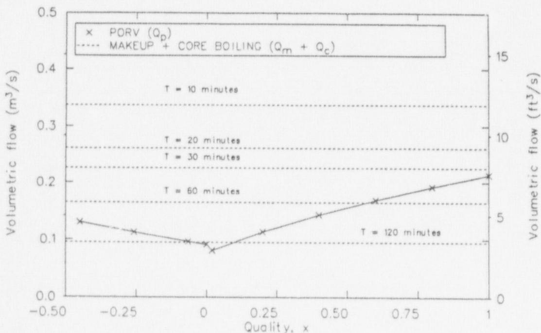
Figure 46. Results of the volume balance for different times after reactor trip.
