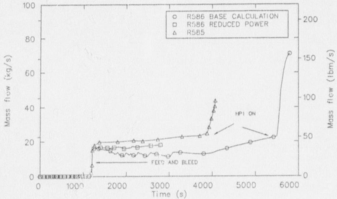
Figure 34. A comparison of calculated mass flows into the RCS during feed and bleed.
