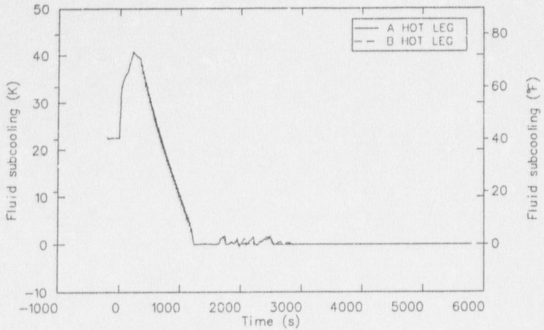
Figure 24. Hot leg subcooling in the R586 feed and bleed calculation.
