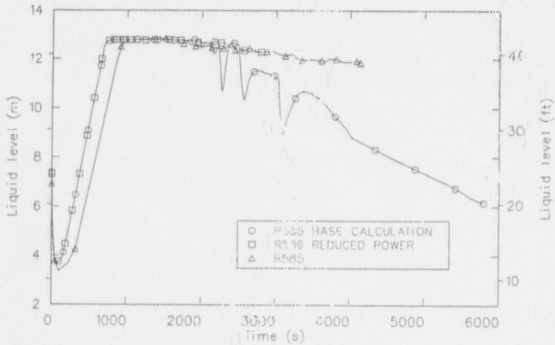
Figure 32. A comparison of calculated collapsed pressurizer liquid levels during feed and bleed.
