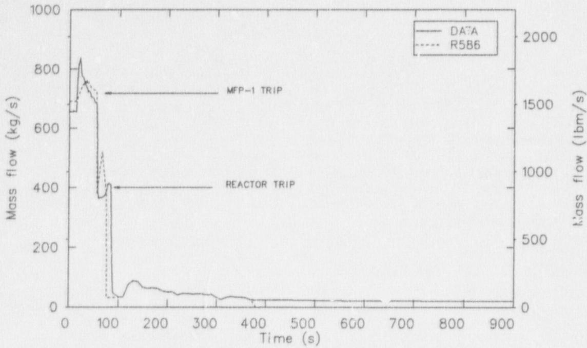
Figure 1. Feedwater flow to OTSG A in the R586 calculation of the Davis-Besse LOFW transient.
