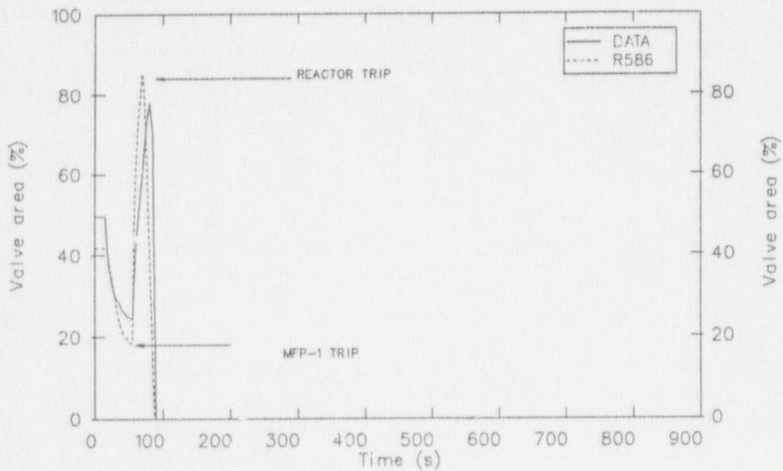
Figure 4. OTSG B main feedwater control valve area in the R586 calculation of the Davis-Besse LOFW transient.
