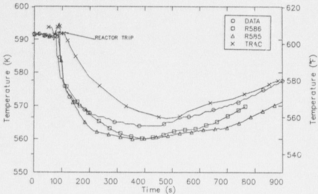
Figure 17. A comparison of calculated coolant temperatures in the B loop hot leg during the Davis-Besse LOFW transient.
