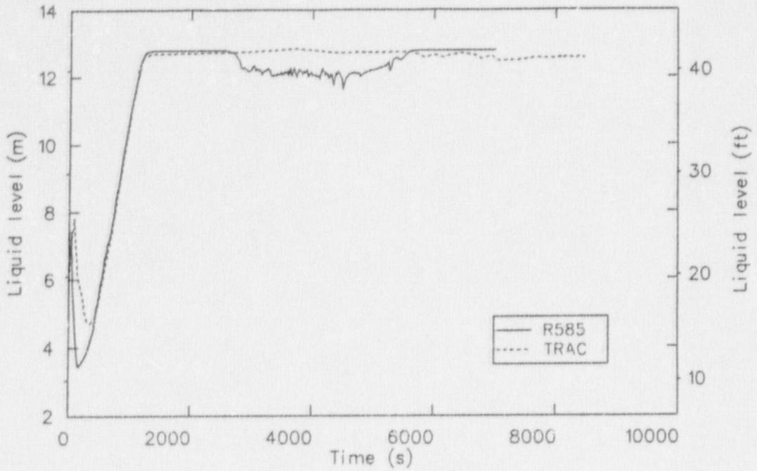
Figure 39. A comparison of calculated collapsed liquid levels in the pressurizer when feed and bleed was initiated near 2200 s.
