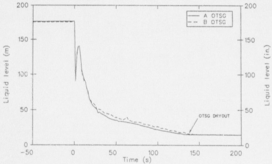
Figure 20. OTSG startup liquid levels in the R586 feed and bleed calculation.
