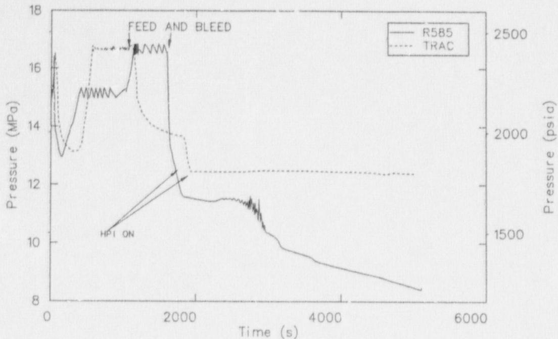
Figure 41. A comparison of calculated reactor coolant pressures when feed and bleed was initiated near 1500 s.
