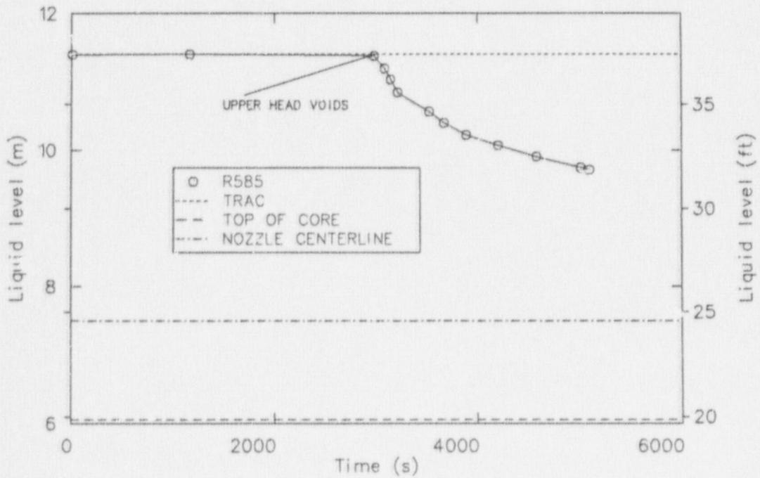
Figure 45. A comparison of calculated collapsed liquid levels in the reactor vessel when feed and bleed was initiated near 1500 s.
