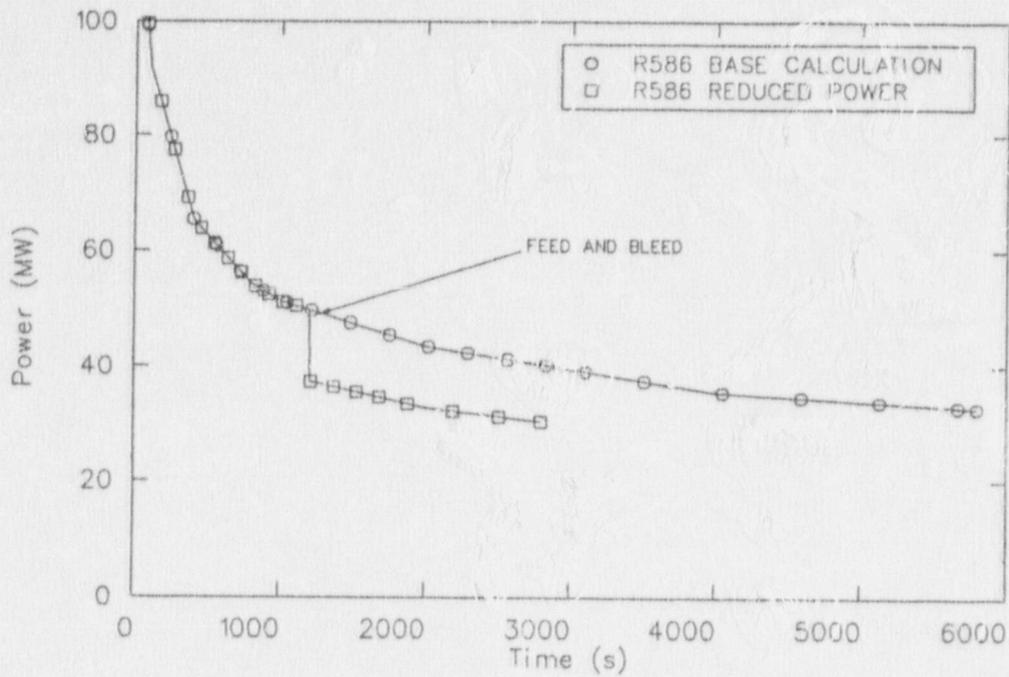
Figure 31. A comparison of core power from the R586 base and sensitivity feed and bleed calculations.
