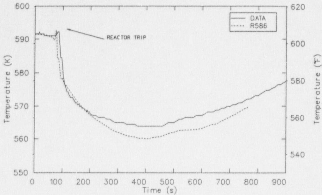
Figure 11. Coolant temperatures in the B loop hot leg in the R586 calculation of the Davis-Besse LOFW transient.
