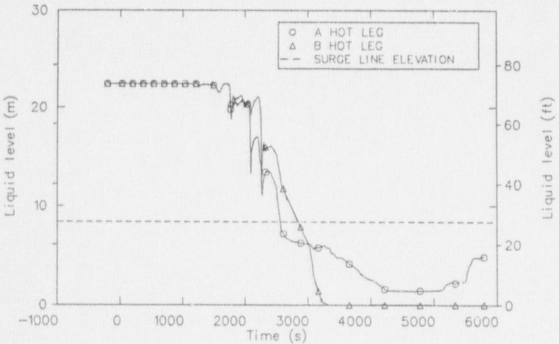
Figure 27. Hot leg collapsed liquid levels in the R586 feed and bleed calculation.
