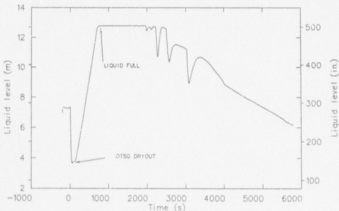
Figure 23. Pressurizer liquid level in the R586 feed and bleed calculation.
