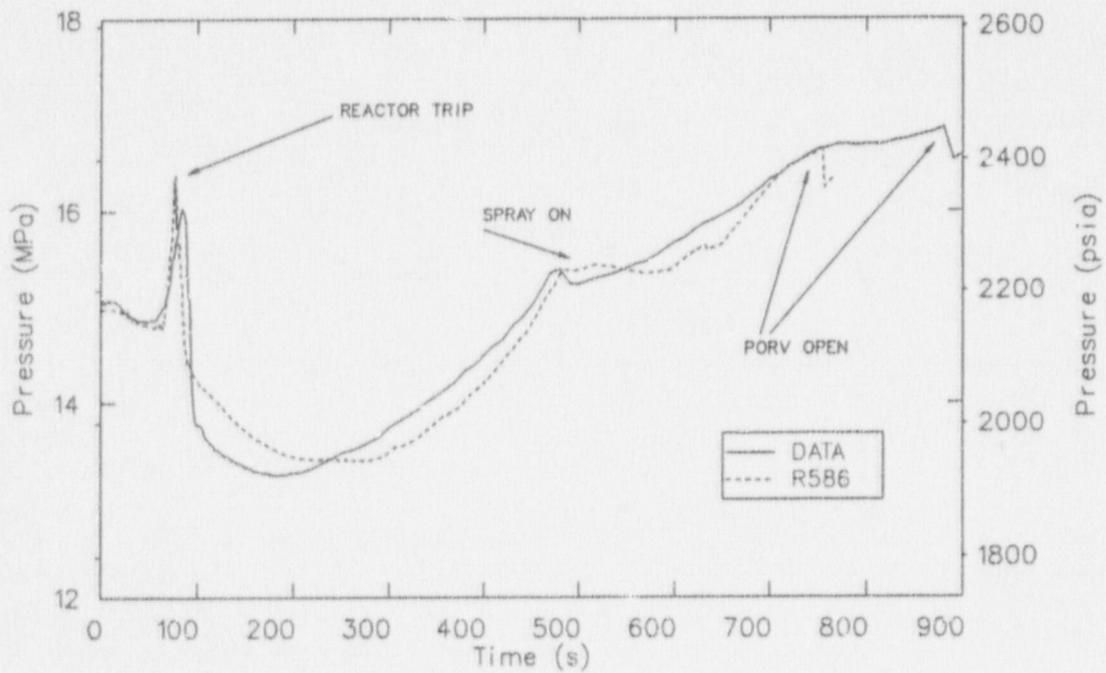
Figure 10. Reactor coolant pressure in the R586 calculation of the Davis-Besse LOFW transient.
