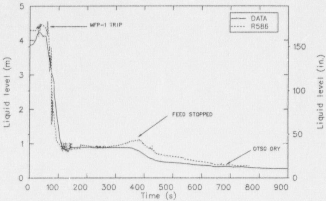
Figure 6. Startup liquid level in OTSG B in the R586 calculation of the Davis-Besse LOFW transient.
