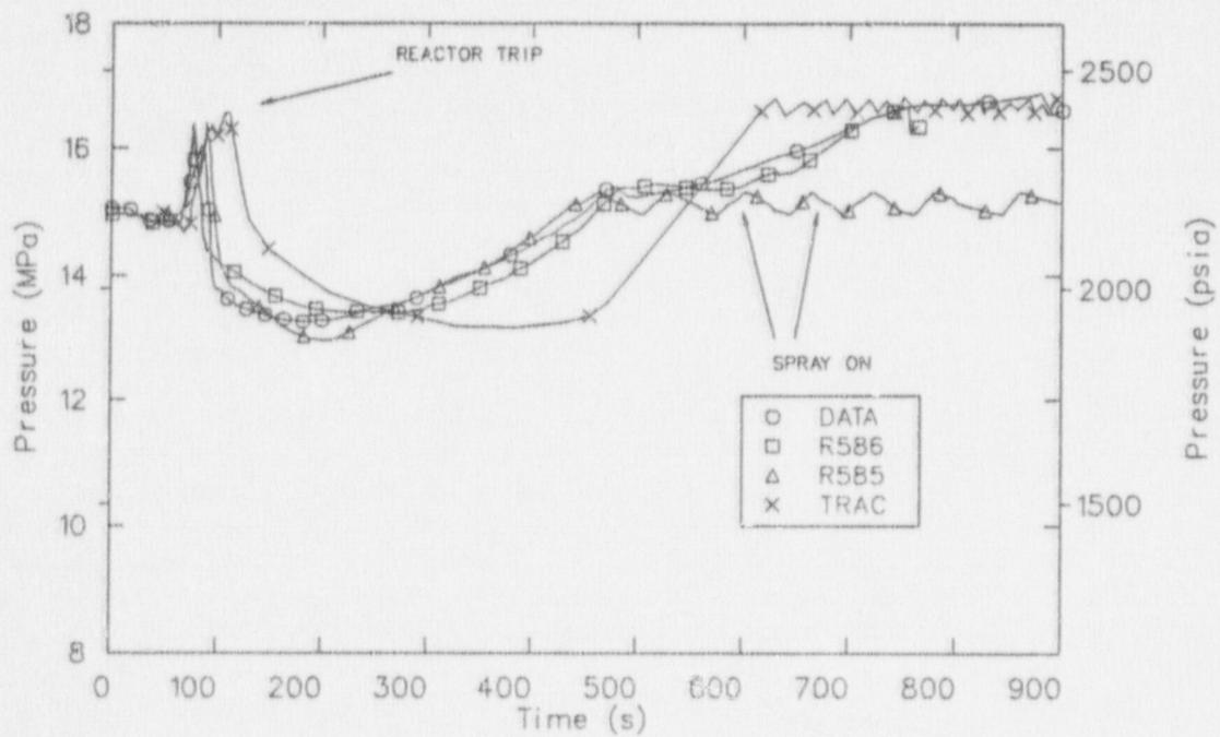
Figure 15. A comparison of calculated reactor coolant pressures during the Davis-Besse LOFW transient.
