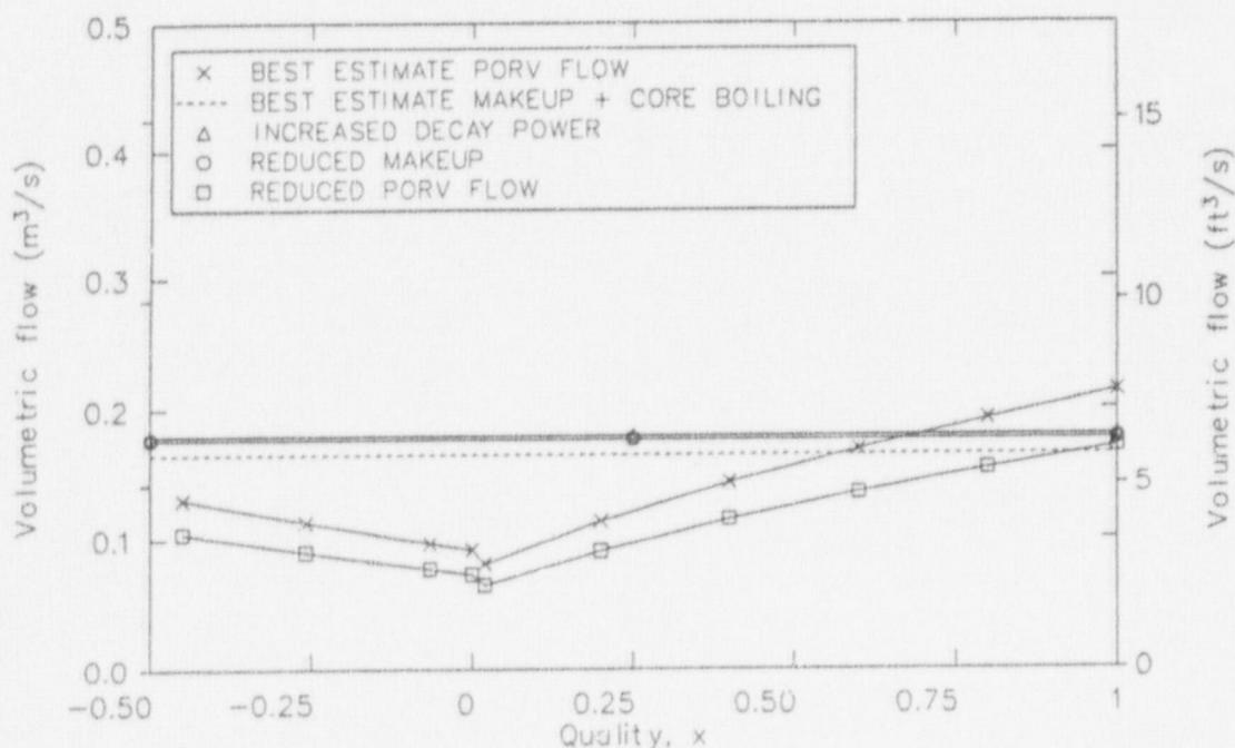
Figure 47. The effect of uncertainty in boundary conditions on the results of the volume balance.
