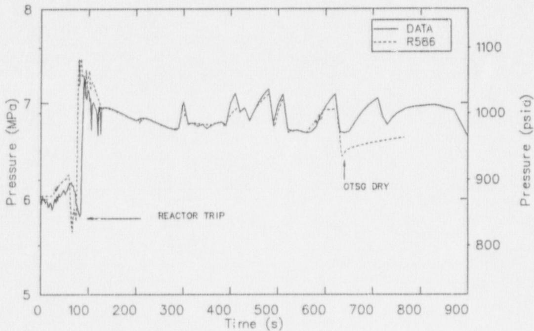
Figure 7. Pressure in OTSG A in the R586 calculation of the Davis-Besse LOFW transient.
