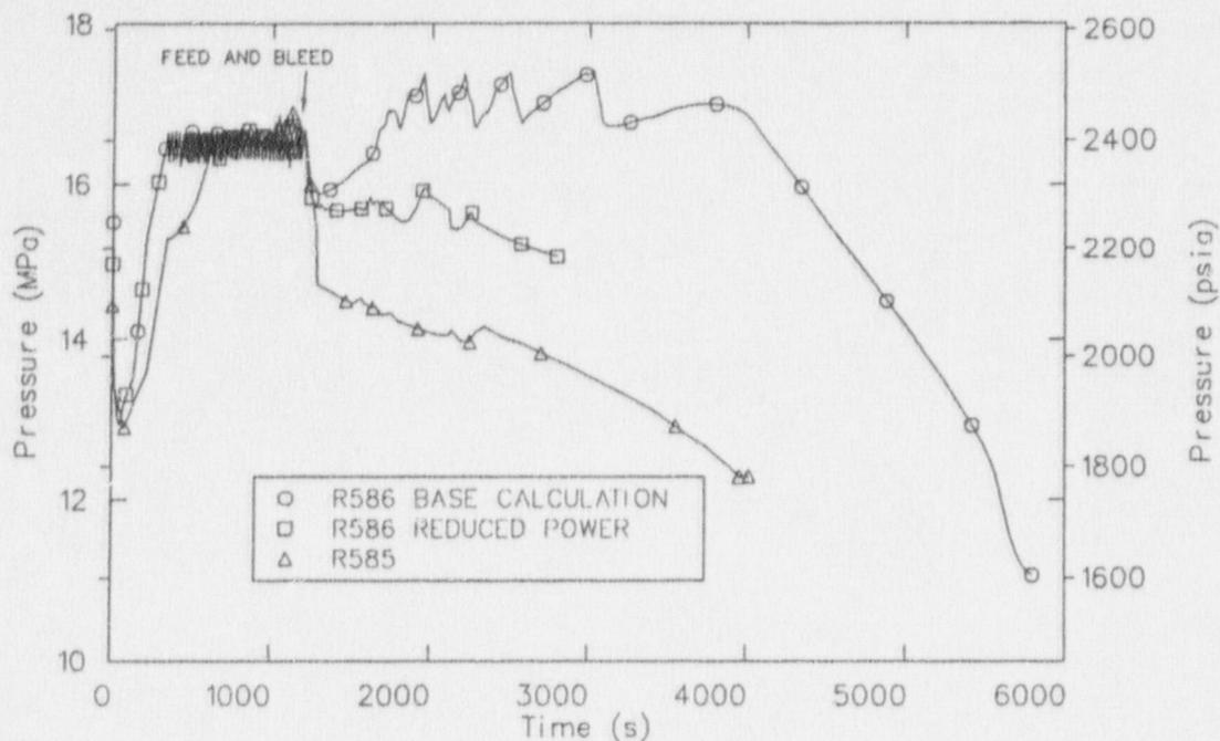
Figure 30. A comparison of calculated reactor coolant pressures during feed and bleed.
