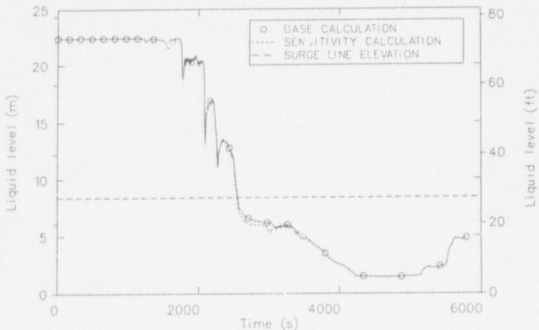
Figure C-1. The effect of hot leg nodalization on collapsed liquid level in the A loop hot leg.
