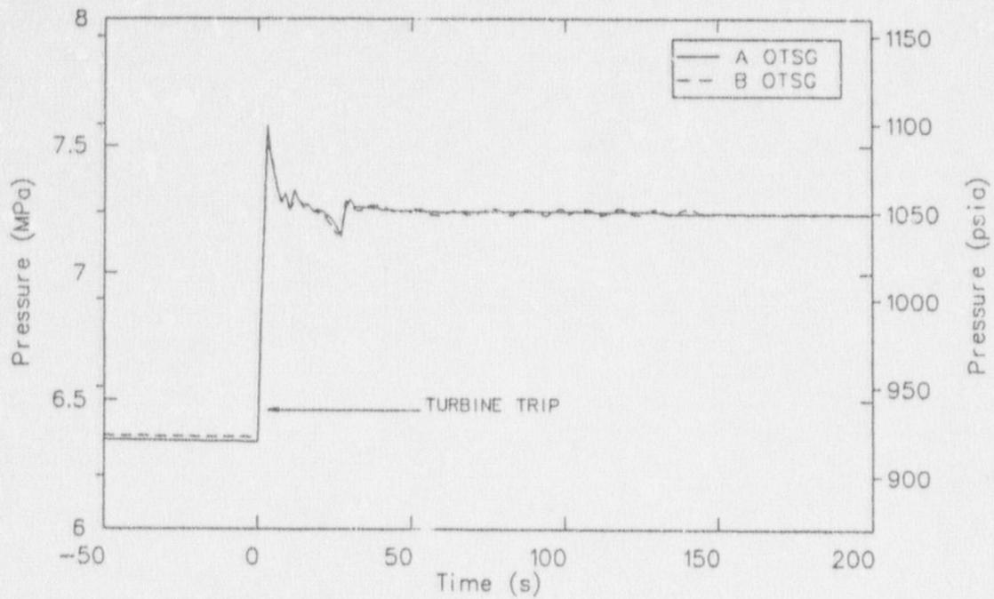
Figure 19. OTSG pressures in the R586 feed and bleed calculation.
