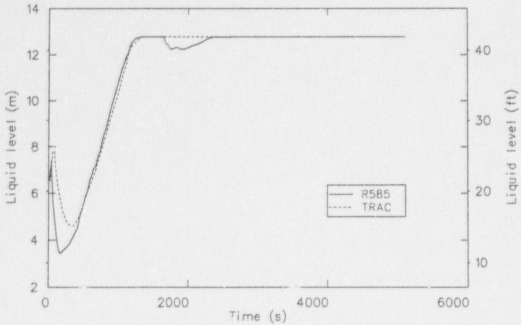
Figure 44. A comparison of calculated collapsed liquid levels in the pressurizer when feed and bleed was initiated near 1500 s.
