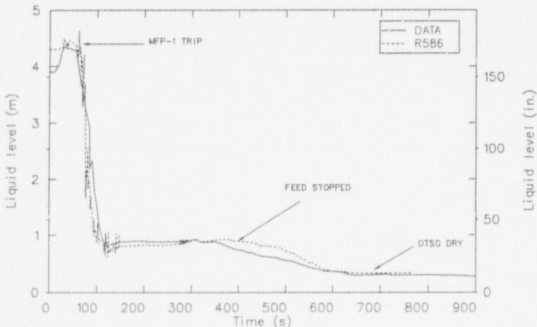
Figure 5. Startup liquid level in OTSG A in the R586 calculation of the Davis-Besse LOFW transient.
