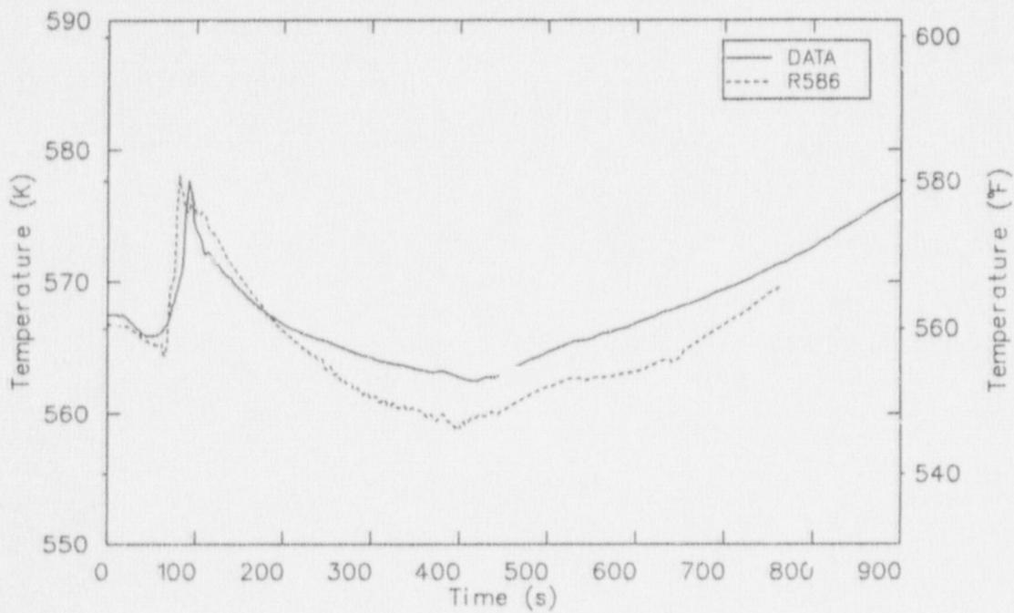
Figure 12. Coolant temperatures in the B loop cold leg in the R586 calculation of the Davis-Besse LOFW transient.
