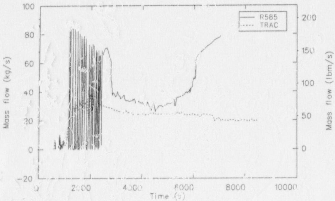
Figure 37. A comparison of calculated mass flow rate of the RCS when feed and bleed was initiated near 2200 s.
