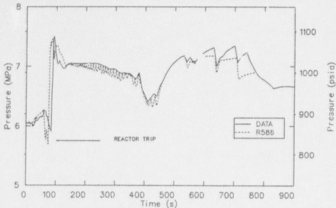
Figure 8. Pressure in OTSG B in the R586 calculation of the Davis-Besse LOFW transient.
