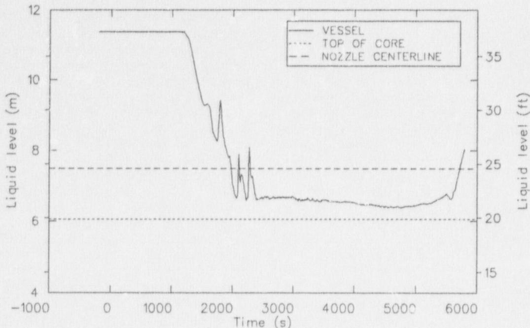
Figure 29. Collapsed liquid level in the reactor vessel during the R586 feed and bleed calculation.
