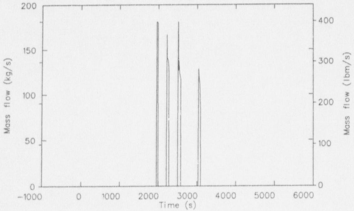
Figure 25. Mass flow through the pressurizer SRVs in the R586 feed and bleed calculation.
