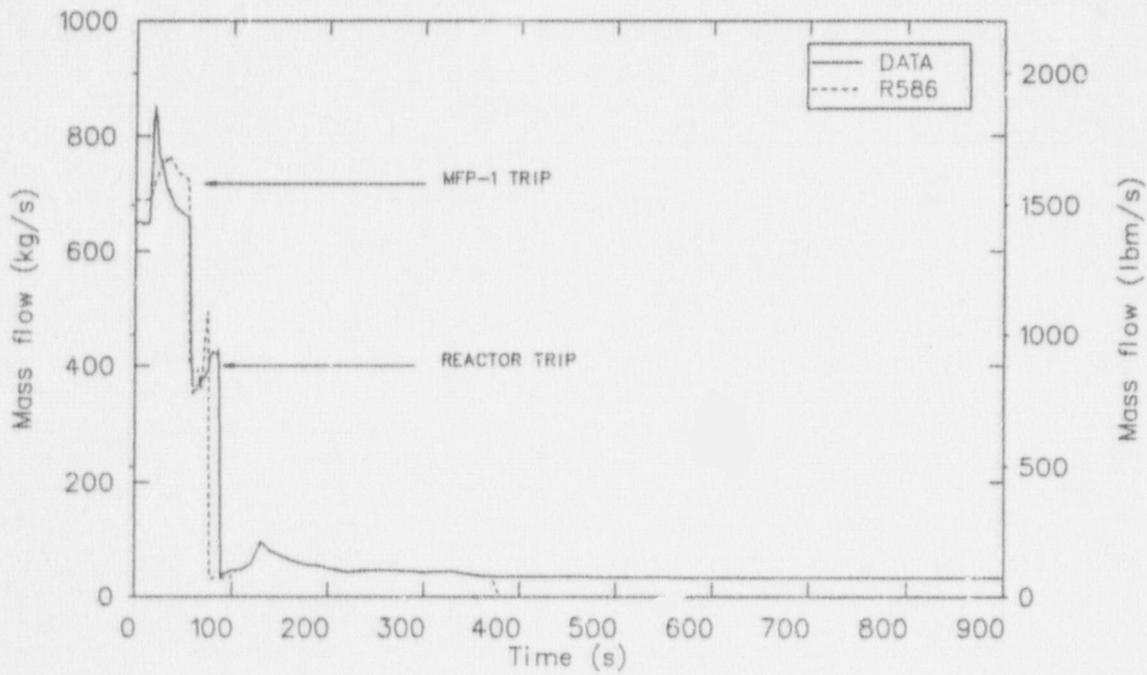
Figure 2. Feedwater flow to OTSG B in the R586 calculation of the Davis-Besse LOFW transient.
