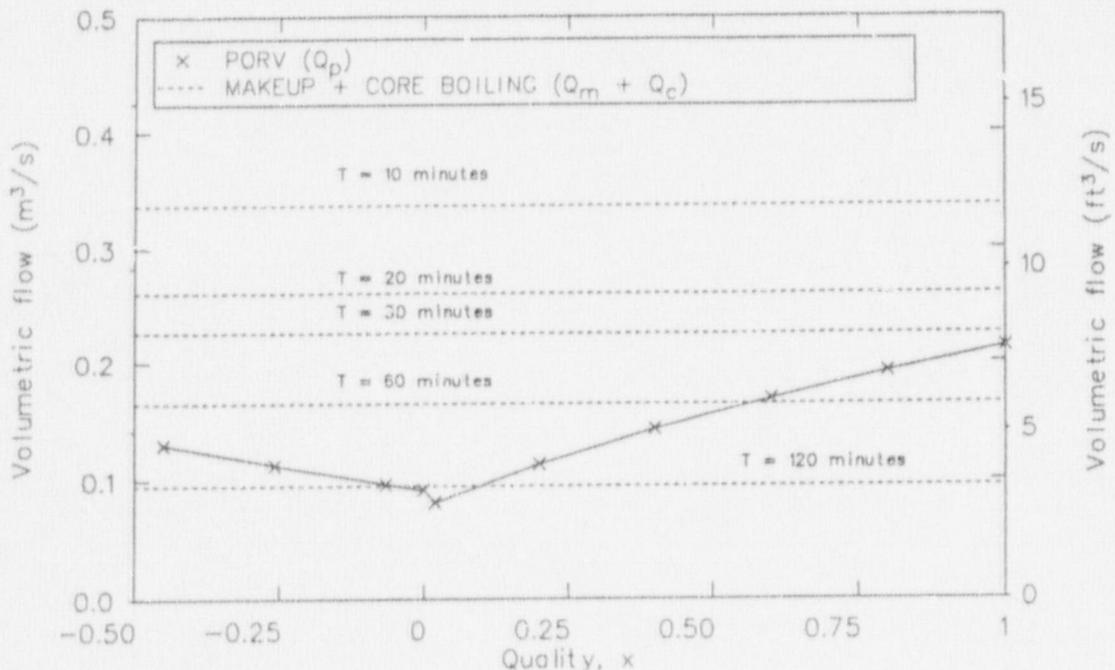
Figure C-3. Results of the volume balance for different times after reactor trip.
