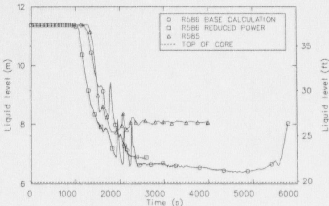
Figure 35. A comparison of calculated collapsed liquid levels in the reactor vessel during feed and bleed.
