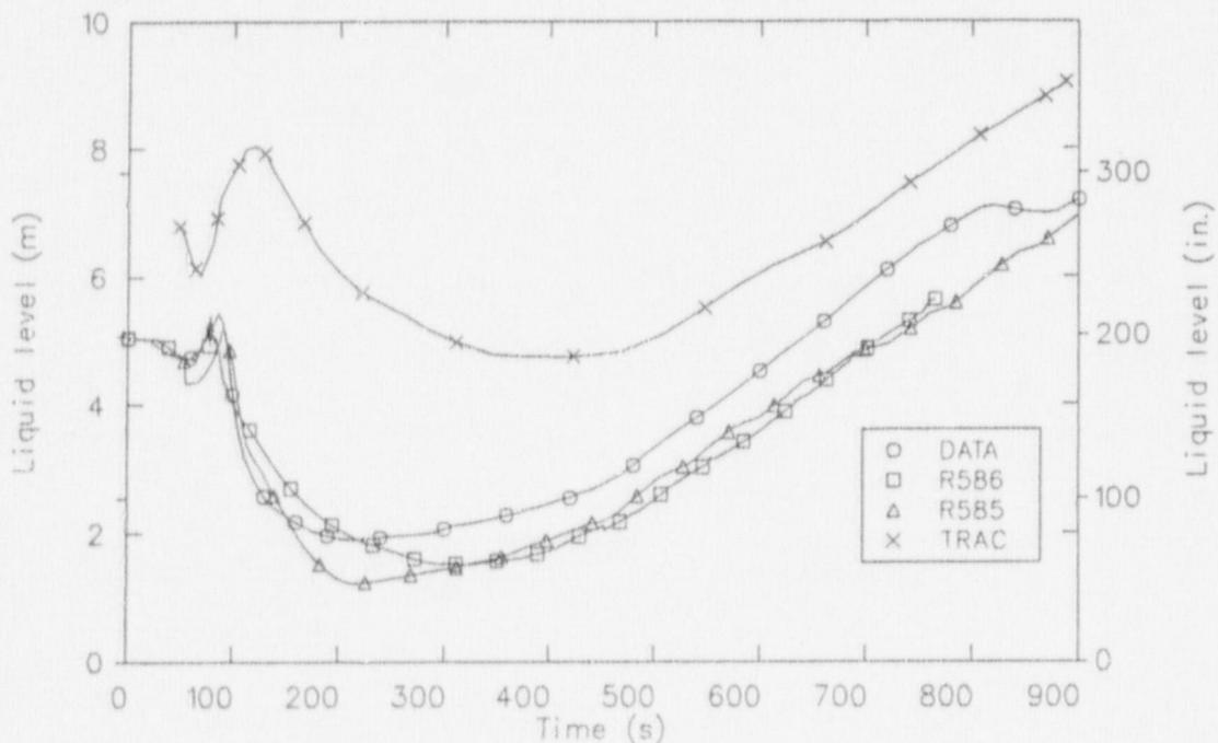
Figure 16. A comparison of calculated pressurizer liquid levels during the Davis-Besse LOFW transient.
