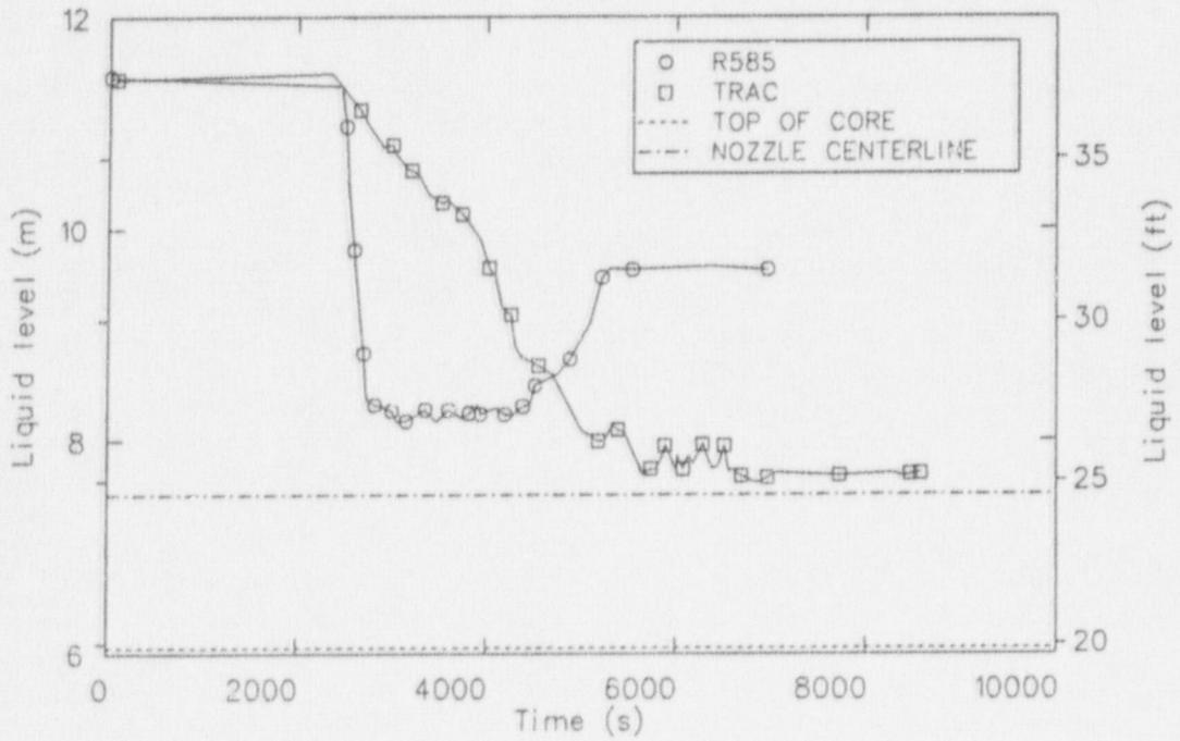
Figure 40. A comparison of calculated collapsed liquid levels in the reactor vessel when feed and bleed was initiated near 2200 s.
