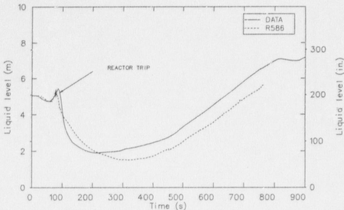
Figure 13. Pressurizer liquid levels in the R586 calculation of the Davis-Besse LOFW transient.
