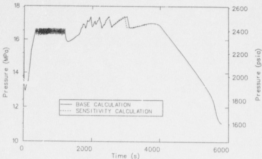
Figure C-2. The effect of hot leg nodalization on RCS pressure.
