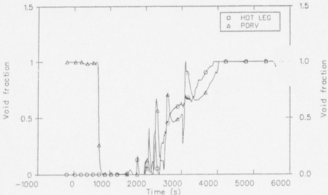
Figure 28. Hot leg and PORV void fractions in the R586 feed and bleed calculation.
