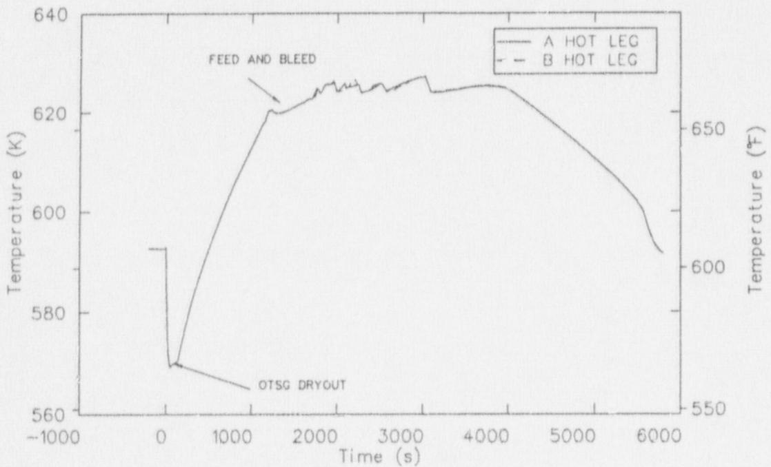
Figure 22. Hot leg coolant temperatures in the R586 feed and bleed calculation.
