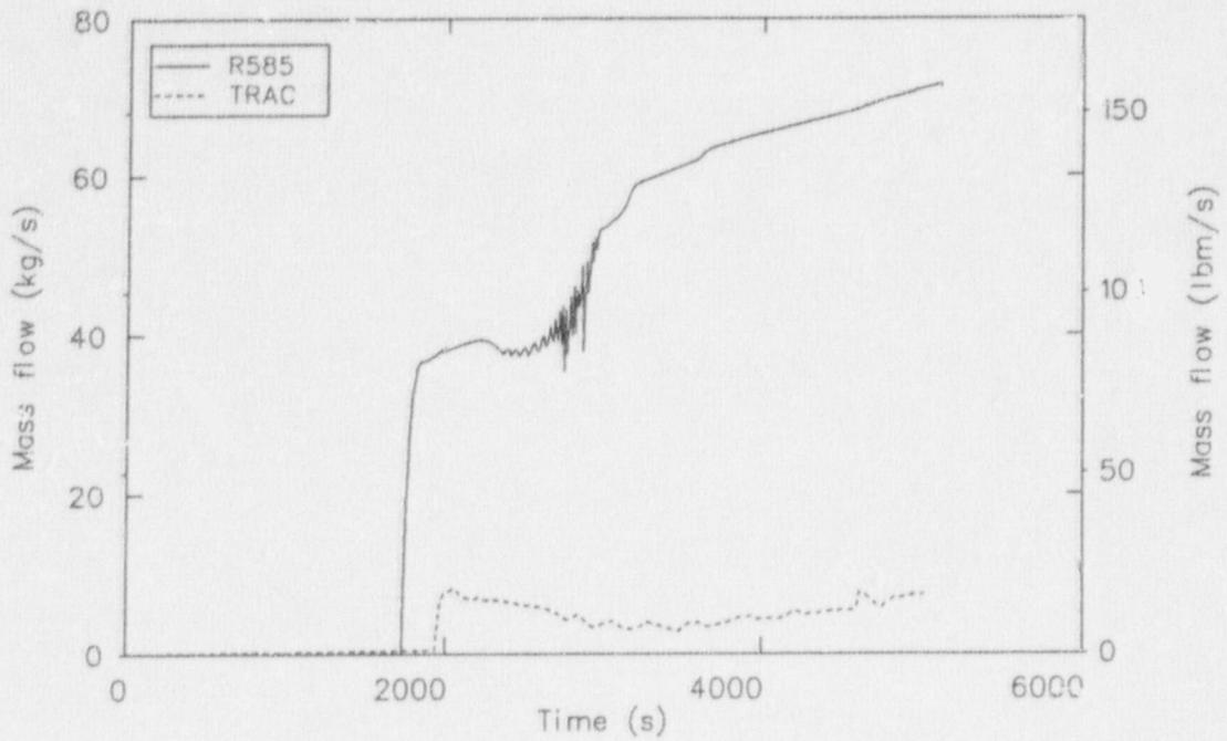
Figure 42. A comparison of calculated HPI flow rates when feed and bleed was initiated near 1500 s.
