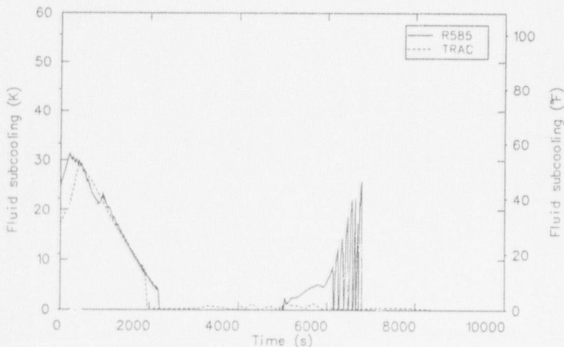
Figure 38. A comparison of calculated subcooling in the A loop hot leg when feed and bleed was initiated near 2200 s.
