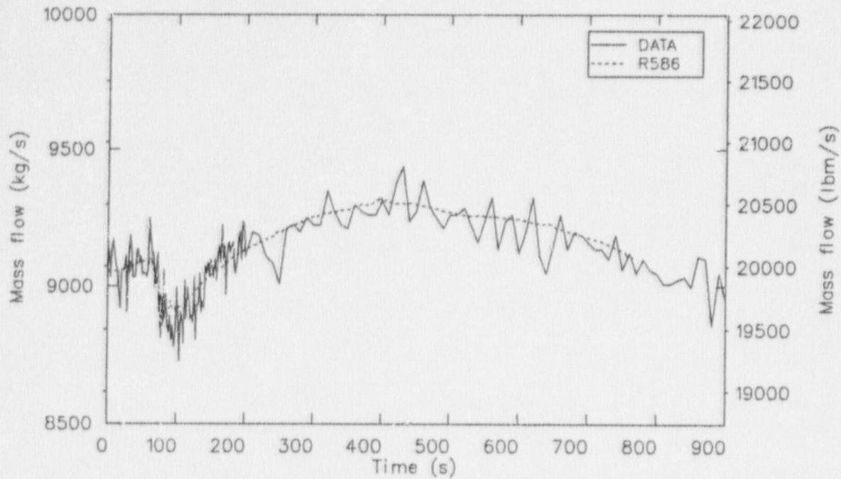
Figure 14. Mass flow in the A loop hot leg in the R586 calculation of the Davis-Besse LOFW transient.
