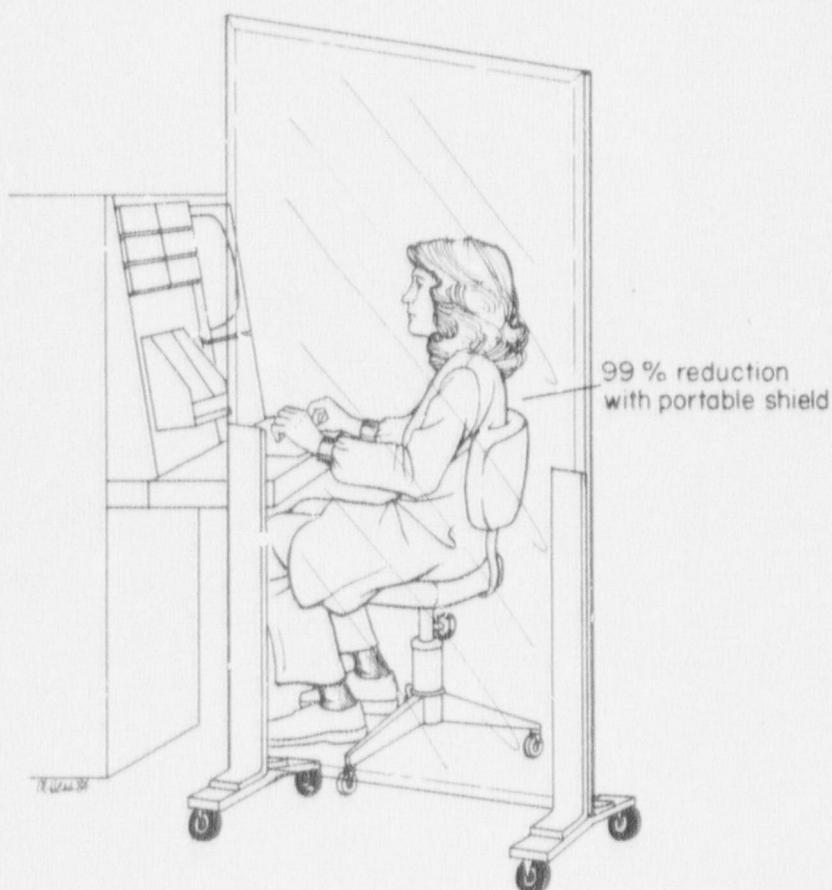
Reduction of personnel radiation exposure due to use of portable lead shield.
