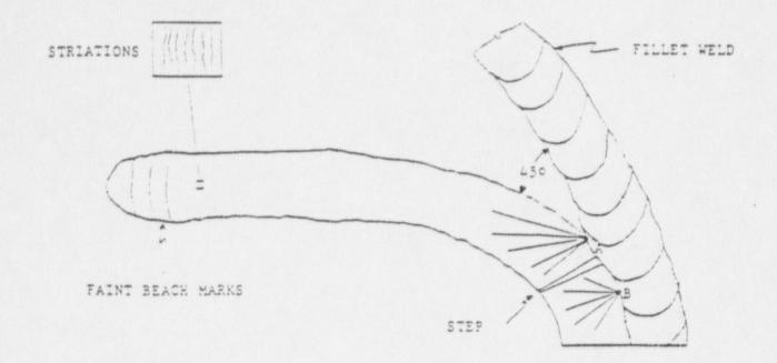
Figure No. 3 A Schematic of the Fracture Surface Highlighting Discernible Features from the Examination
