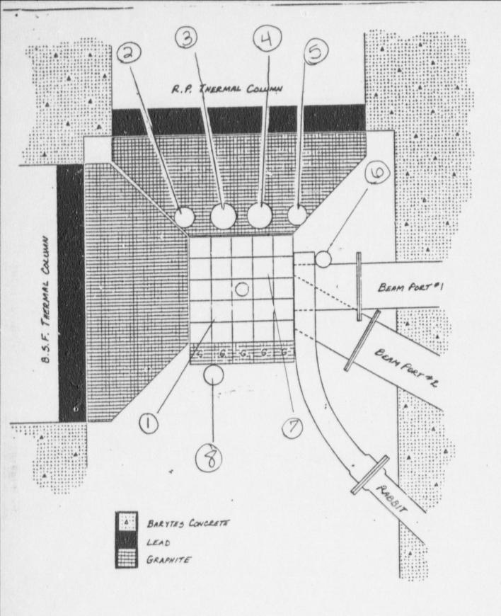
FIGURE 1. OSU Reactor Core Layout - Top View
