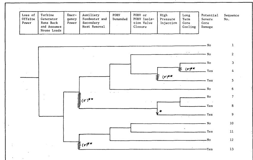
NSIC 103111 — Sequence of Interest for Condenser Circulating Water Valves Failure to Close at Oconee 3 \*not included in mitigation procedures.
