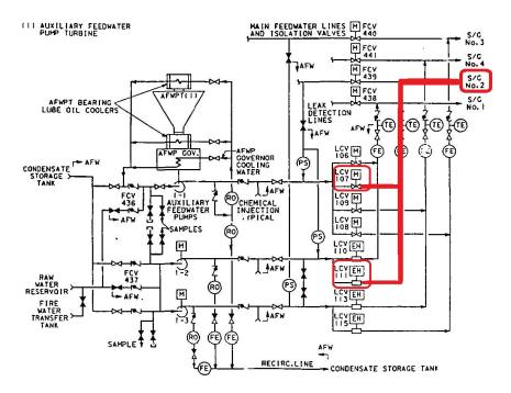
The red lines show the piping downstream of LCVs 107 and 111 that supply flow to Unit 1 Steam Generator No. 2.
