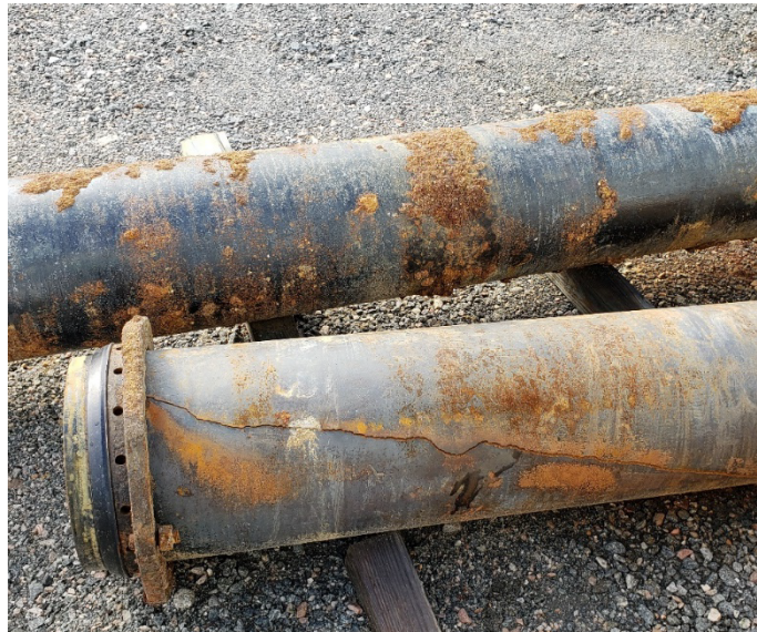
July 2019 Surry Power Station Fire Main Yard Loop Piping Rupture (ADAMS Accession No. ML20056D677)
