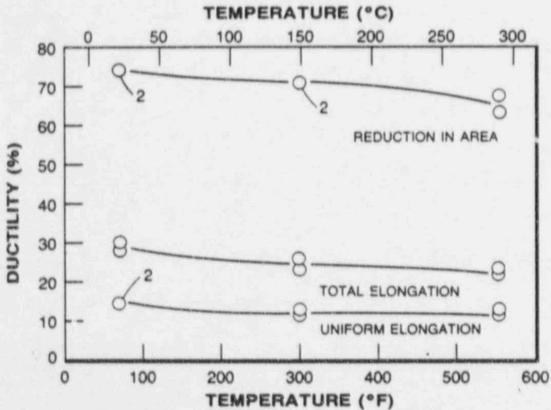
FIGURE 3-7. PREIRRADIATION TENSILE PROPERTIES FOR THE CATAWBA UNIT NO. 2 REACTOR PRESSURE VESSEL CORE REGION WELD METAL
