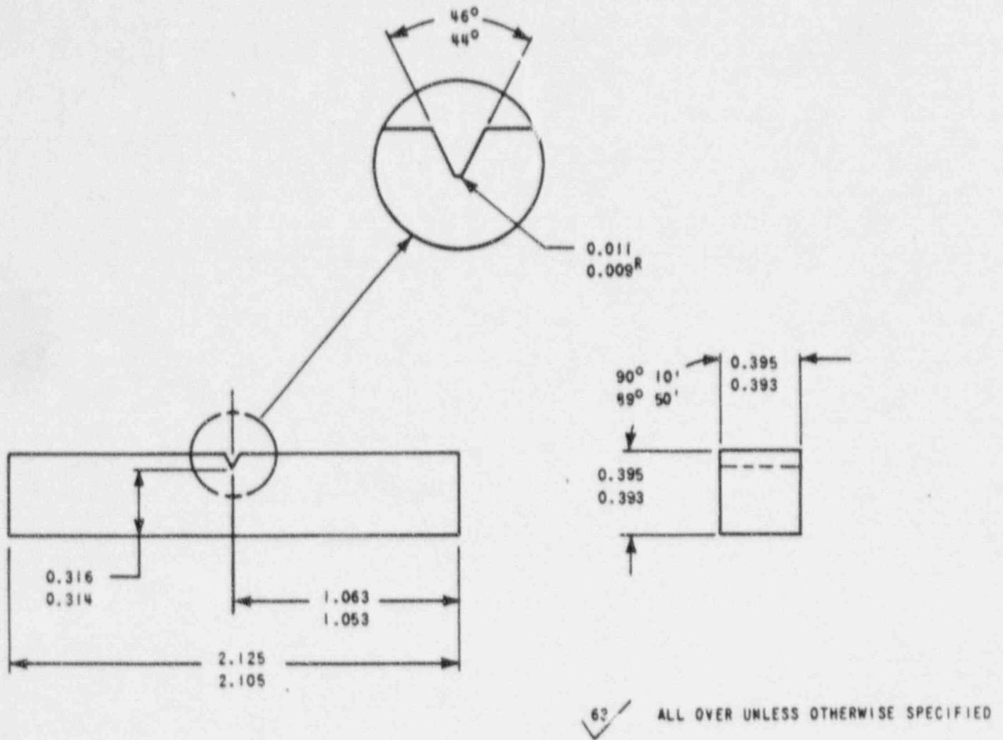
Figure 2-1. Charpy V-notch Impact Specimen
