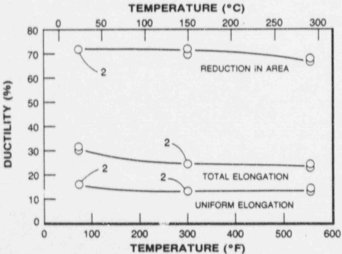
FIGURE 3-5. PREIRRADIATION TENSILE PROPERTIES FOR THE CATAWBA UNIT NO. 2 REACTOR PRESSURE VESSEL INTERMEDIATE SHELL PLATE B8605-1 (LONGITUDINAL ORIENTATION)
