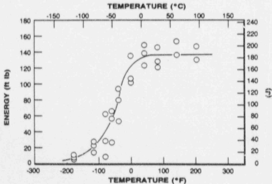
FIGURE 3-4. PREIRRADIATION CHARPY V-NOTCH IMPACT ENERGY FOR THE CATAWBA UNIT NO. 2 REACTOR PRESSURE VESSEL WELD HEAT-AFFECTED-ZONE MATERIAL
