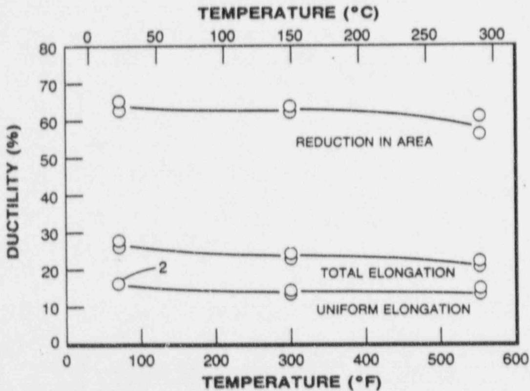
FIGURE 3-6. PREIRRADIATION TENSILE PROPERTIES FOR THE CATAWBA UNIT NO. 2 REACTOR PRESSURE VESSEL INTERMEDIATE SHELL PLATE B8605-1 (TRANSVERSE ORIENTATION)
