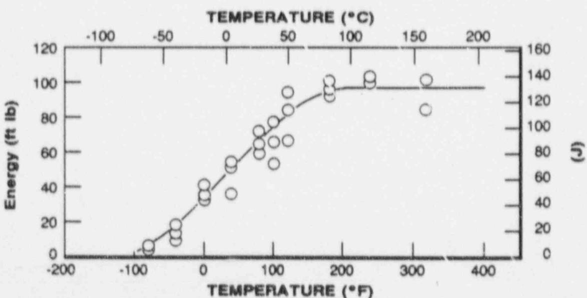
FIGURE 3-2. PREIRRADIATION CHARPY V-NOTCH IMPACT ENERGY FOR THE CATAWBA UNIT NO. 2 REACTOR PRESSURE VESSEL INTERMEDIATE SHELL PLATE B8605-1 (TRANSVERSE ORIENTATION)
