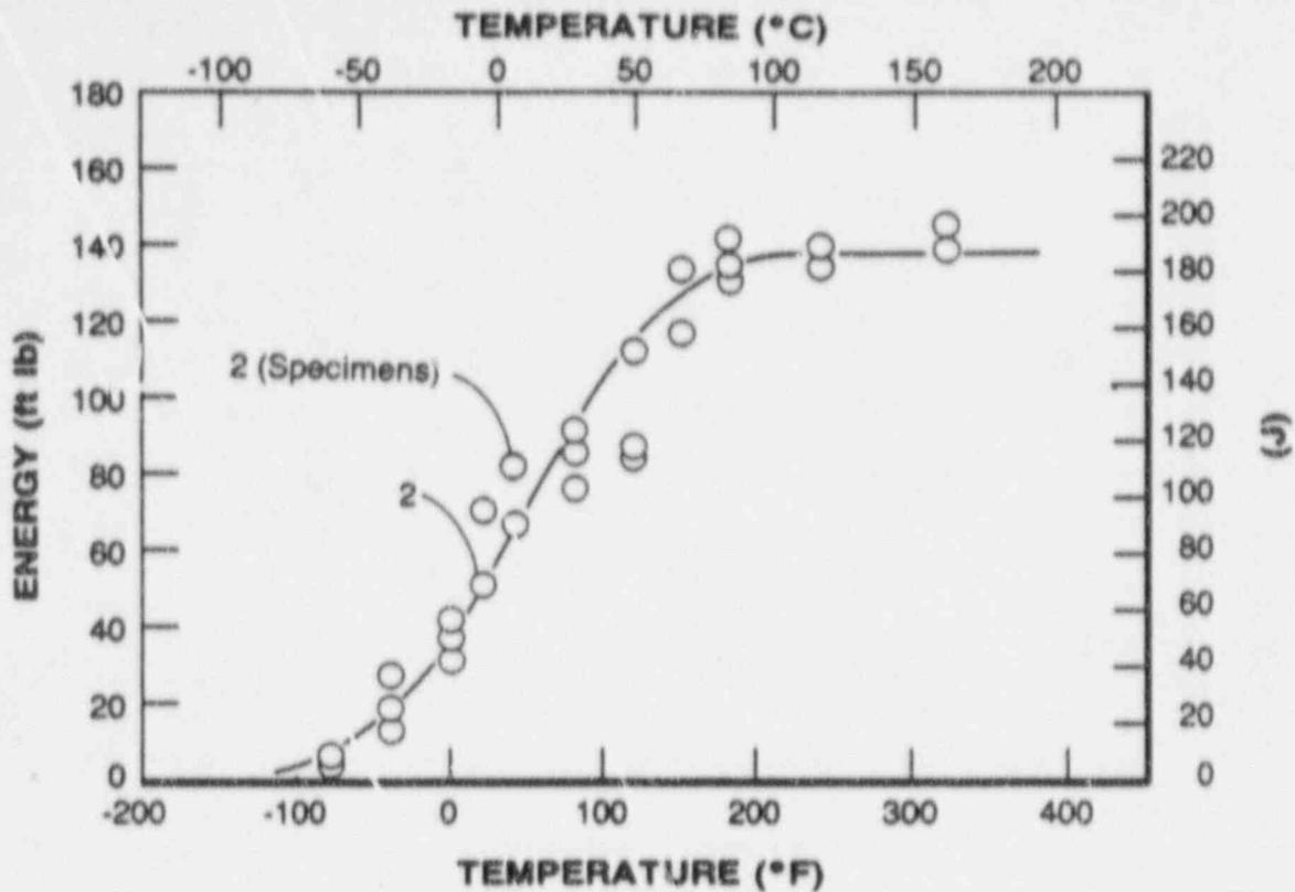
FIGURE 3-1. PREIRRADIATION CHARPY V-NOTCH IMPACT ENERGY FOR THE CATAWBA UNIT NO. 2 REACTOR PRESSURE VESSEL INTERMEDIATE SHELL PLATE B8605-1 (LONGITUDINAL ORIENTATION)
