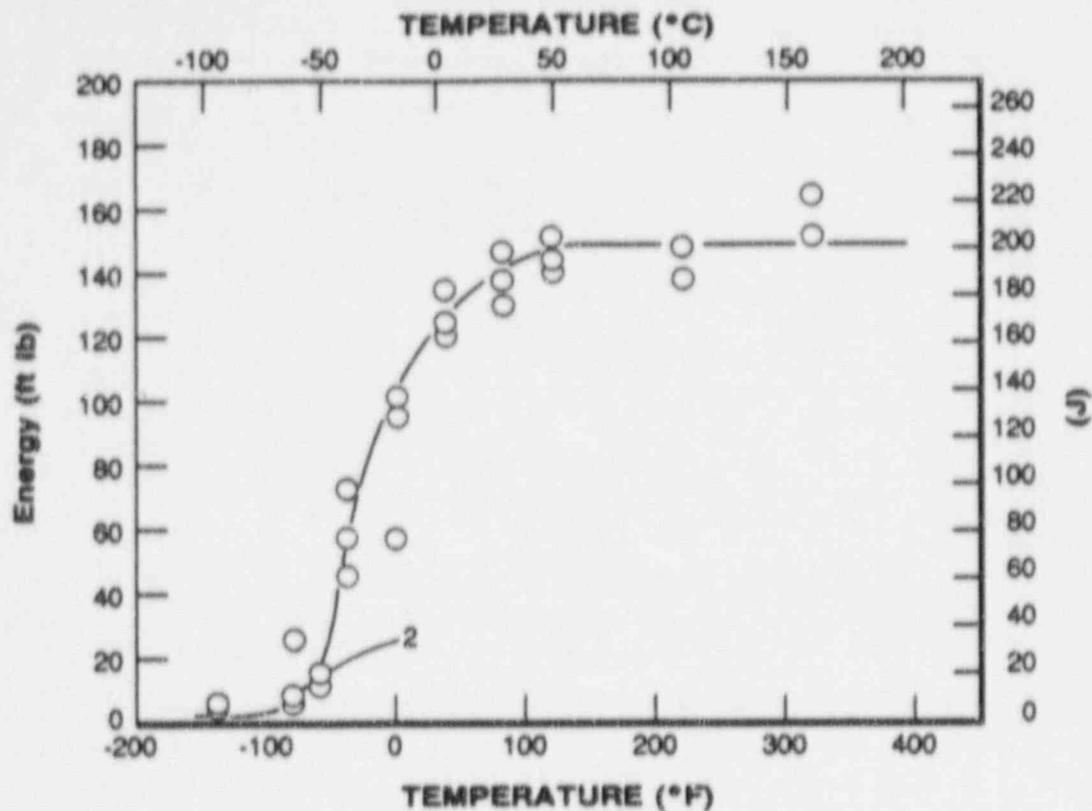
FIGURE 3-3. PREIRRADIATION CHARPY V-NOTCH IMPACT ENERGY FOR THE CATAWBA UNIT NO. 2 REACTOR PRESSURE VESSEL CORE REGION WELD METAL
