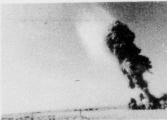
t = 1.0 sec. EJECTED MELT REACHES MAXIMUM HEIGHT. PARTICLES BEGIN SEPARATION FROM AEROSOL.
