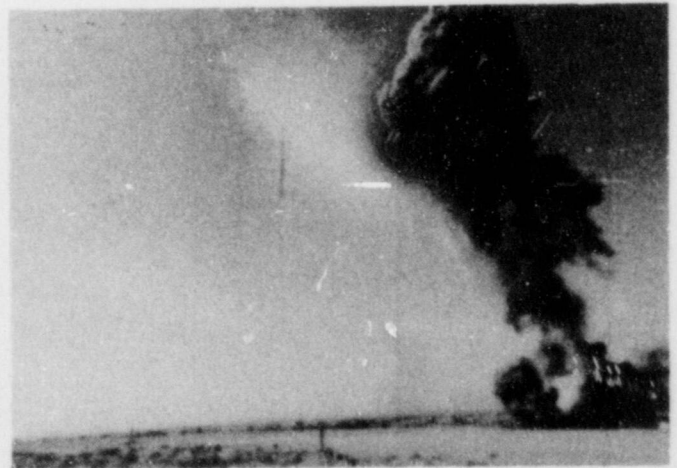
t = 1.5 sec. SEPARATION COMPLETE. PARTICLES FOLLOWING PARABOLIC TRAJECTORIES.
