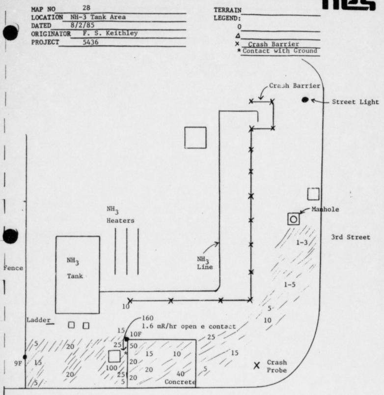
Remarks: \*Highly contaminated area (160,000 dpm/probe area) found at former catalyst loading area (concrete area). Contamination levels drop off as you move outward from this area. The contamination seems to have drained off towards manhole. Area by NH<sub>3</sub> heaters has a few spotty low level contamination, but area usually clean.
