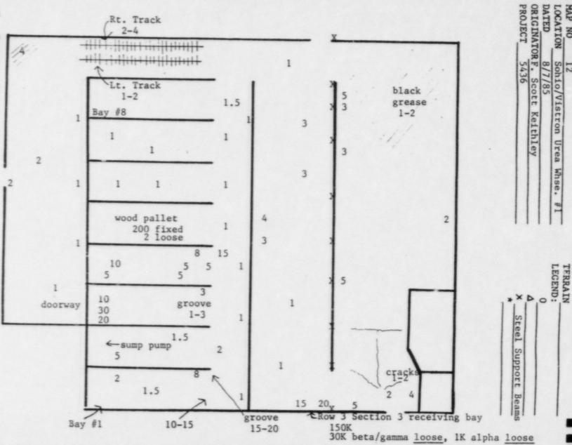
REMARKS: Highly contaminated wooden pallet found in Bay #5 (200K fixed; 2K loose - beta/gamma). Posted as radioactive material. Area near gas tanks highly contam., loose contam. detected. Posted area as radioactive materials area - no gas tanks & pipe to be removed from area. East end of warehouse has black grease with fixed contam. (1-2K). Fixed contam. usually fourn within concrete floor grooves & cracks.
