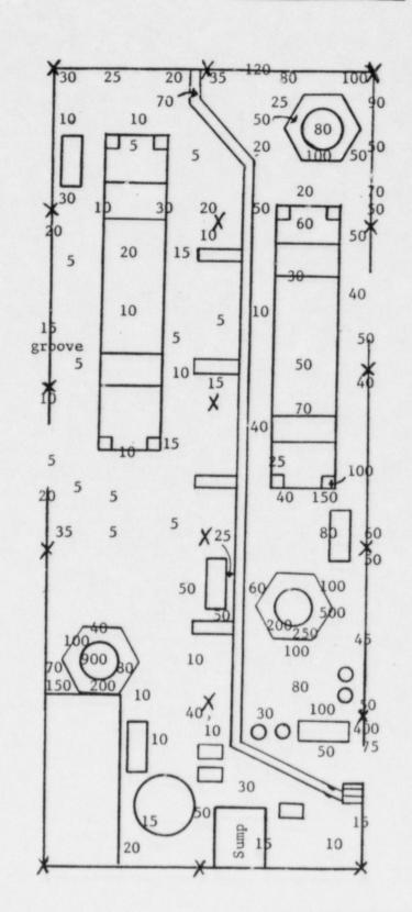
concrete bases. Also high levels of fixed contamination detected where the bases meet concrete All readings taken using RM-20 with HP-210 Entire area has gross tanks, pumps and calciners are secured to floor. High levels of fixed contamination detected at outside walls. High levels of fixed contamination detected where All readings are in (K) thousand dpm/probe area. fixed contamination within concrete floor.
