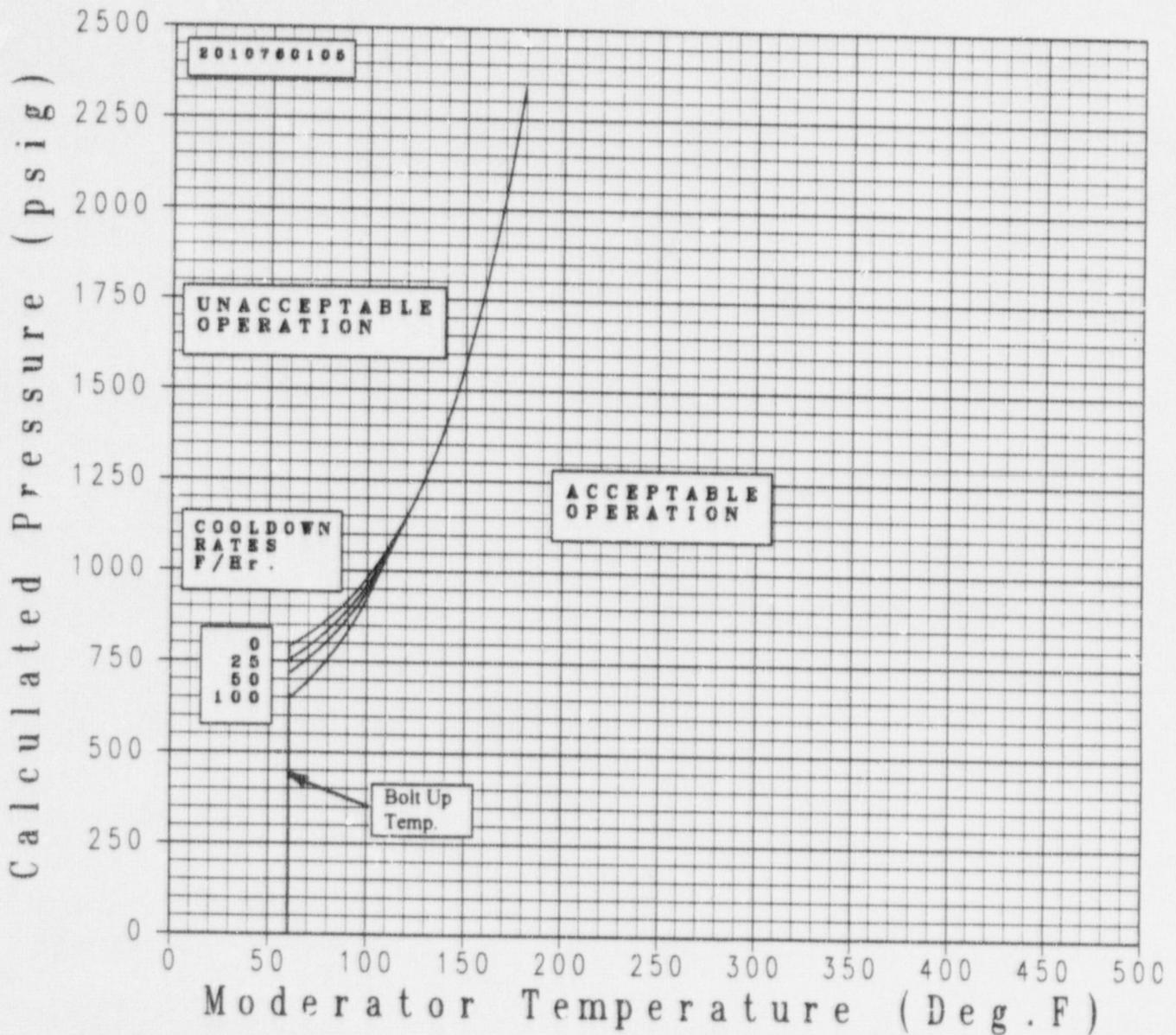
FIGURE 5-4 V. C. Summer Unit 1 Reactor Coolant System Cooldown Limitations (Cooldown Rates of 0, 25, 50 and 100°F/hr) Applicable to 32 EFY (Without Margins for Instrumentation Errors)
