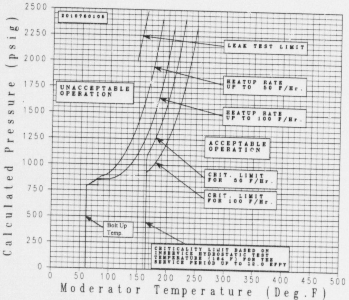
FIGURE 5-3 V. C. Summer Unit 1 Reactor Coolant System Heatup Limitations (Heatup Rate of 50 and 100°F/hr) Applicable to 32 EFPY (Without Margins for instrumentation Errors)
