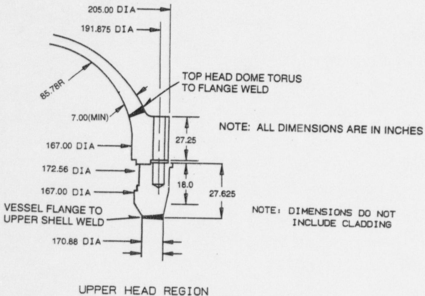
Figure 3-1 Geometry of the Upper Head/Flange Region of a Typical Westinghouse Four Loop Plant Reactor Vessel
