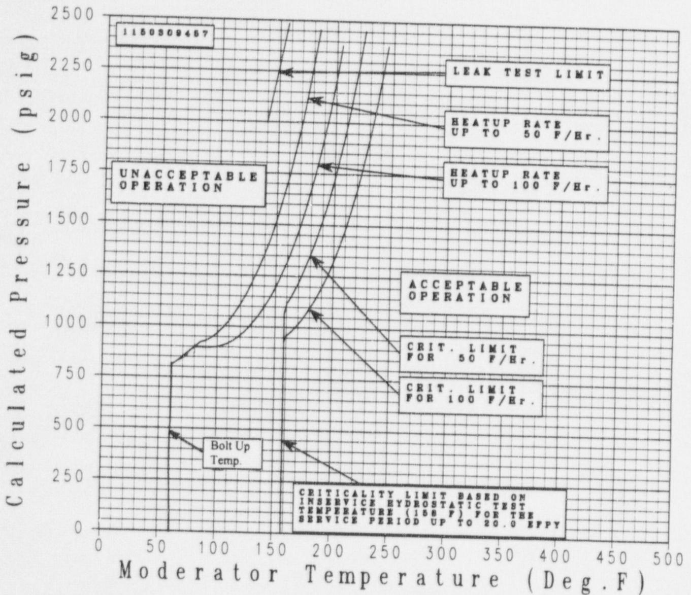
FIGURE 5-1 V. C. Summer Unit 1 Reactor Coolant System Heatup Limitations (Heatup Rates of 50 and 100°F/hr) Applicable to 20 EFPY (Without Margins for Instrumentation Errors)
