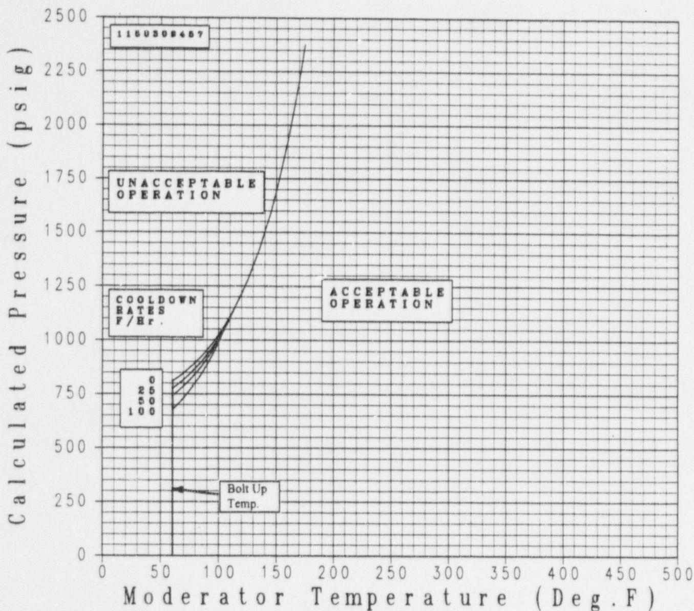
FIGURE 5-2 V. C. Summer Unit 1 Reactor Coolant System Cooldown Limitations (Cooldown Rates of 0, 25, 50 and 100°F/hr) Applicable to 20 EFPY (Without Margins for Instrumentation Errors)
