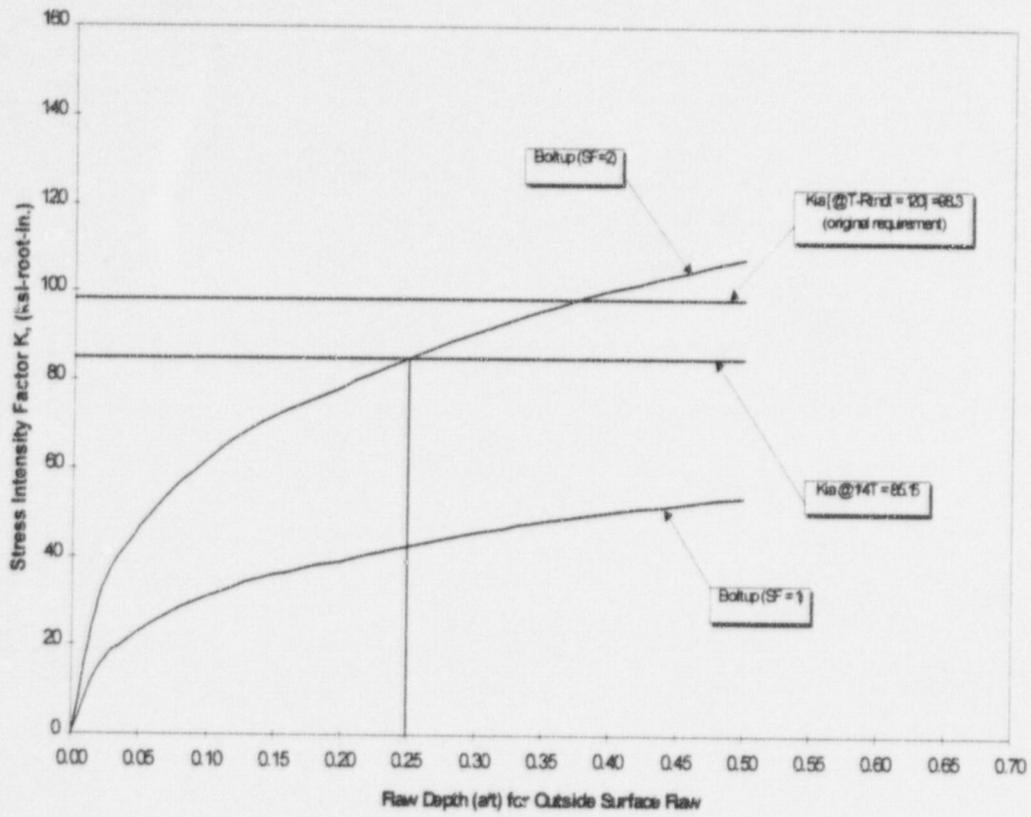
Figure 3-2 Crack Driving Force as a Function of Flaw Size: Outside Surface Flaw in the Closure Head to Flange Region Weld
