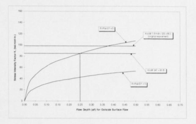
Figure 2. Crack Driving Force as a Function of Flaw Size: Outside Surface Flaw in the Closure Head to Flange Region Weld
