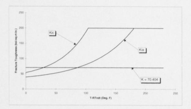
Figure 5. Determination of Boltup Requirement, Three Loop plant, using KIC
