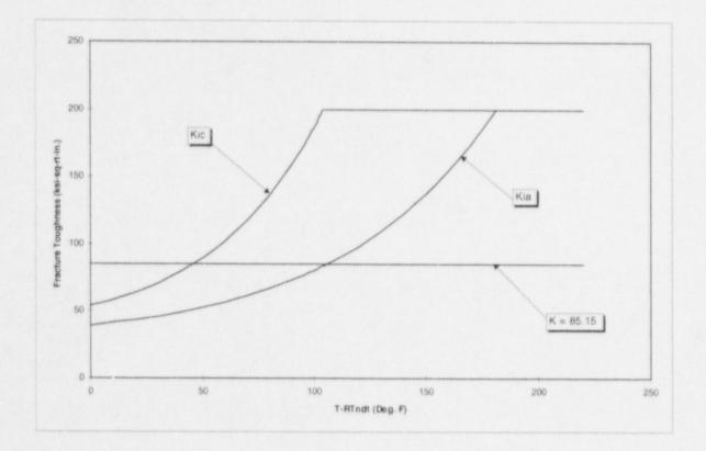
Figure 3. Determination of Boltup Requirement, Four Loop plant, using KIC
