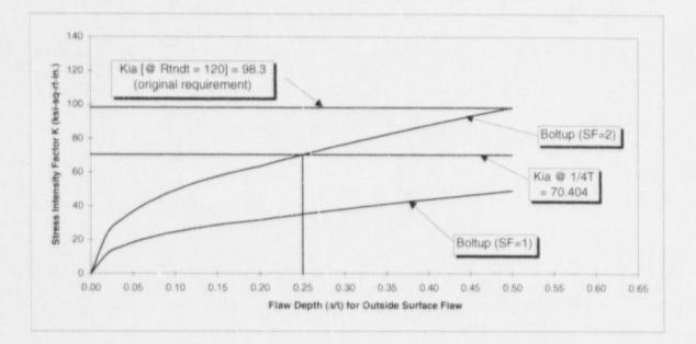
Figure 4. Crack Driving Force as a Function of Flaw Size: Outside Surface Flaw in the Closure Head to Flange Region Weld, Three Loop plant Document Control Desk Attachment 2 NRR 990009 RC-99-0152 Page 9 of 9
