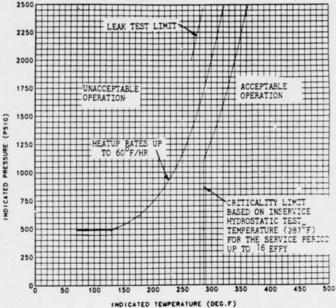
Figure 5 Farley Unit 1 Reactor Coolant System Heatup Limitations Applicable for the First 16 EFY
