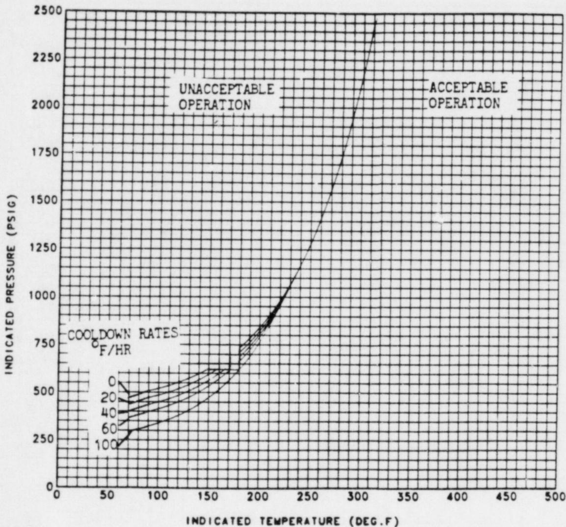
Figure 6 Farley Unit 1 Reactor Coolant System Cooldown Limitations Applicable for the First 16 EFY
