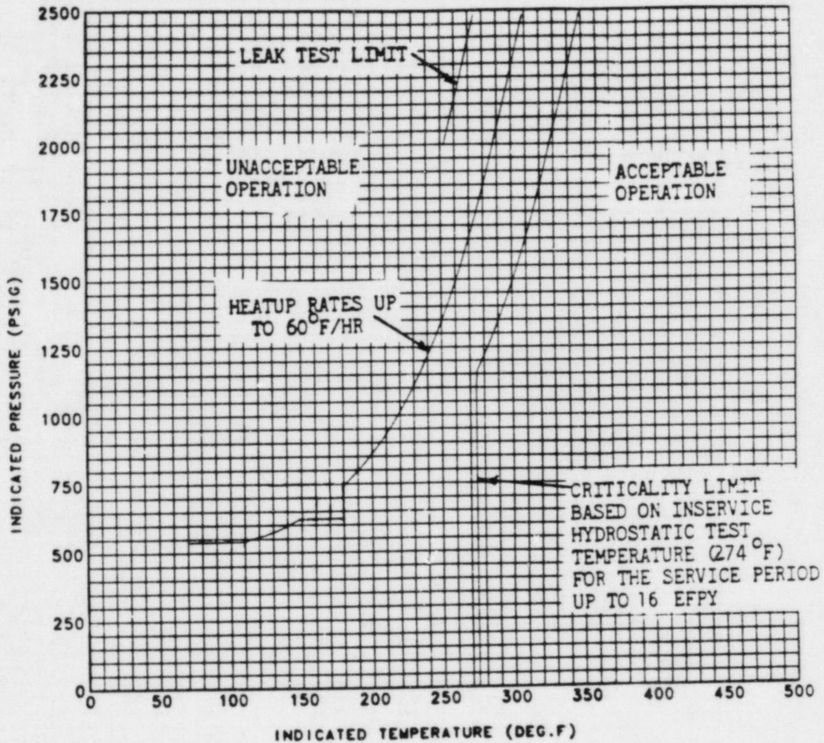
Figure 9 Farley Unit 1 Reactor Coolant System Heatup Limitations Applicable for the First 16 EFPY
