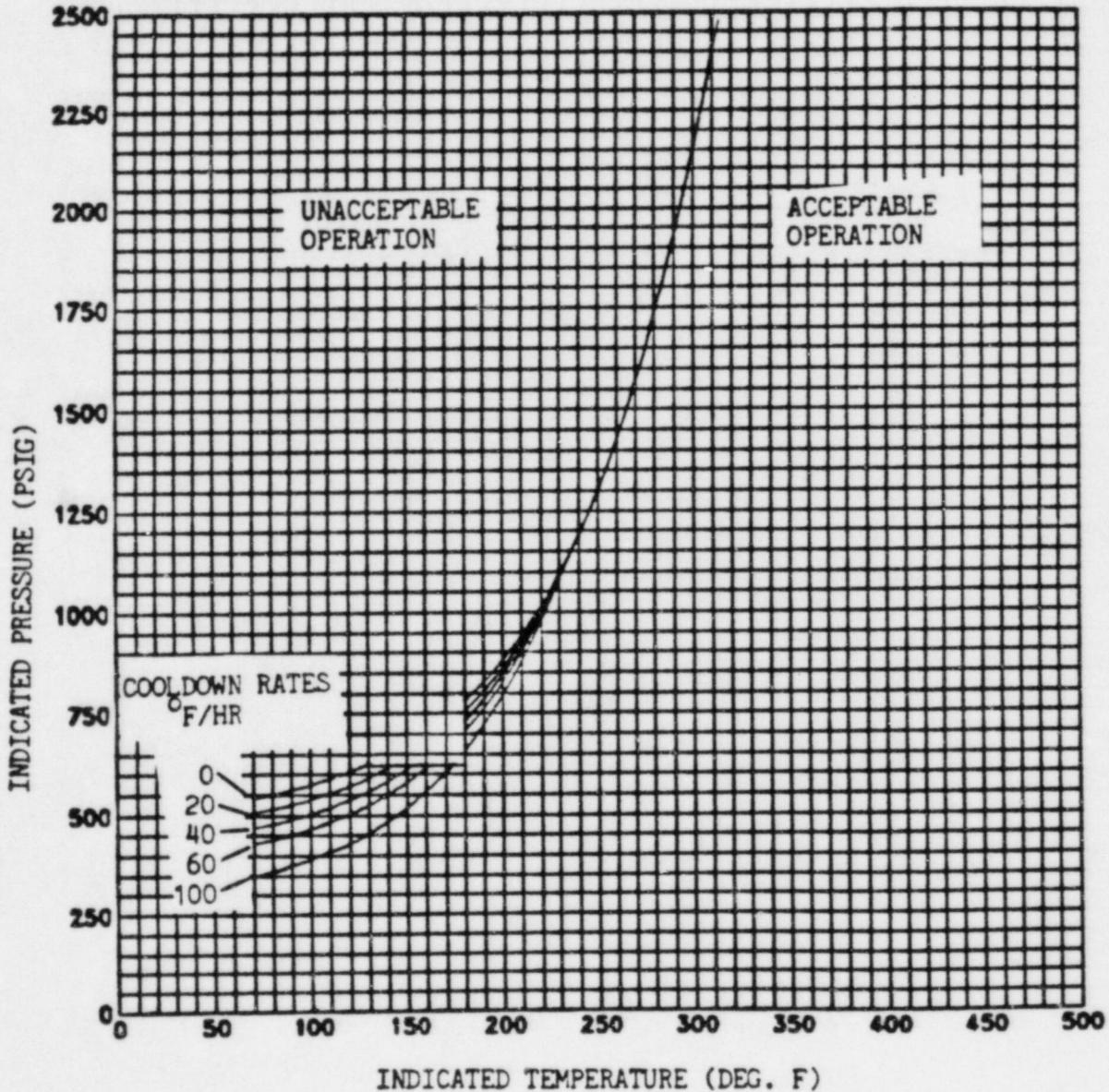
Figure 12 Farley Unit 1 Reactor Coolant System Cooldown Limitations Applicable for up to 32 EFPY
