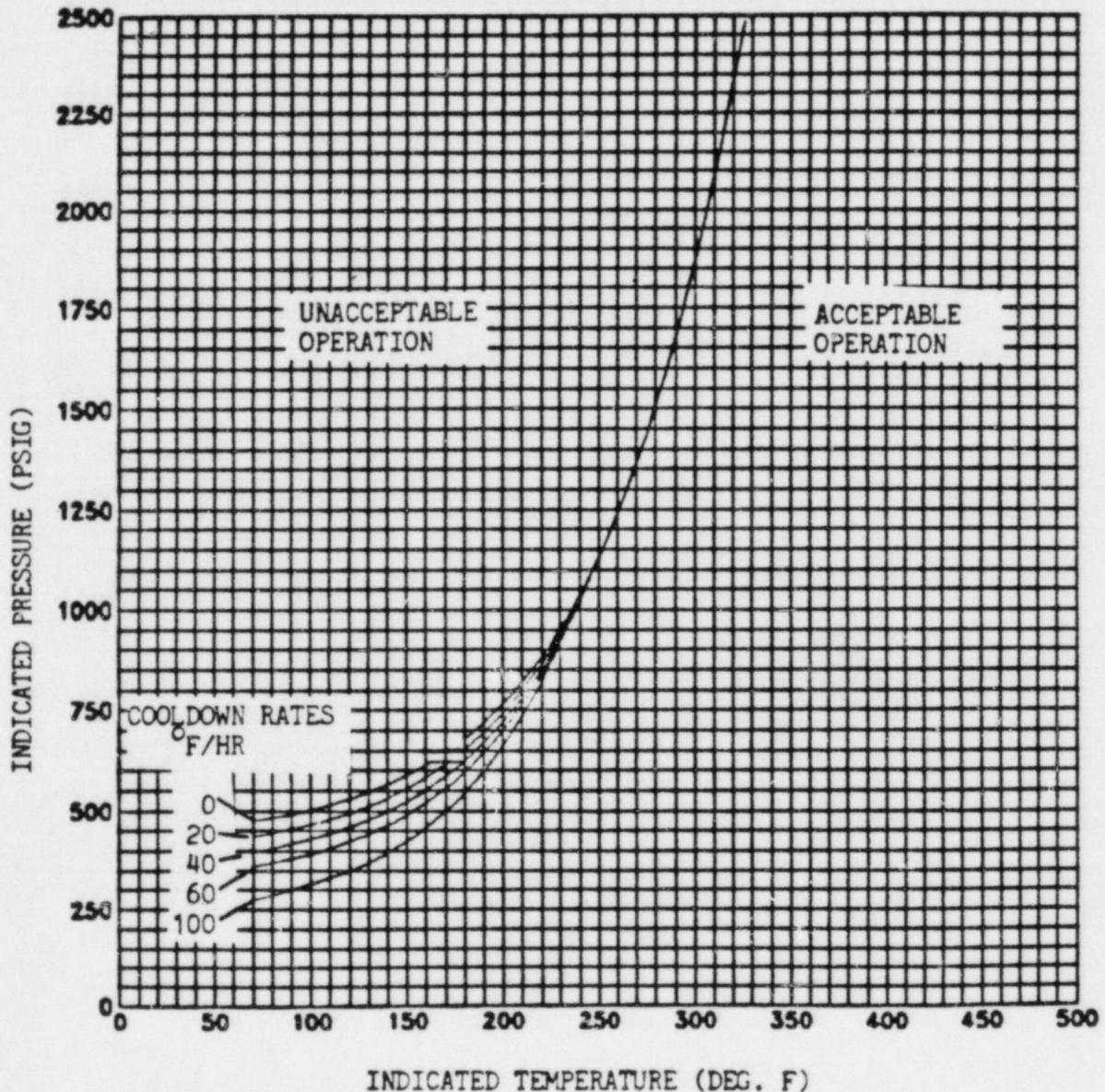
Figure 8 Farley Unit 1 Reactor Coolant System Cooldown Limitations Applicable for up to 32 EFPY
