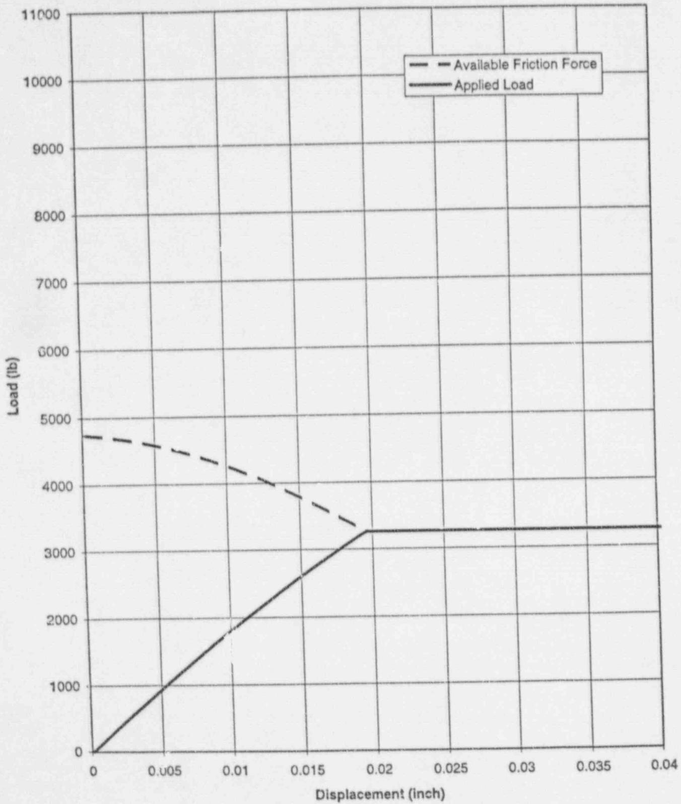
Figure 3-5. Load History for Friction Force and Applied Load for 4-inch Long Expansion (Prequalification Tests)
