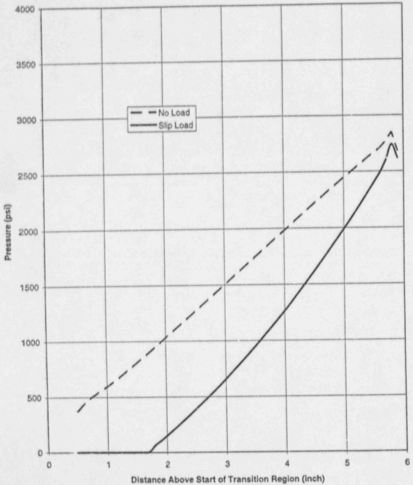
Figure 3-18. Contact Pressure for Mid-Radius OTSG Tubes With 22-inch Expansion Region
