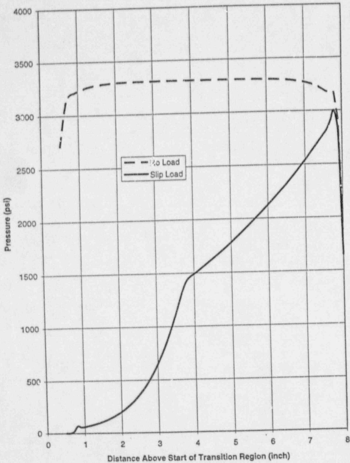
Figure 3-3. Contact Pressure Distribution for 8-inch Long Expansion (Prequalification Tests)
