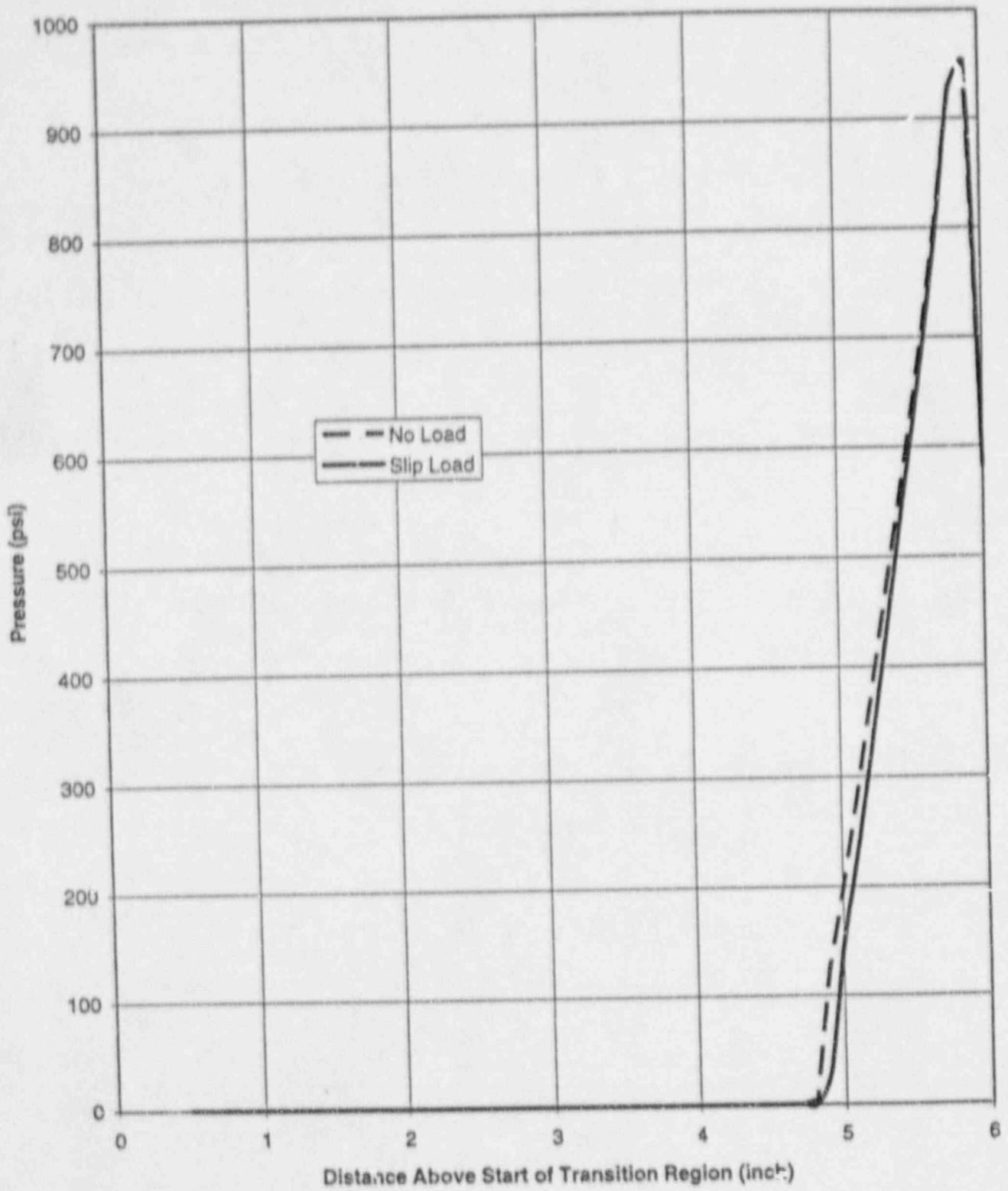
Figure 3-17. Contact Pressure for Center OTSG Tubes With 22-inch Expansion Region
