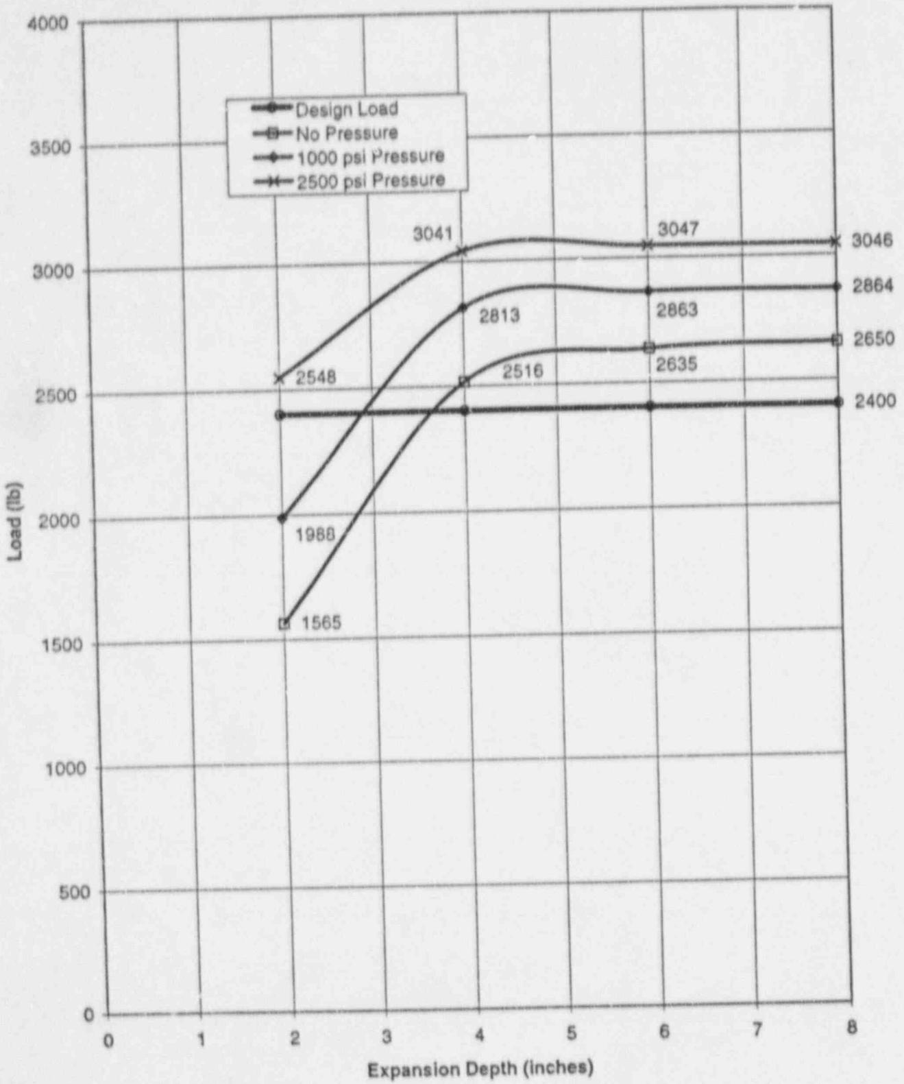
Figure 3-11. Pullout Load Versus Expansion Length for Peripheral OTSG Tubes
