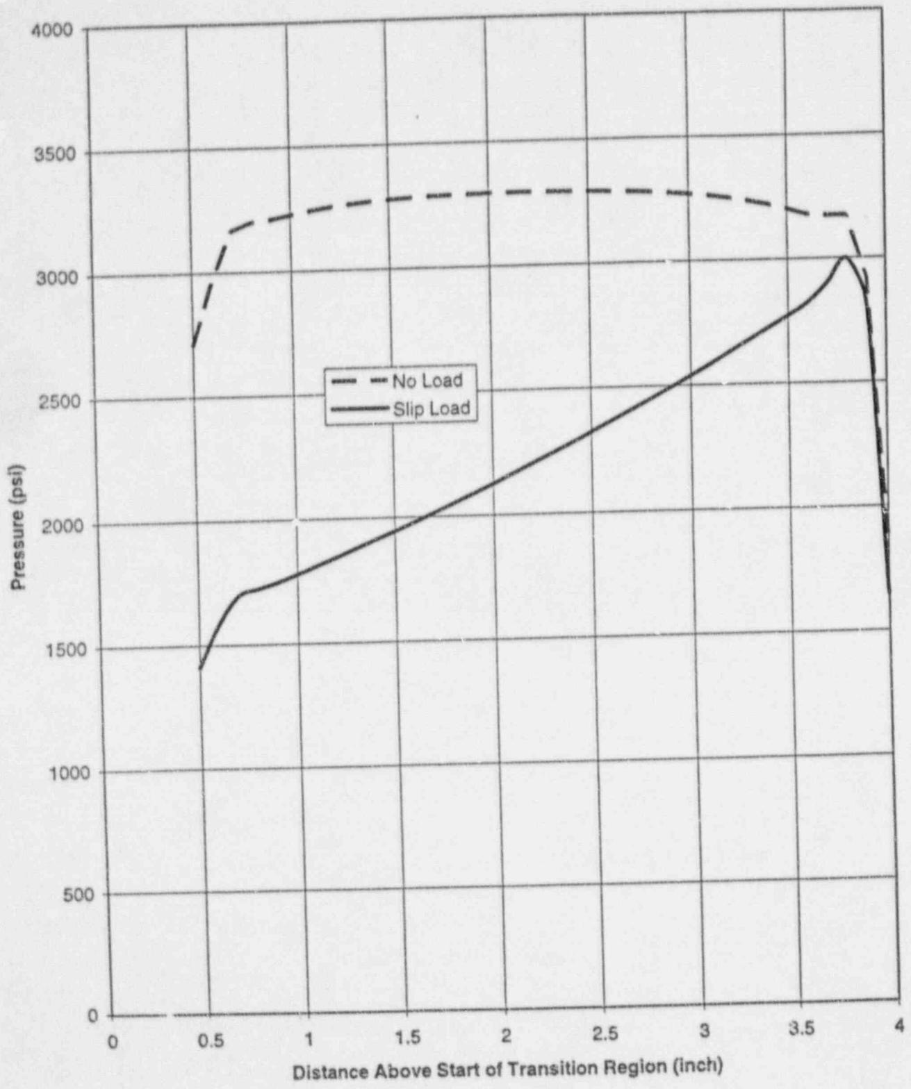
Figure 3-1. Contact Pressure Distribution for 4-inch Long Expansion (Prequalification Tests)
