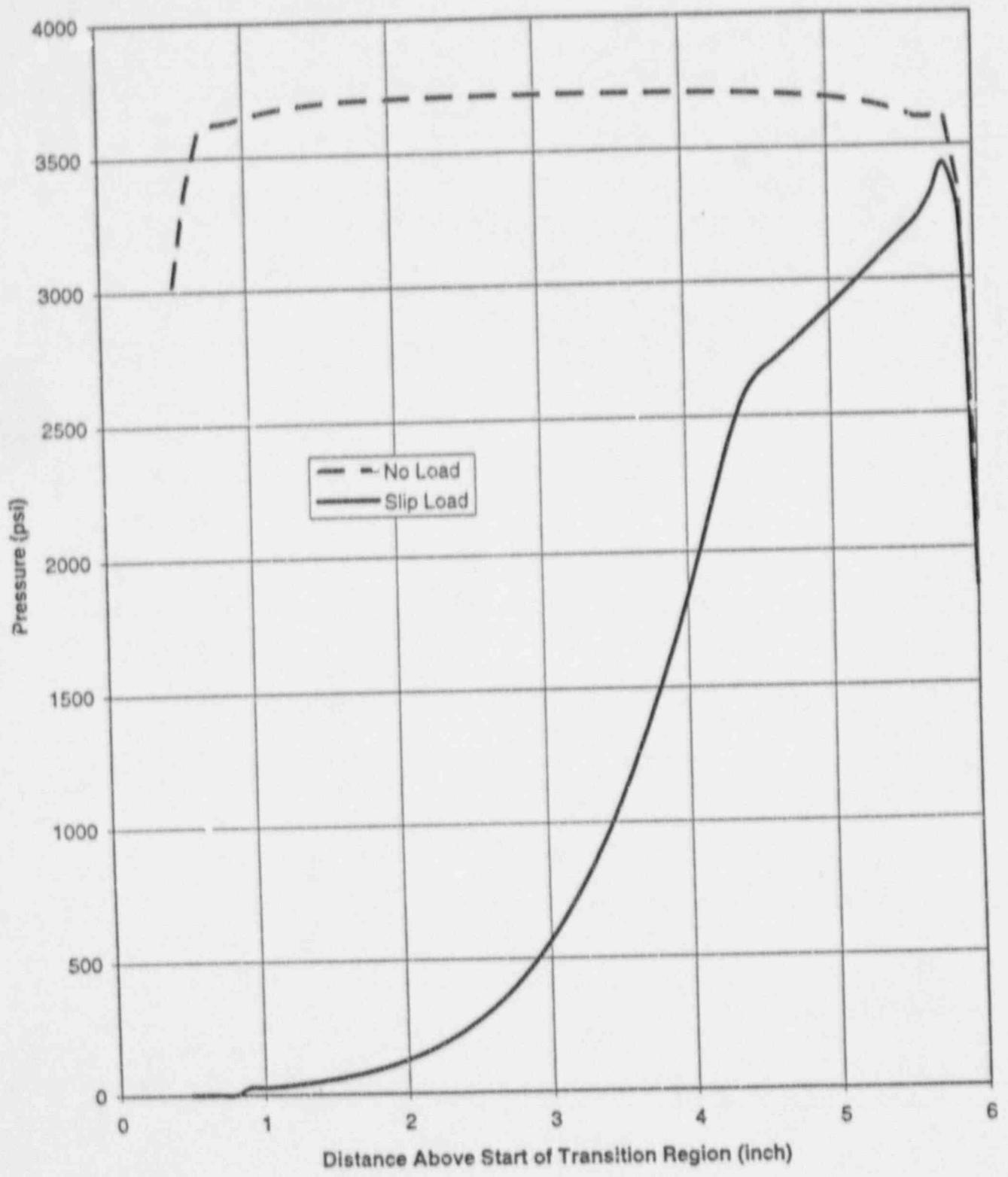
Figure 3-10. Contact Pressure Distribution - 1000 Psi Internal Pressure (Peripheral OTSG Tubes)
