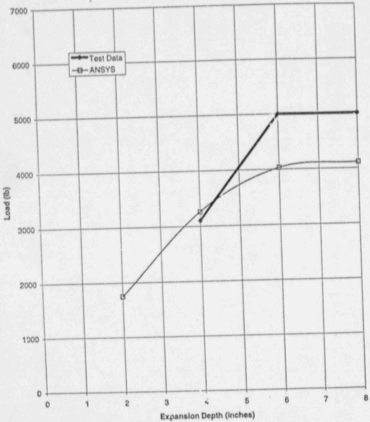
Figure 3-8. Pullout Load Versus Expansion Length for Prequalification Tests
