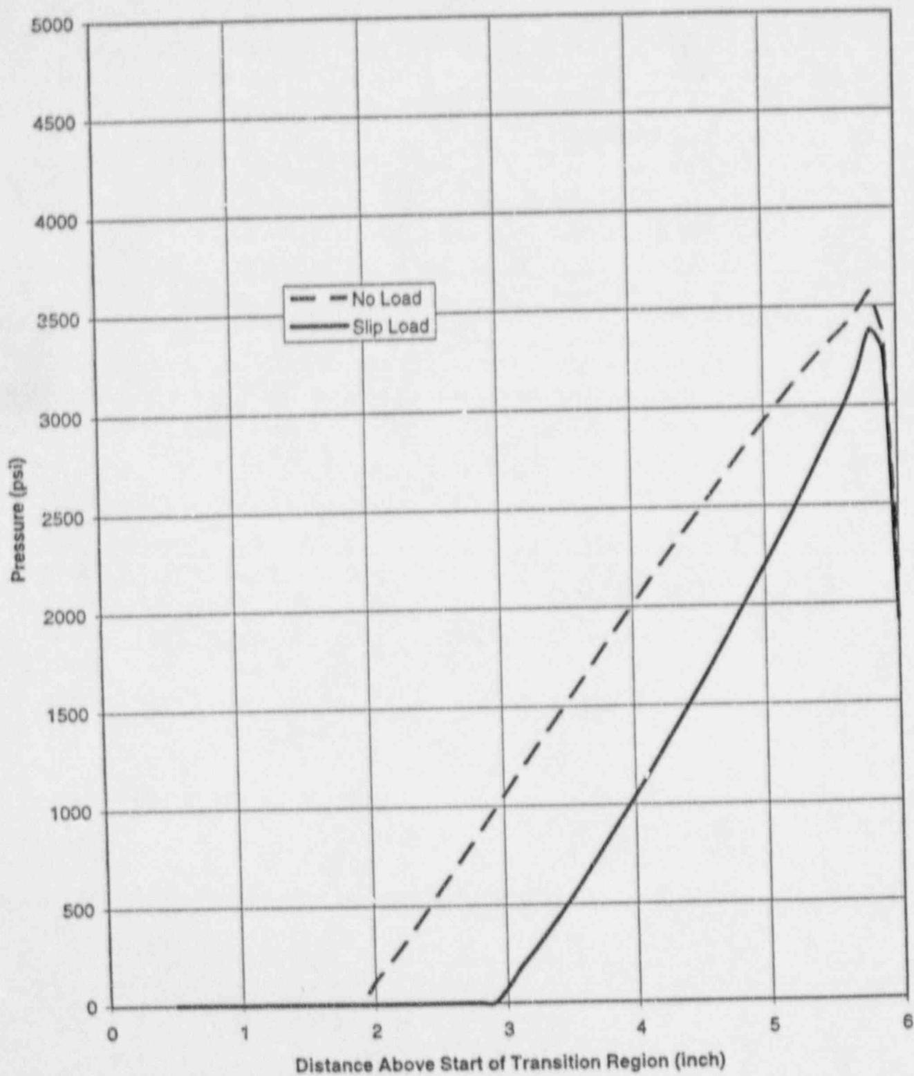
Figure 3-13. Contact Pressure for 6-inch Long Expansion With Tubesheet Bow (Center OTSG Tubes)
