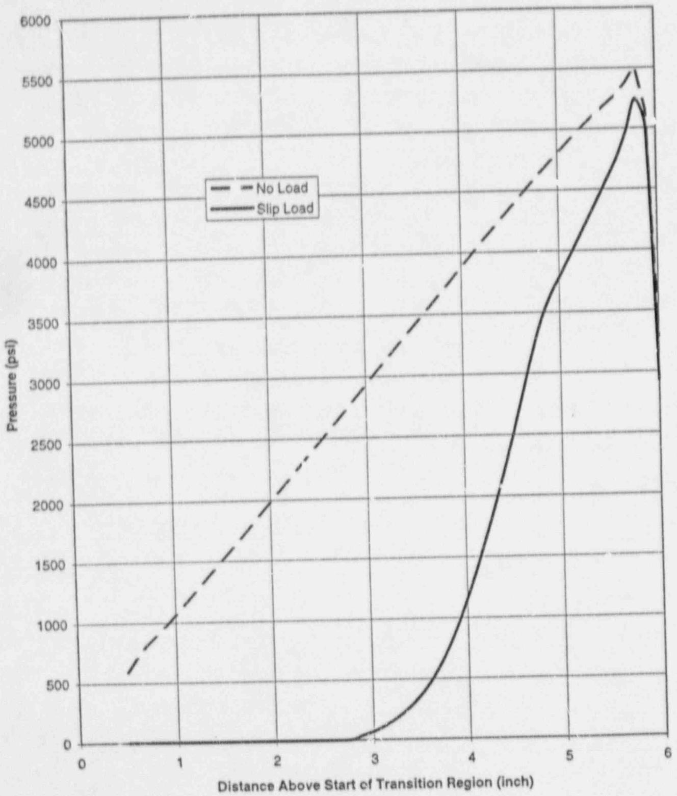
Figure 3-14. Contact Pressure for 6-inch Long Expansion With Tubesheet Bow and 2500 Psi Internal Pressure (Center OTSG Tubes)
