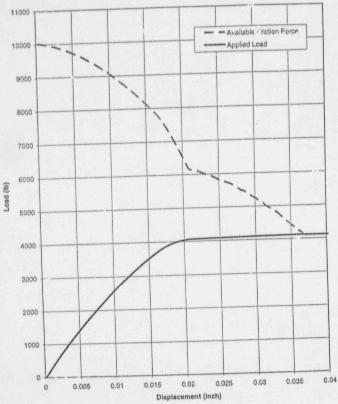
Figure 3-7. Load History for Friction Force and Applied Load for 8-inch Long Expansion (Prequalification Tests)
