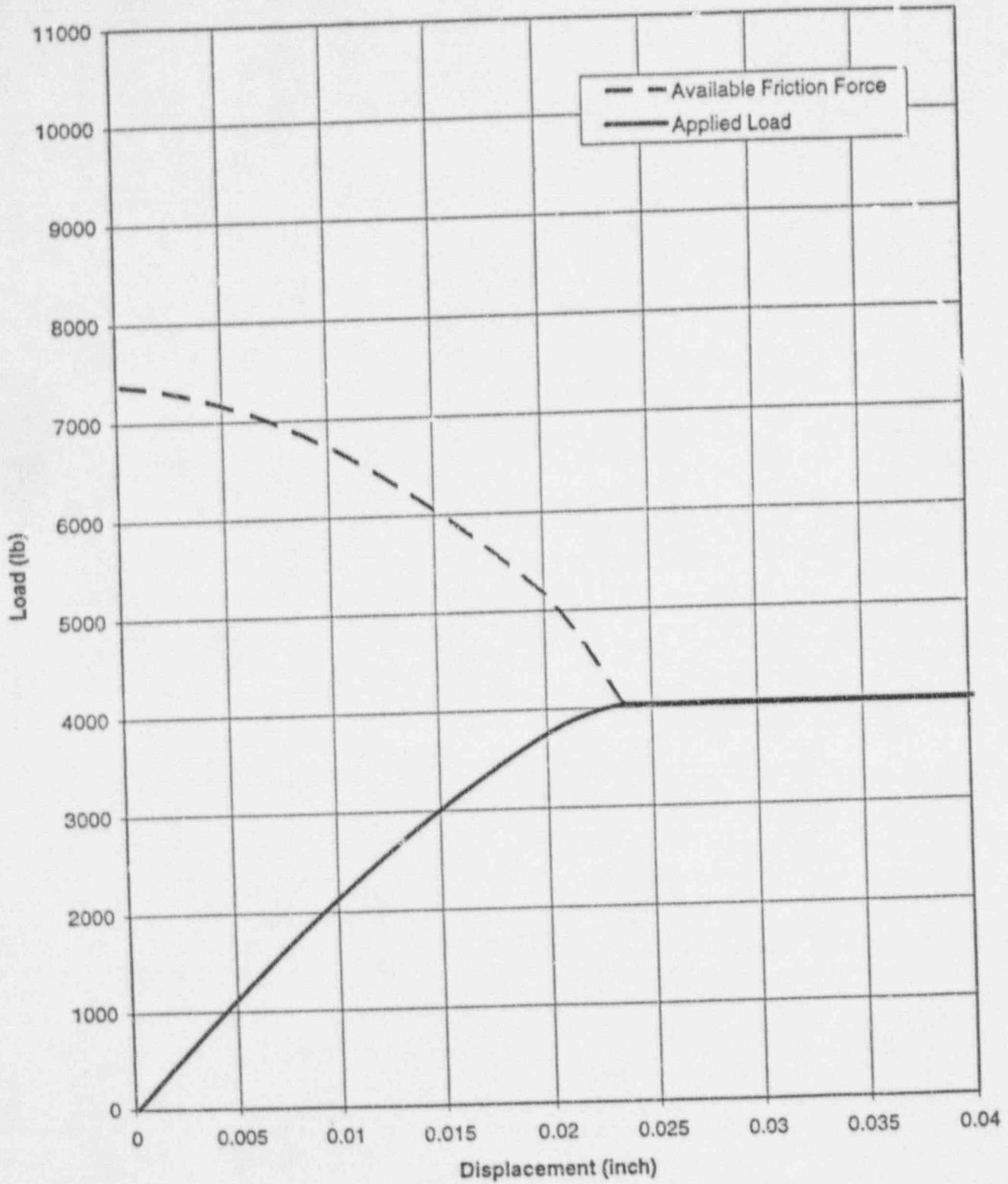
Figure 3-6. Load History for Friction Force and Applied Load for 6-inch Long Expansion (Prequalification Tests)
