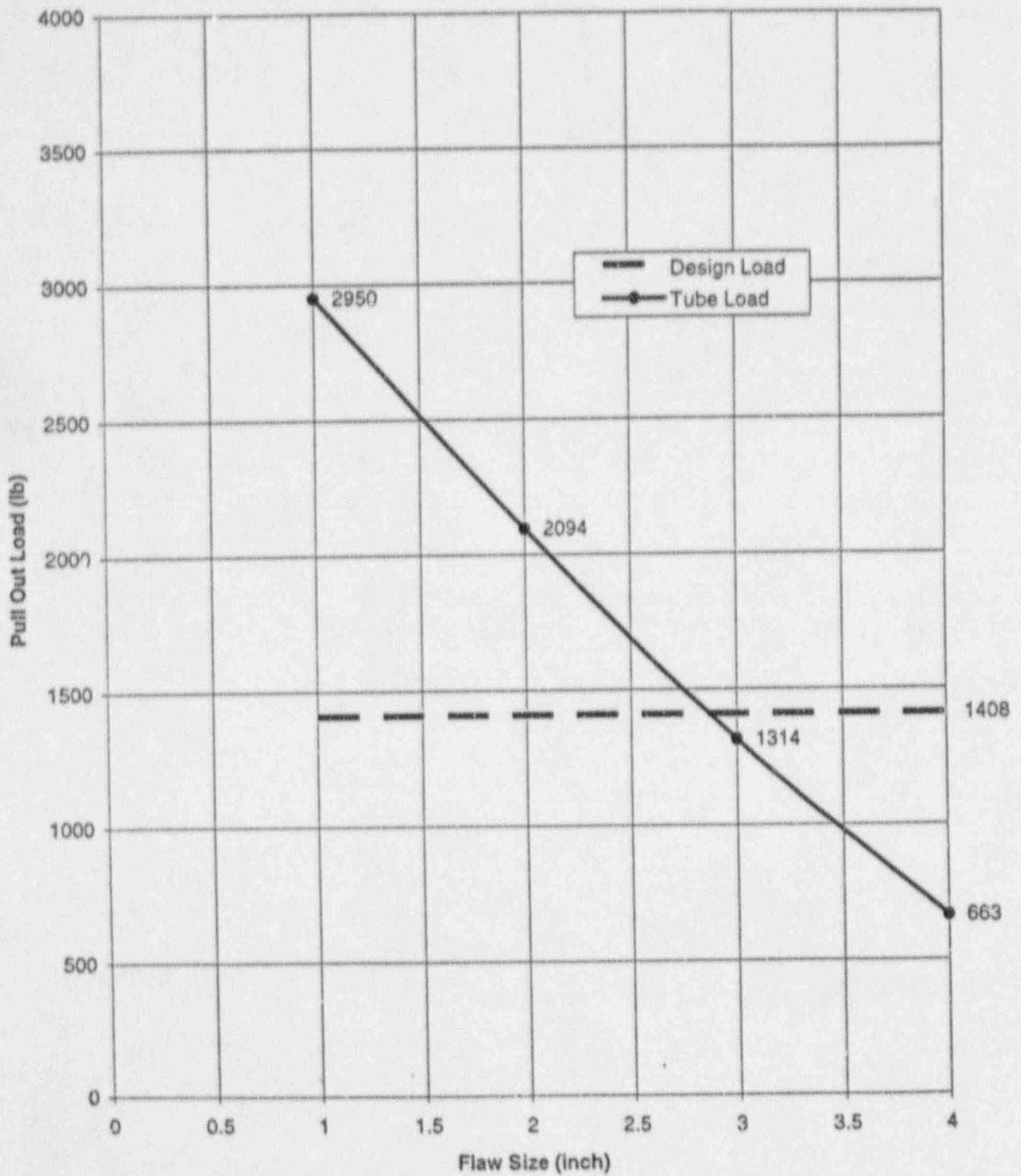
Figure 3-15. Pullout Load for Center OTSG Tubes With 17-inch Expansion Region
