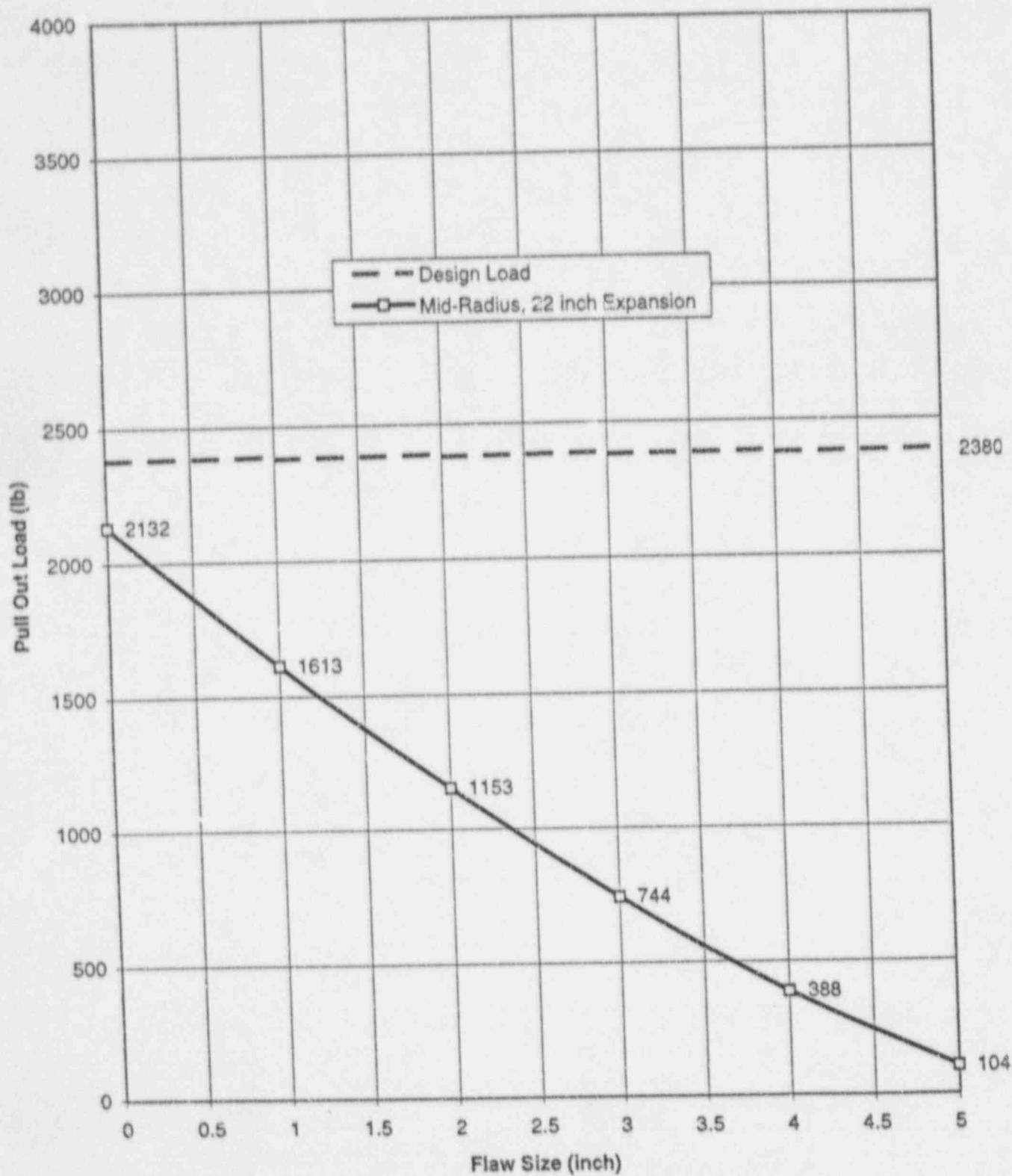
Figure 3-19. Pullout Load for Mid-Radius OTSG Tubes With 22-inch Expansion Region
