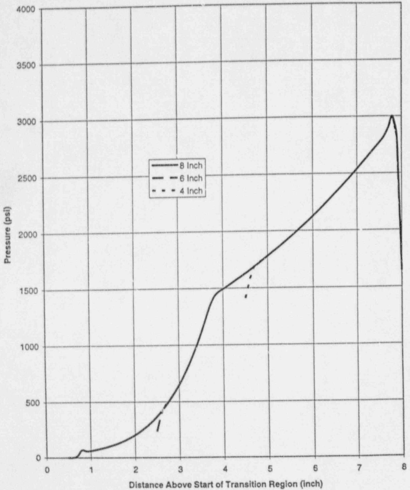
Figure 3-4. Contact Pressure Distribution for 4-, 6- and 8-inch Long Expansion (Prequalification Tests)
