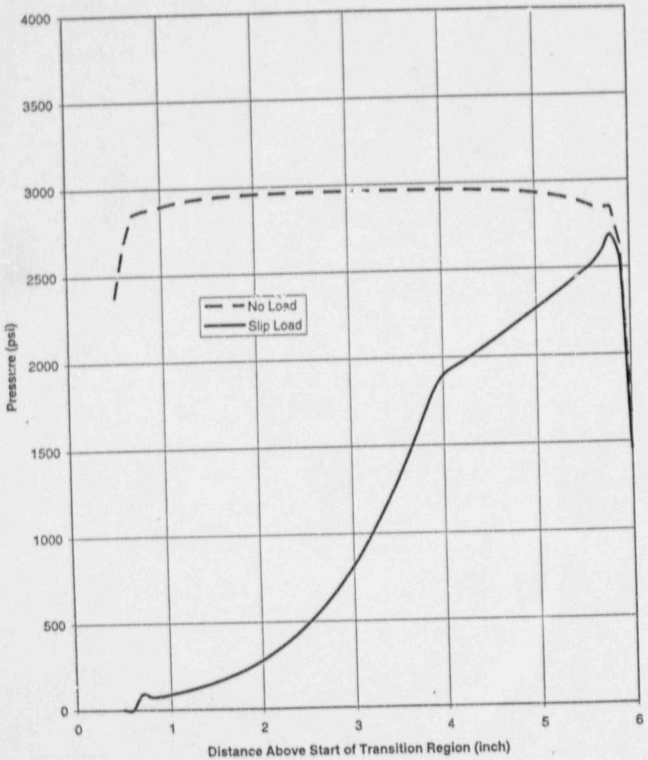
Figure 3-9. Contact Pressure Distribution for 6-inch Long Expansion (Peripheral OTSG Tubes)
