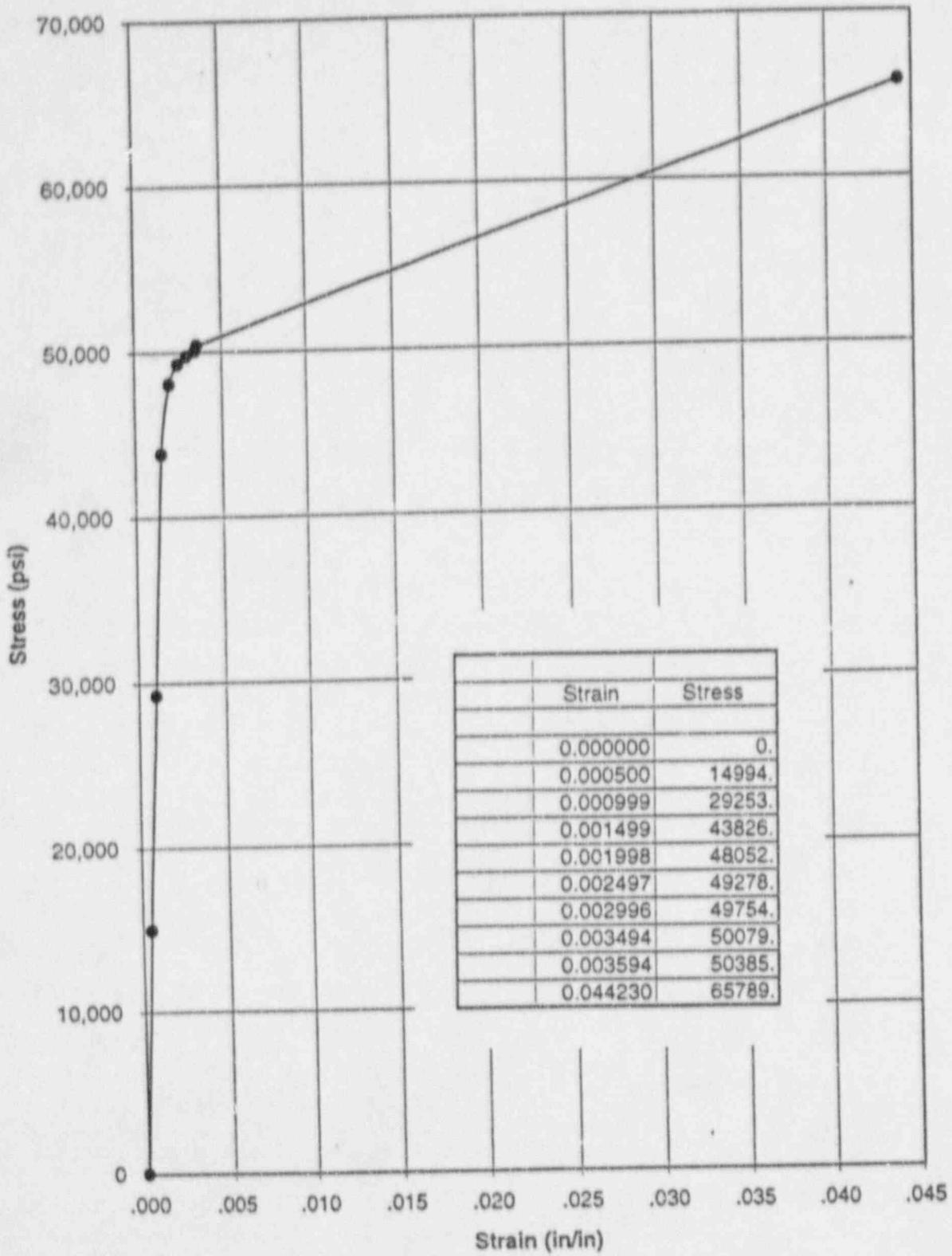
Figure 3-21. True Stress Versus True Strain for Typical Tube Material
