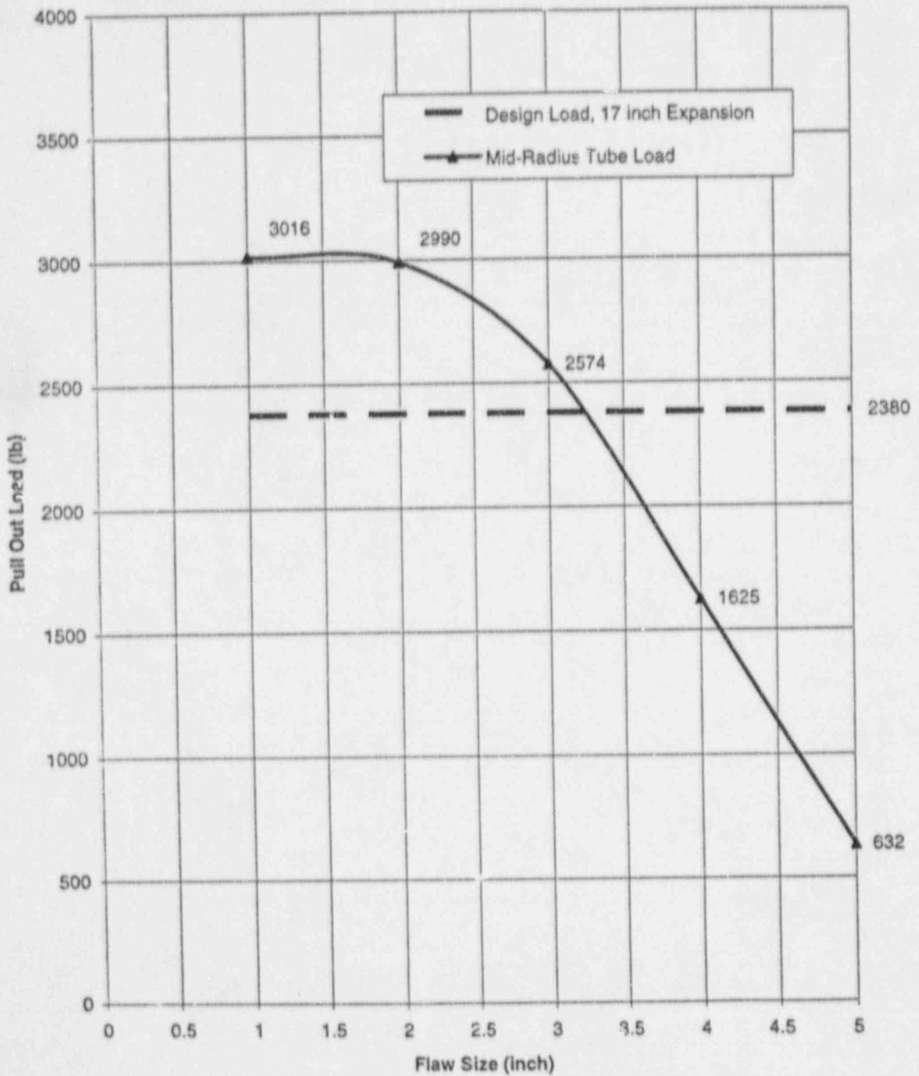
Figure 3-16. Pullout Load for Mid-Radius OTSG Tubes With 17-inch Expansion Region
