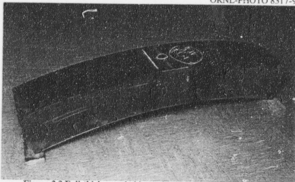
Figure 2.3 Full-thickness clad beam blank before final machining
