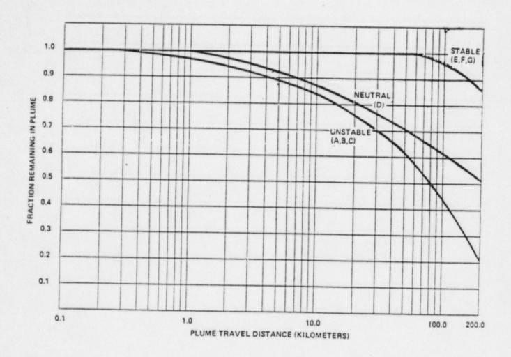
Plume Depletion Effect for 100-Meter Releases
