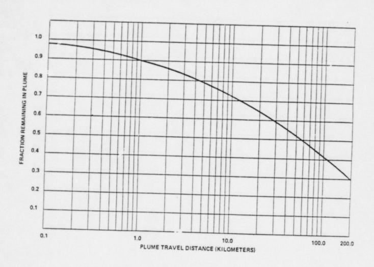
Plume Depletion Effect for 30-Meter Releases
