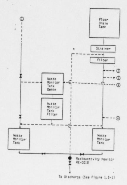
\*Dotted lines indicate alternate routes for increased operational flexibility and/or additional processing.
