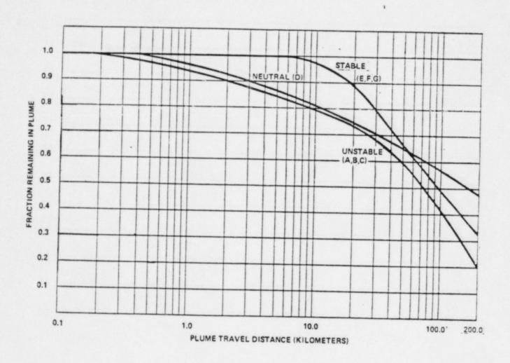
Plume Depletion Effect for 60-Meter Releases
