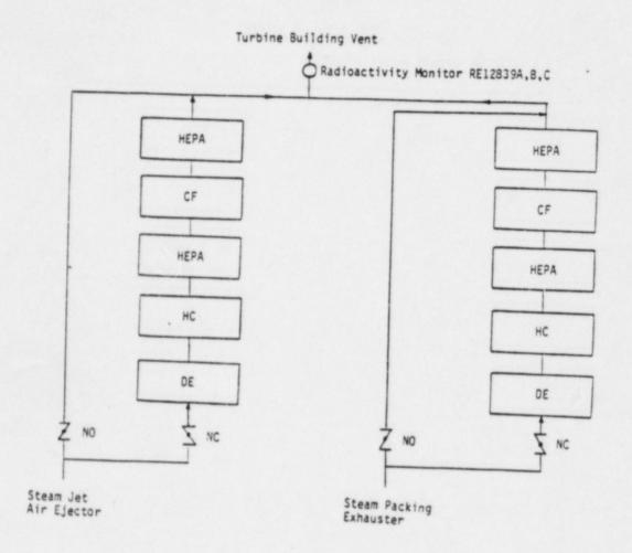
HEPA -High Efficiency Particulate Air Filter
