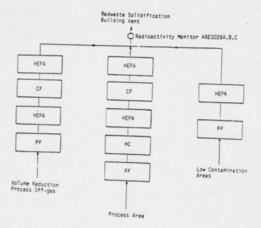
HEPA -High Efficiency Particulate Air Filter
