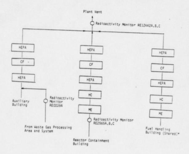
HEPA -High Efficiency Particulate Air Filter
