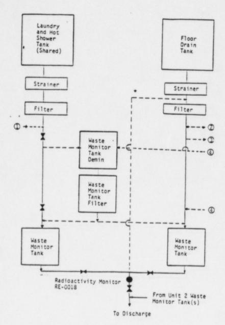
\*Dotted lines indicate alternate routes for increased operational flexibility
