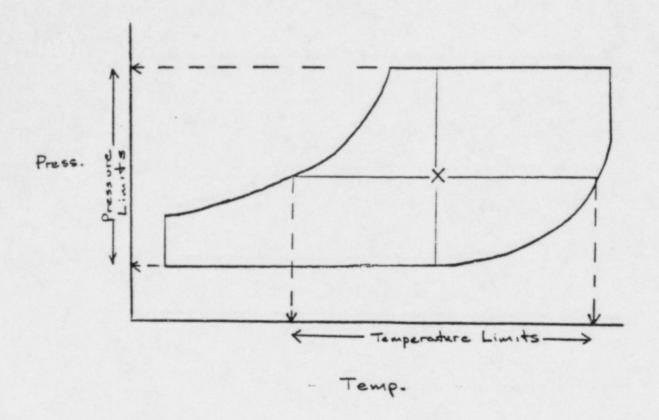
RCS PRESSURE LIMITS - DETERMINED BY THE HEIGHT OF THE ACCEPTABLE REGION AT RCS AVERAGE TEMPERATURE
