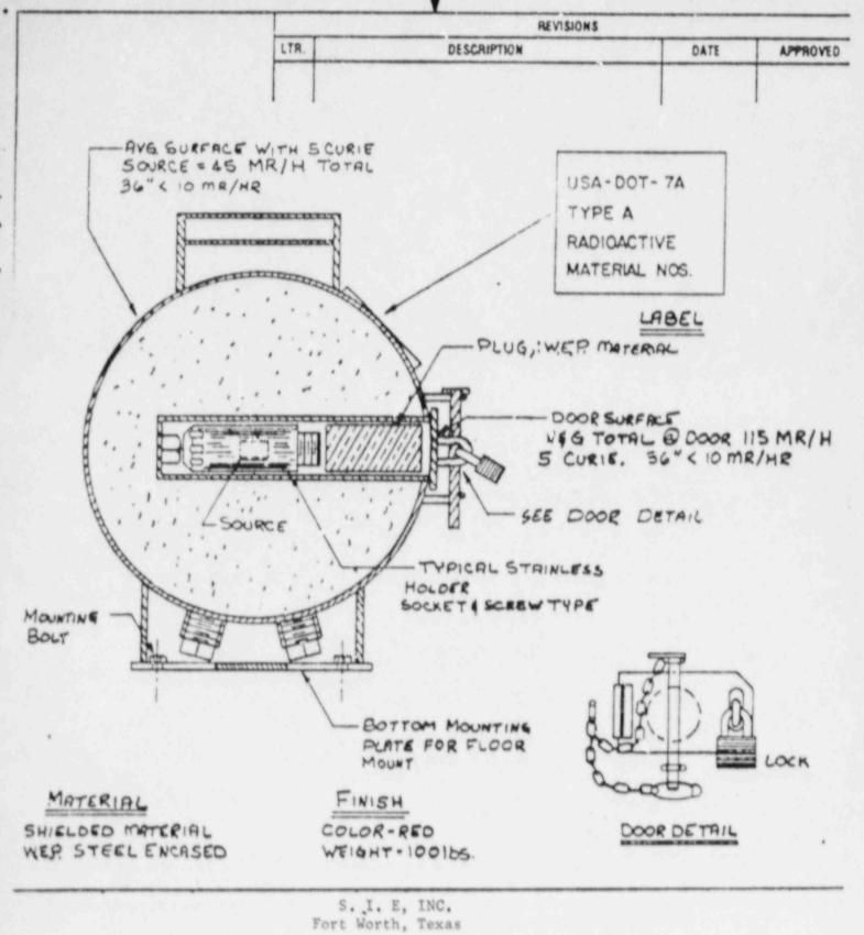
3 or 5 Curies AmBe Neutron Storage Shield 14" Diameter Spherical
