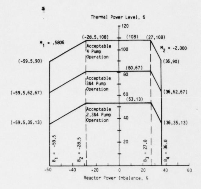
TMI-1 Protection System Maximum Allowable Setpoints for Reactor Power Imbalance, Cycle 5
