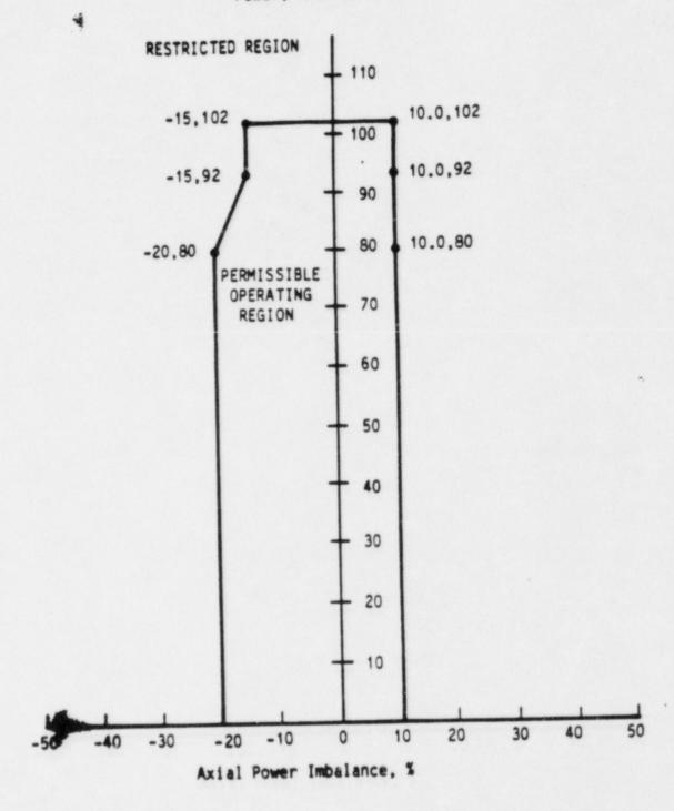
Power Imbalance Envelope for Operation From 0 EFPD to 250 ±10 EFPD, Cycle 5
