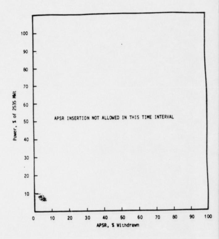
APSR Position Limits for Operation After 250 ± 10 EFPO, Cycle 5
