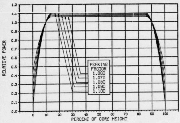
CLASS 2 TYPE: DOUBLE-HUMPED SYMMETRIC, HIGH POWER AFTER PEAK
