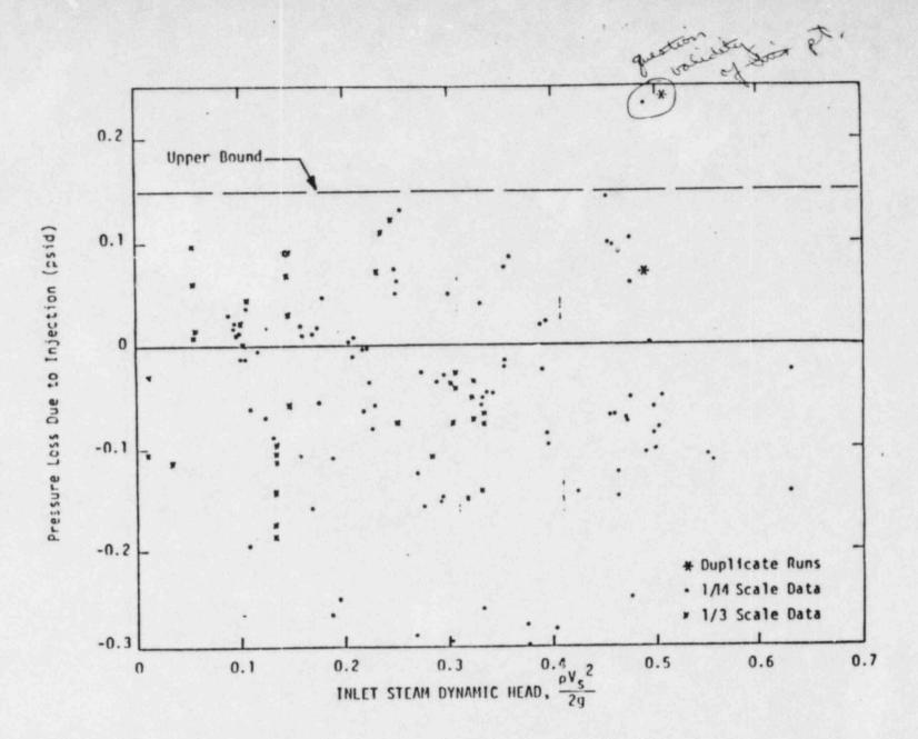
Pressure Loss Due to Pumped Safety Injection
