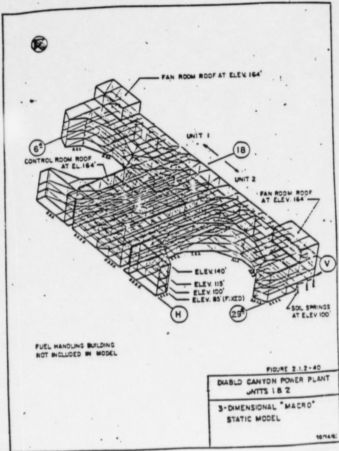
Fig. 3.9 3-D Detailed FEM Model for Auxiliary Building (Ref. 4)
