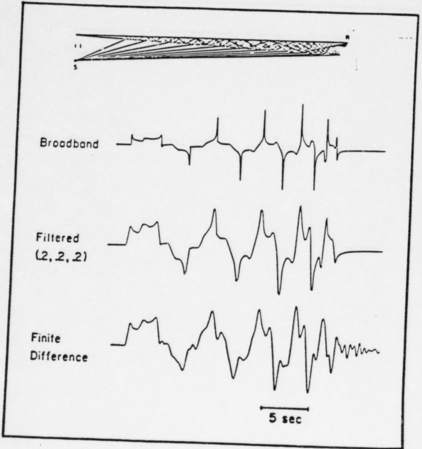
Figure 26 Comparison of GRT results with finite difference calculations (after Vidale et al., 1985).
