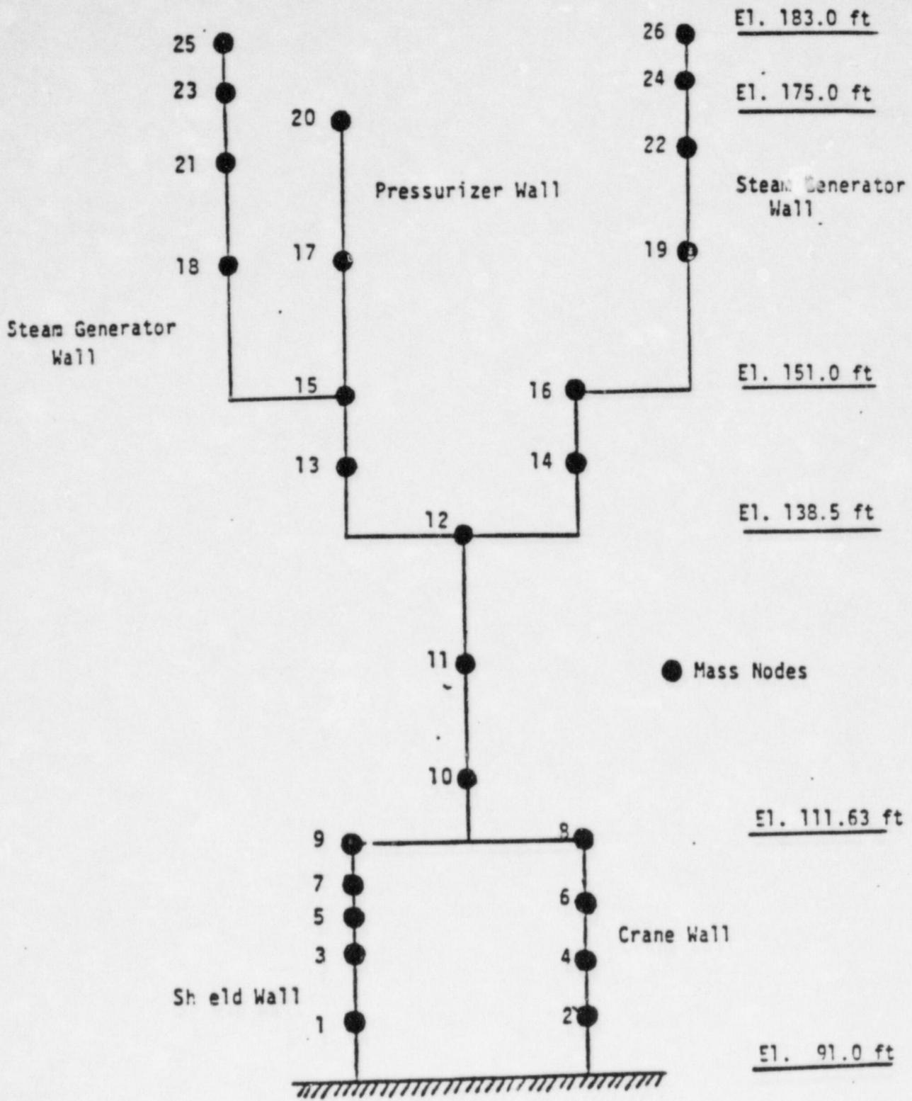
Fig. 2.8 2-D 26-Mass Multiple-Stick Model for Internal Structure (Ref. 3)
