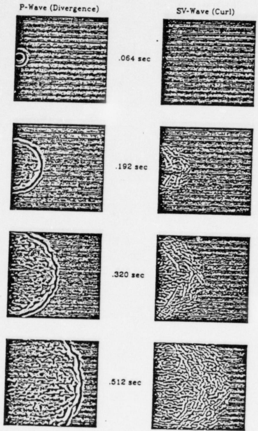
Figure 7: Time slices of the divergence (P waves) and curl (SV waves) for a wavefield propagating through the medium shown in Figure 6.
