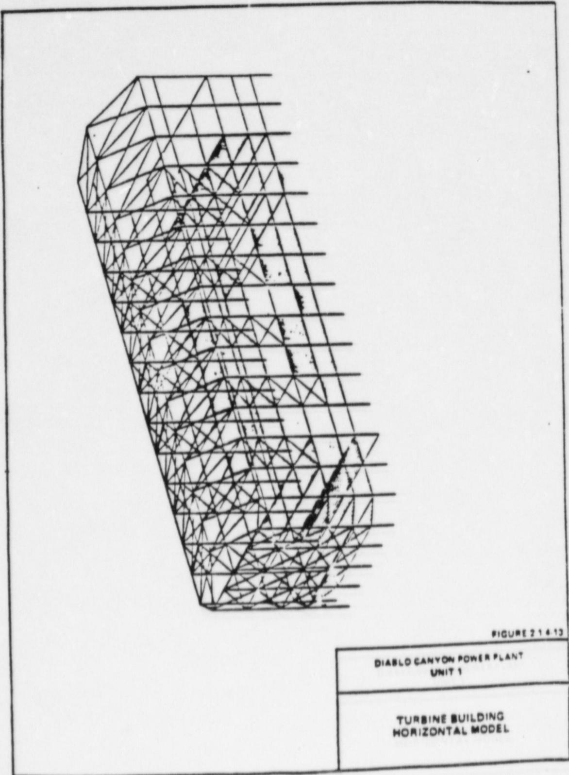
Fig. 4.7 3-D Detailed FEM Model for Unit 1 Turbine Building (Ref. 4)
