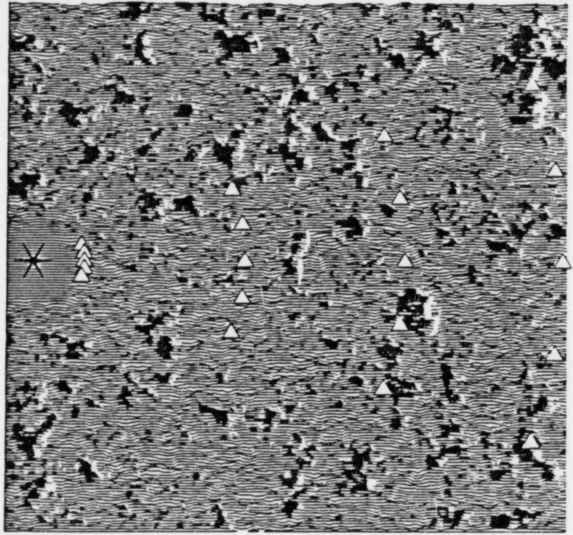
Figure 6: Typical velocity model used for random media studies. The star denotes the location of the explosion source and the triangles are the receivers. The medium has an exponential correlation function with a correlation distance of 80 m. The velocity variation are 10%.
