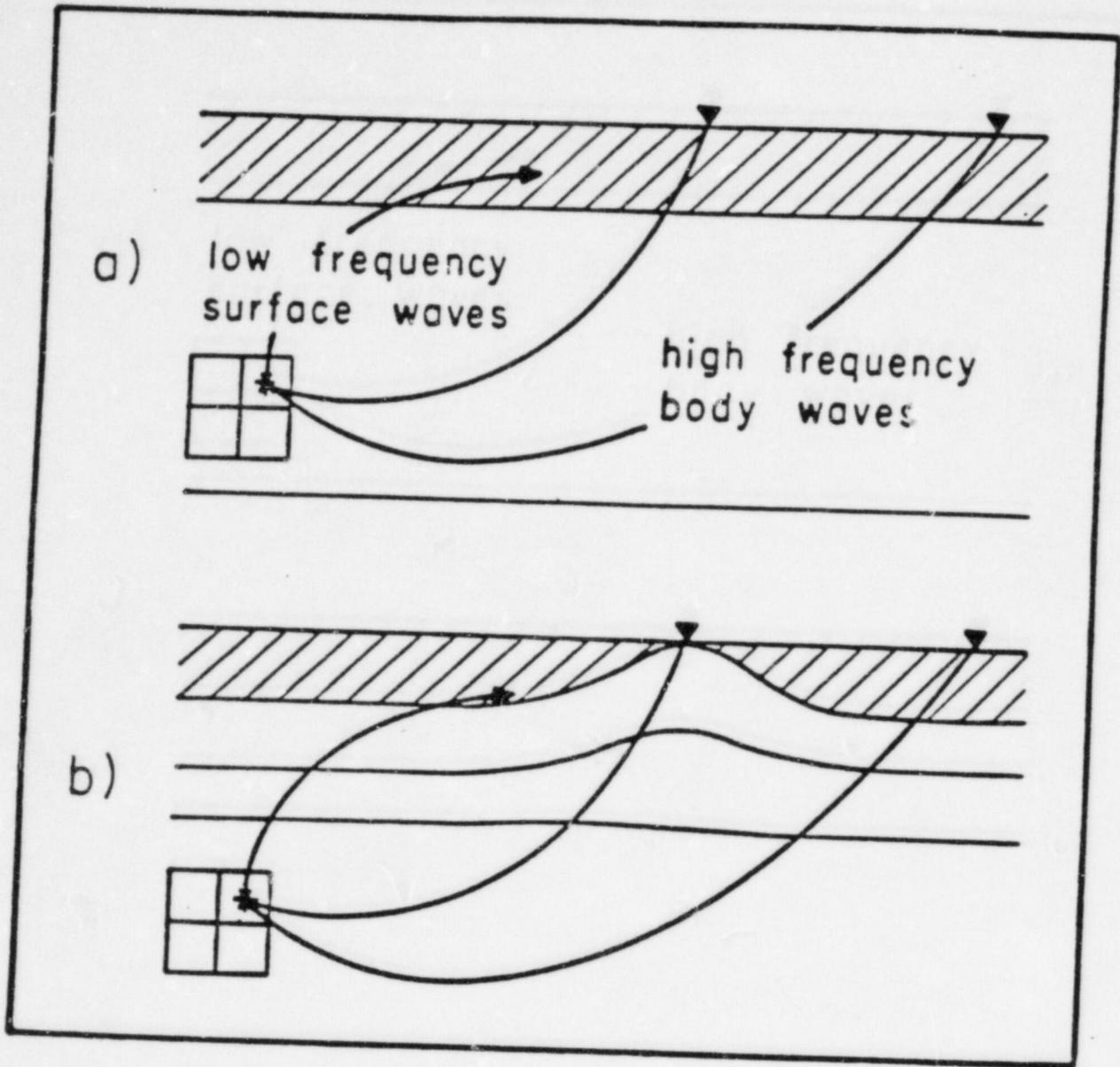
Figure 2: Schematic diagram displaying energy paths for a) flat-layered model versus b) laterally varying structure. The model is two-dimensional or constant properties into and out of the plane of the paper.
