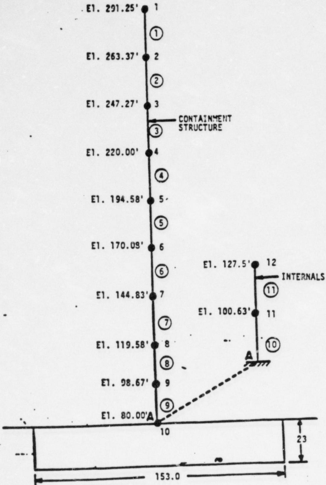
SSI ANALYSIS MODEL USED IN CLASSI AND SASSI ANALYSES AND IN SITE ROCK SENSITIVITY STUDIES
