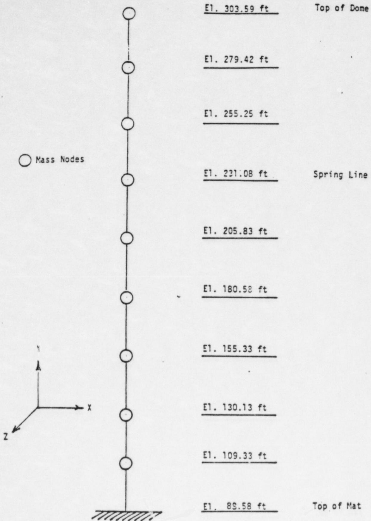
Fig. 2.7 9-Mass Stick Model for Exterior Shell (Ref. 2)
