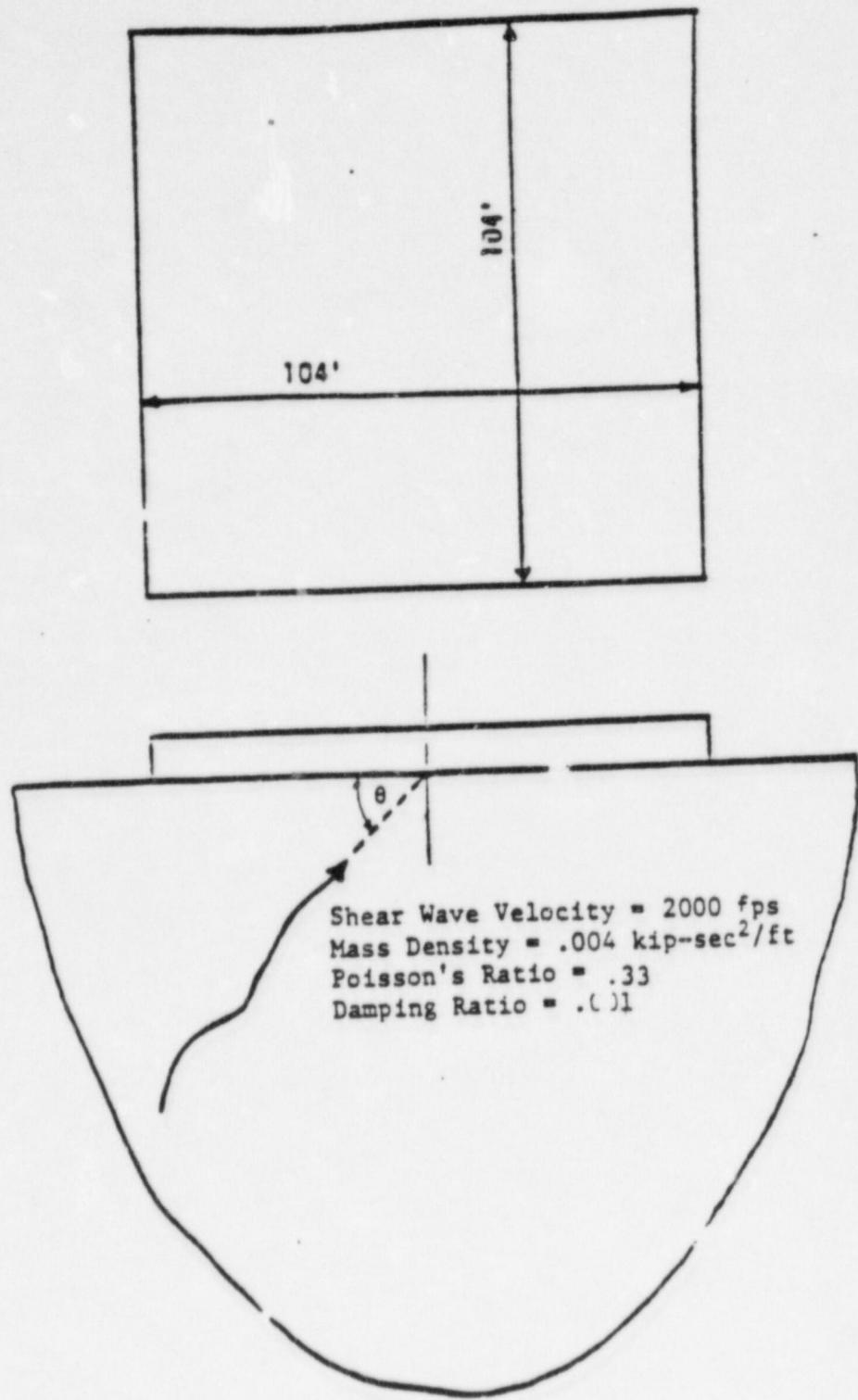
Fig. 4.2-3.1 Square Foundation on Elastic Half-space
