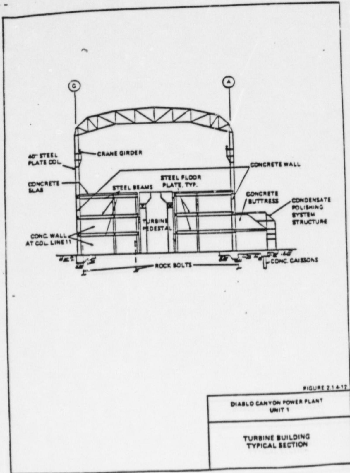
Fig. 4.6 Unit 1 Turbine Building, Transverse Section (Ref. 4)
