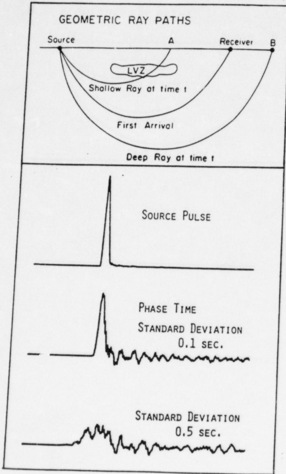
Figure 2. Degradation of a pulse by scattering of the phase.
