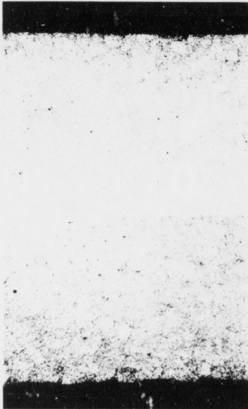
Figure 7. Typical edge view of section 2 removed from RHR pump "A" wear ring segment. The edge in the upper photo was adjacent to the wear surface and the edge in the lower photo was adjacent to the impeller.
