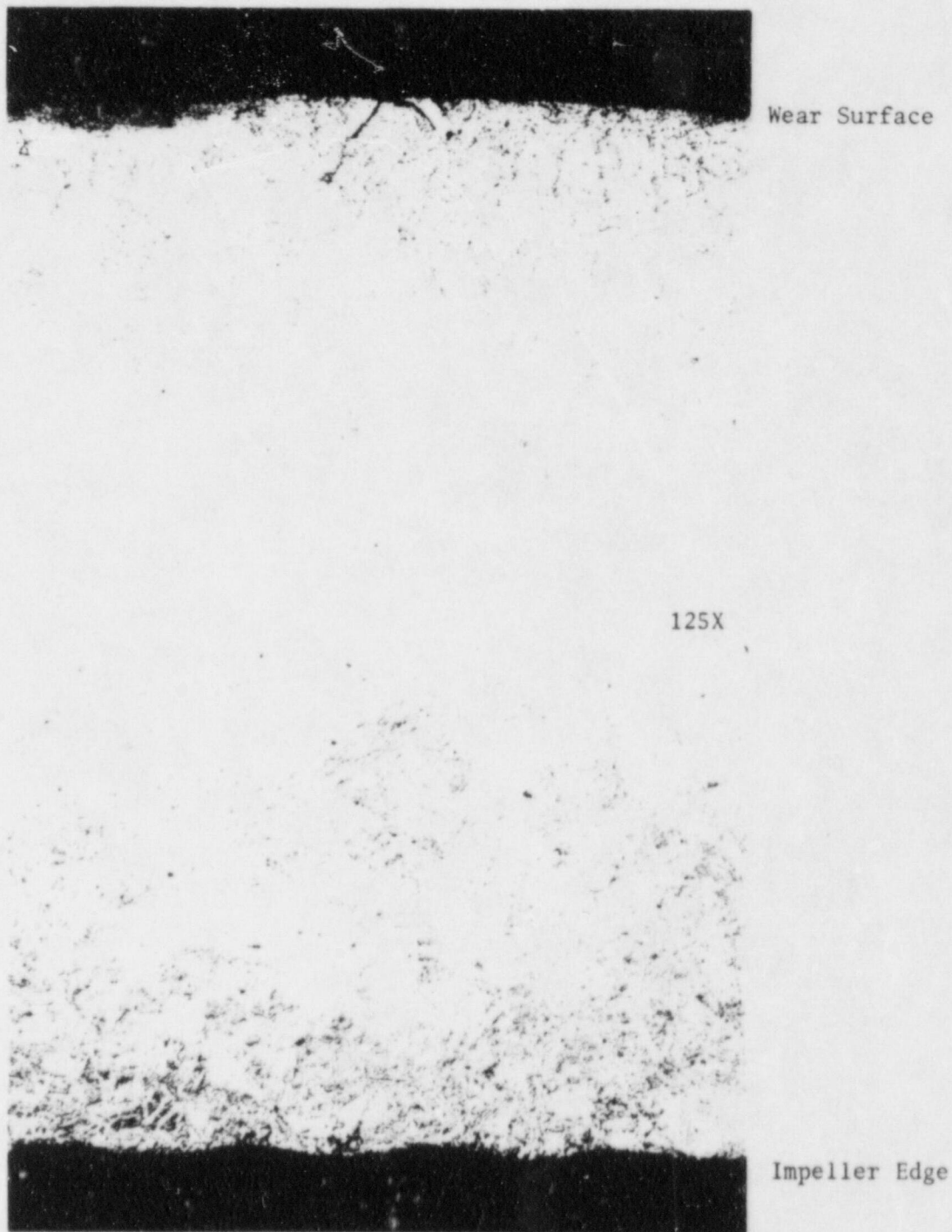
Figure 8. Typical edge views of section 3 removed from RHR pump "A" wear ring segment. The edge in the upper photo was adjacent to the wear surface and the edge in the lower photo was adjacent to the impeller. Note shallow intergranular crack in upper photo. Hardness at this location is approximately 43 Rockwell C.
