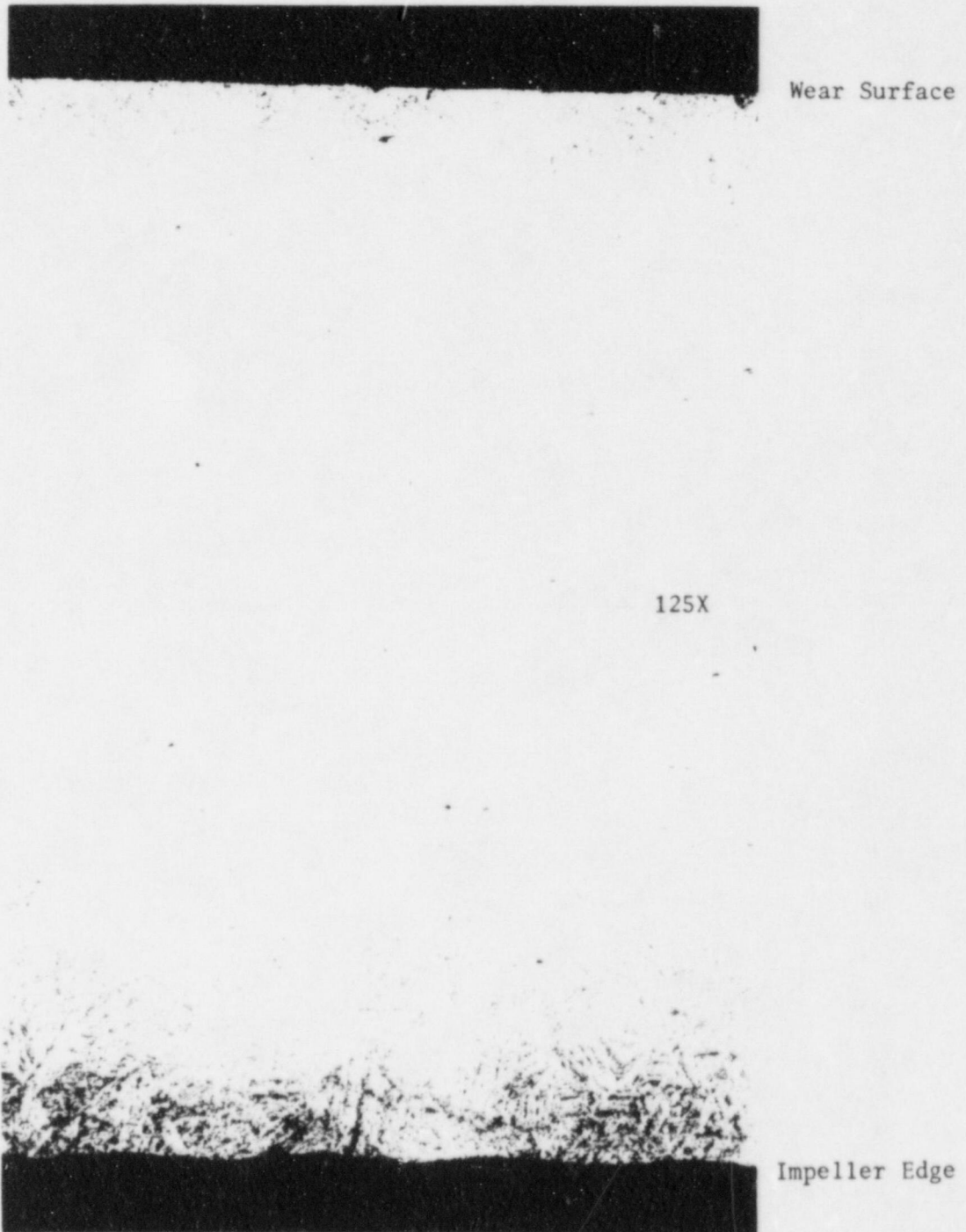
Figure 13. Typical edge view of section 1 removed from RHR pump "B" wear ring. The edge in the upper photo was adjacent to the wear surface and the edge in the lower photo was adjacent to the impeller.
