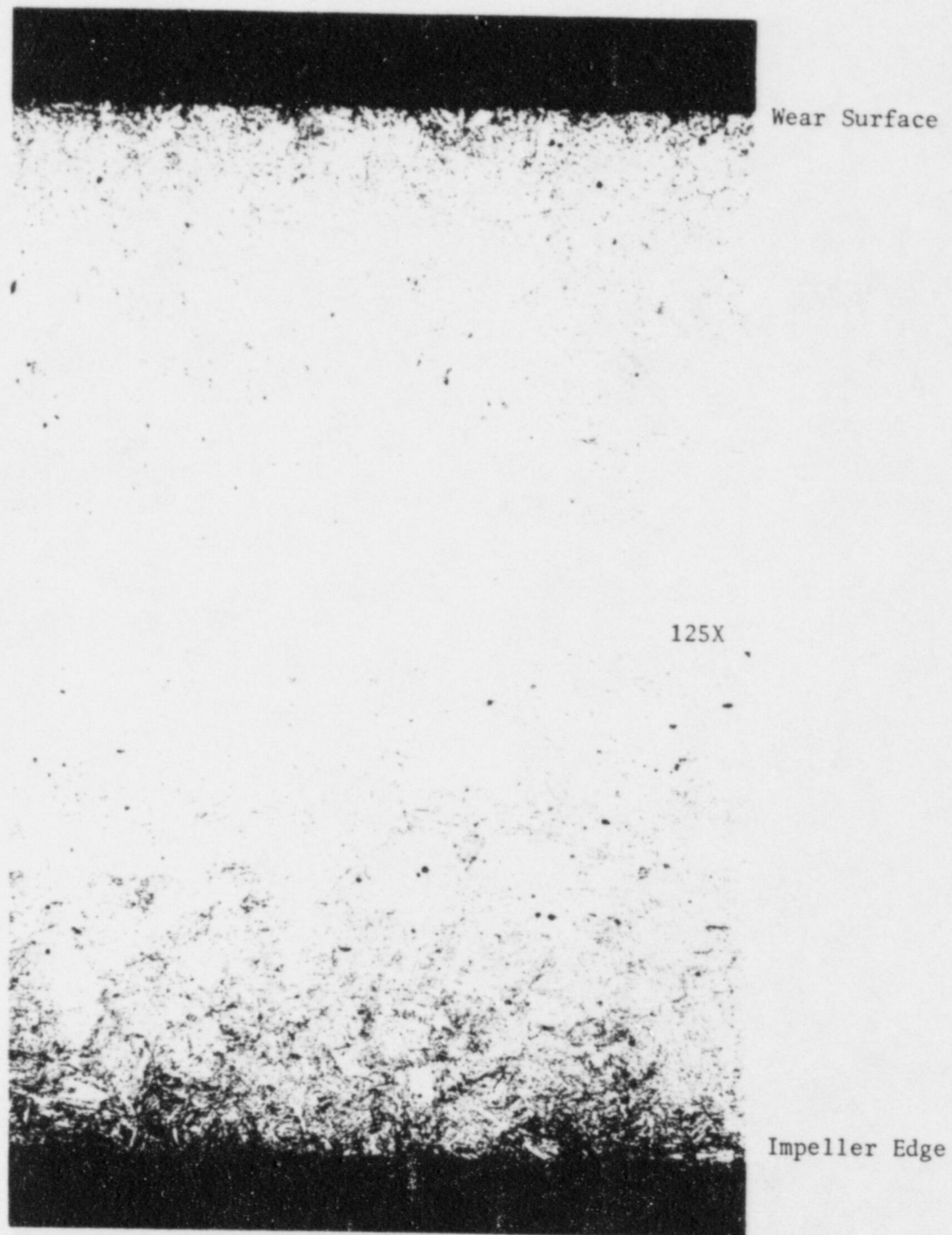
Figure 10. Typical edge views of section 5 removed from RHR pump "A" wear ring segment. The edge in the upper photo was adjacent to the wear surface and the edge in the lower photo was adjacent to the impeller.
