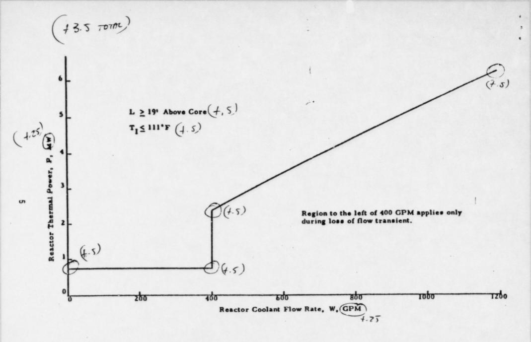
Figure 2.1 Safety limits with forced convection flow
