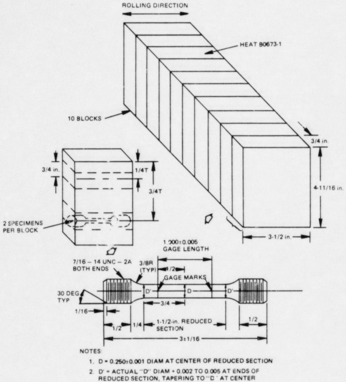
Figure 3-6. Fabrication Method for Base Metal Tensile Specimens
