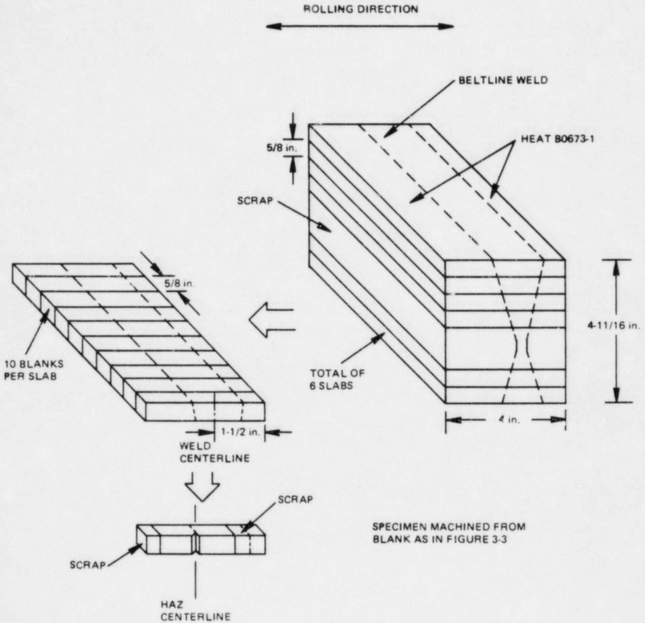
Figure 3-5. Fabrication Method for HAZ Charpy Specimens
