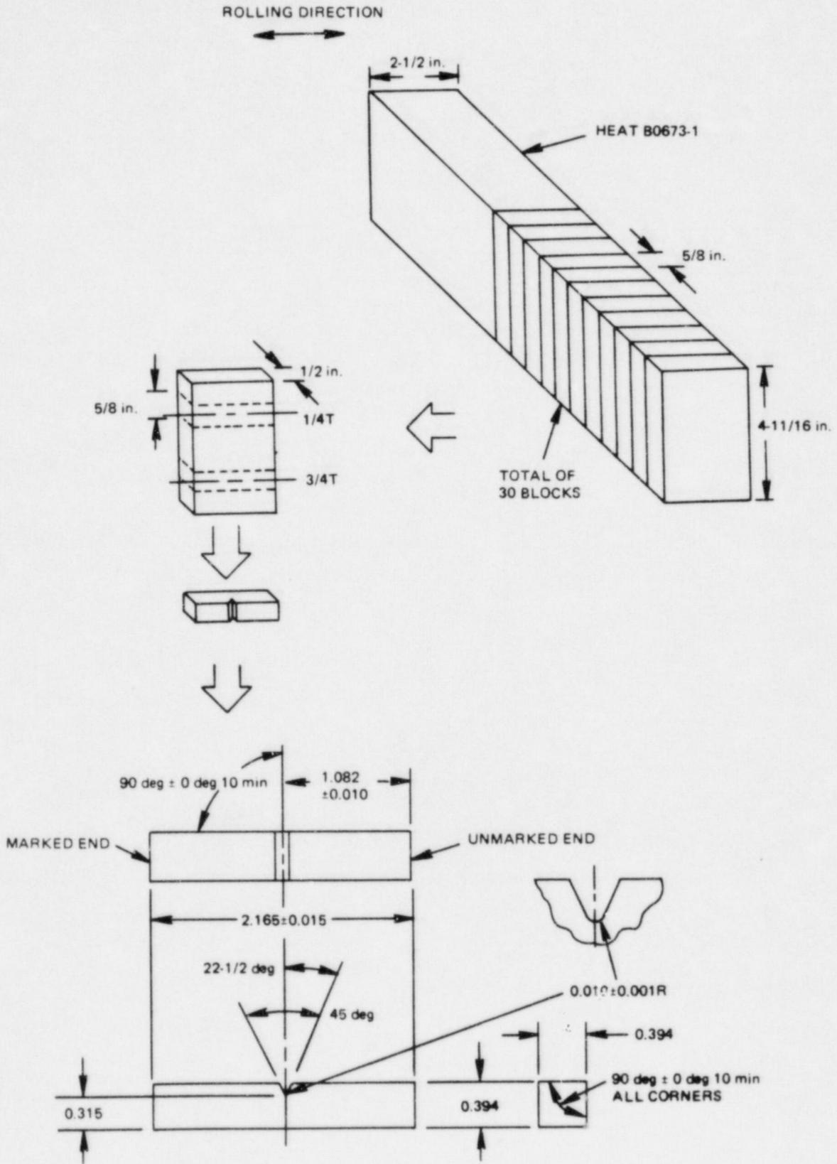
Figure 3-3. Fabrication Method for Base Metal Charpy Specimens
