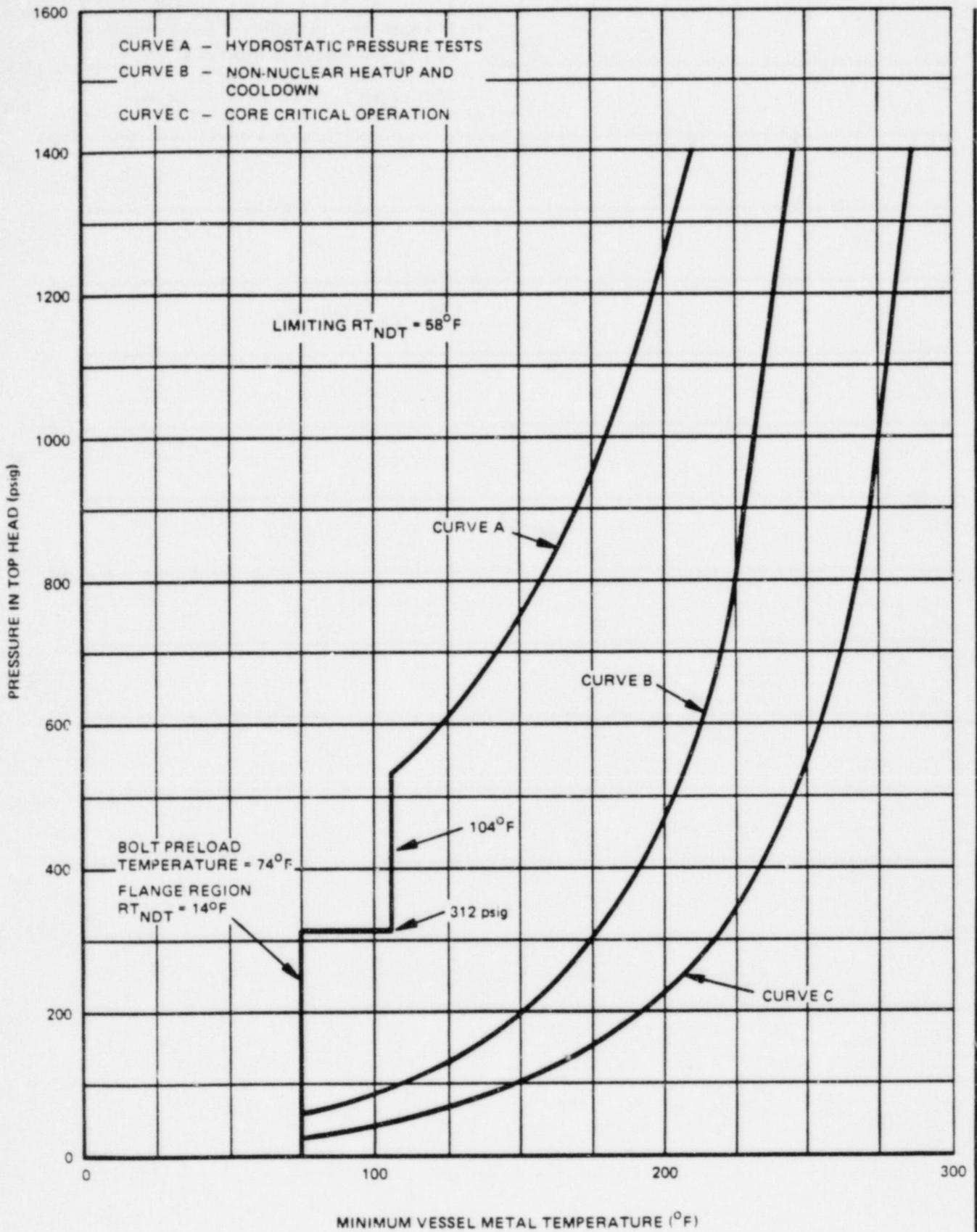
Figure 7-2. Pressure Versus Minimum Temperature, Valid to 12 EPFY
