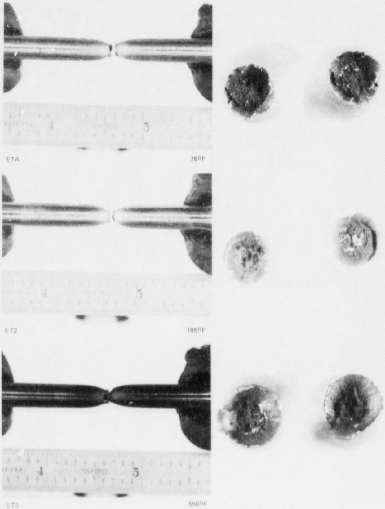
Figure 6-10. Fracture Location, Necking Behavior, and Fracture Appearance for Unirradiated Base Metal Tensile Specimens
