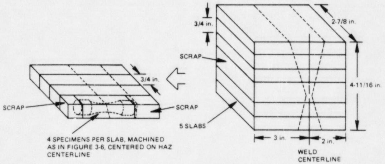
Figure 3-8. Fabrication Method for HAZ Tensile Specimens
