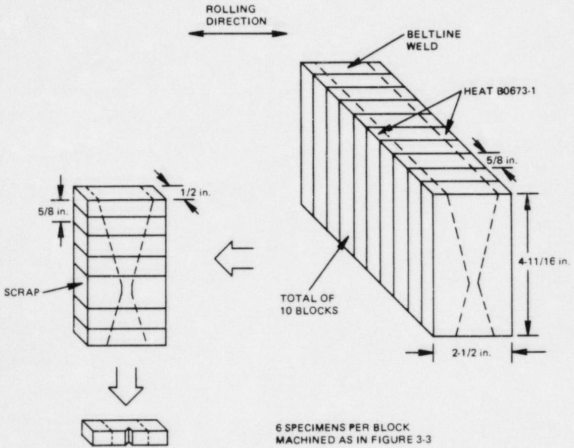
Figure 3-4. Fabrication Method for Weld Metal Charpy Specimens
