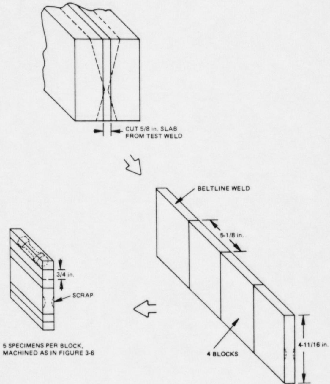
Figure 3-7. Fabrication Method for Weld Metal Tensile Specimens
