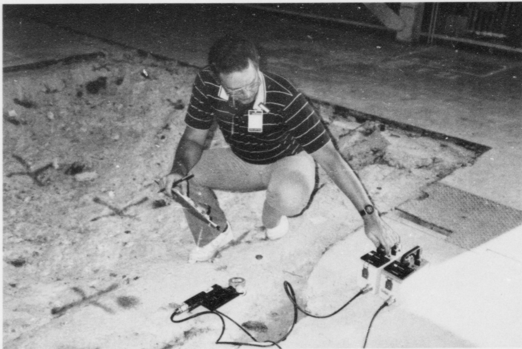
FIGURE 5: Direct Measurements of Floors and Lower Walls. Total alpha and beta-gamma contamination measurements were made using portable scalers and detectors. The grid system (X's on the floor) is visible in the remediated area of the concrete.
