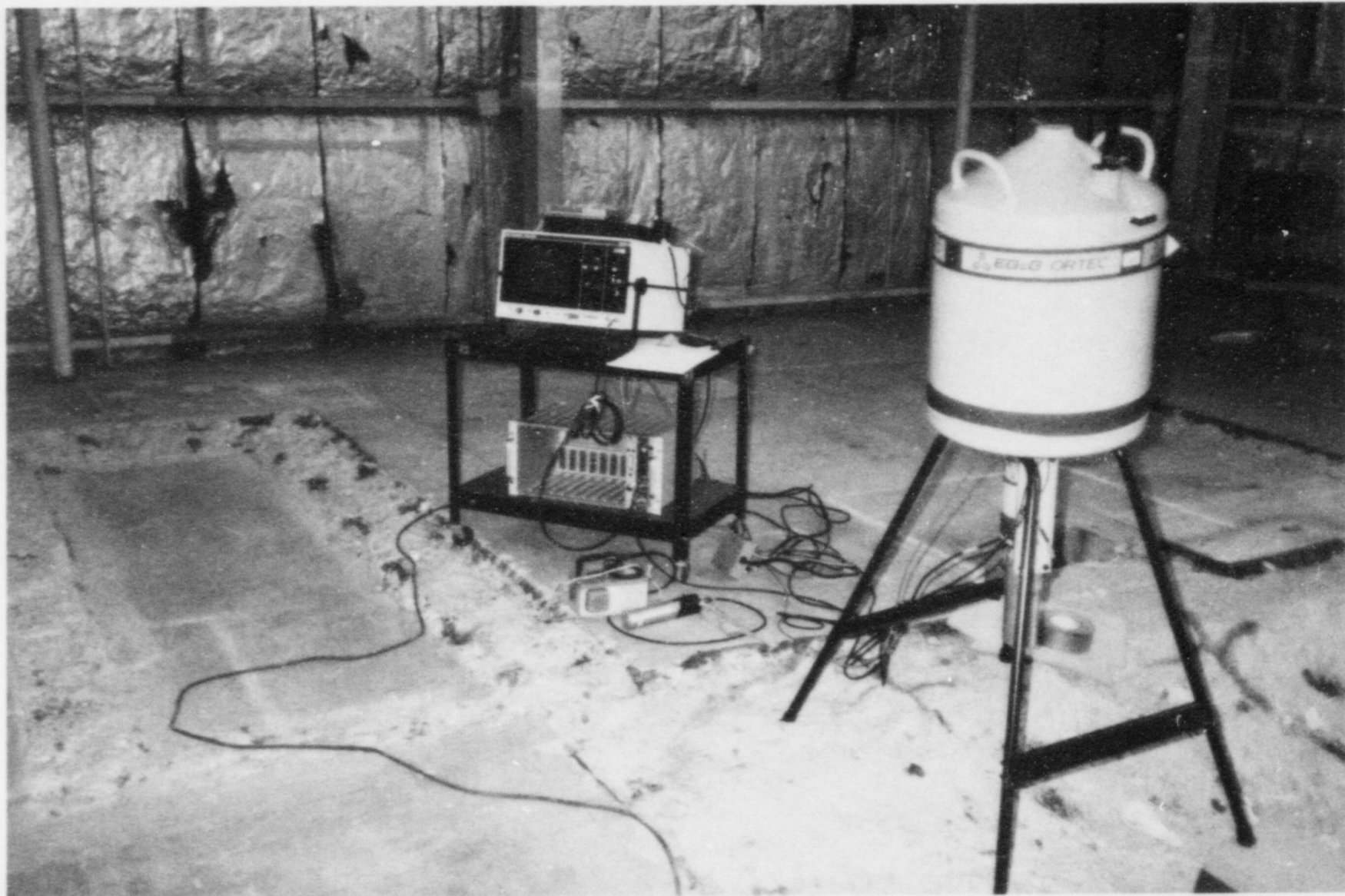
FIGURE 7: In-situ Gamma Spectrometry Measurements. Gamma spectra were collected at random locations and locations of elevated radiation levels, using a high purity germanium detector and 4096 channel pulse height analyzer.
