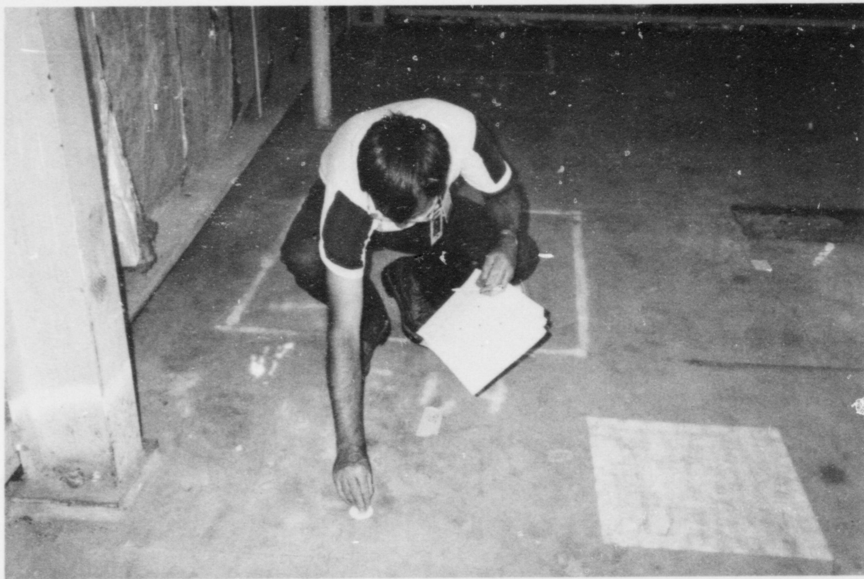
FIGURE 6: Transferable Contamination Surveys. Smears were taken at the location of the highest radiation measurement in each grid block.
