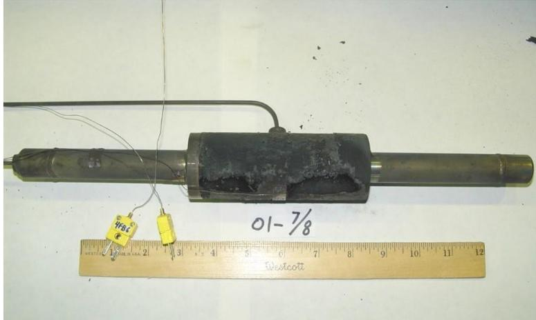
**Figure 7-32 Specimen 01-7/8 in the Post-test Condition**
