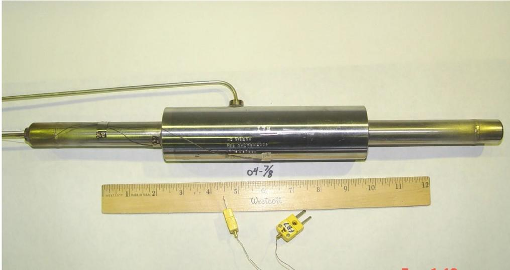
**Figure 7-10 Specimen 04-7/8 in the As-received Condition**
