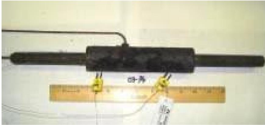
**Figure 7-35 Specimen 03-3/4 in the Post-test Condition**
