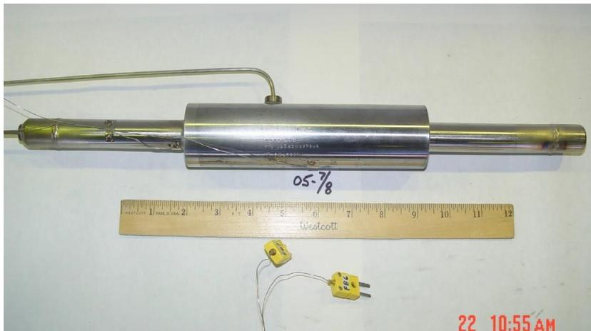
**Figure 7-13 Specimen 05-7/8 in the As-received Condition**
