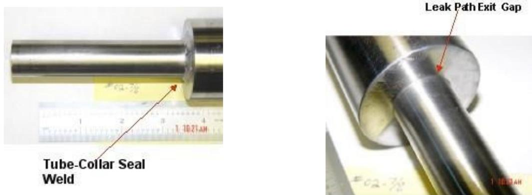
Figure 7-2 Close up Views of Leak Specimen Seal Weld and Leak Path Exit Gap of Specimen 10-7/8
