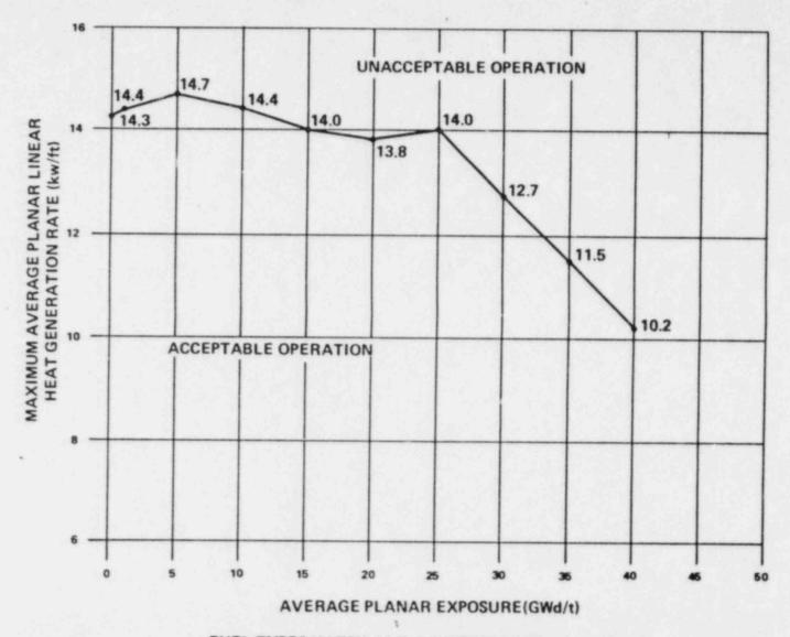
FUEL TYPES HATCH-1 I.C. 1.2,3 (7X7) 80 MIL CHANNELS MAXIMUM AVERAGE PLAN, CINEAR HEAT GENERATION RATE (MPALHGR) VERSUS AVERAGE PLANAR EXPOSURE F:GURE 3.2.1-6
