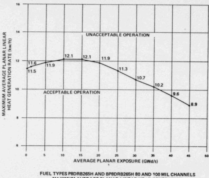
UEL TYPES P8DRB265H AND BP8DRB265H 80 AND 100 MIL CHANNEL MAXIMUM AVERAGE PLANAR LINEAR HEAT GENERATION RATE (MAPLHGR) VERSUS AVERAGE PLANAR EXPOSURE FIGURE 3.2.1-7
