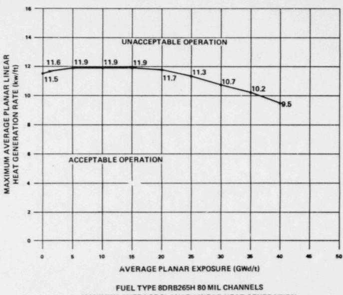
MAXIMUM AVERAGE PLANAR LINEAR HEAT GENERATION RATE (MAPLHGR) VERSUS AVERAGE PLANAR EXPOSURE FIGURE 3.2.1-8
