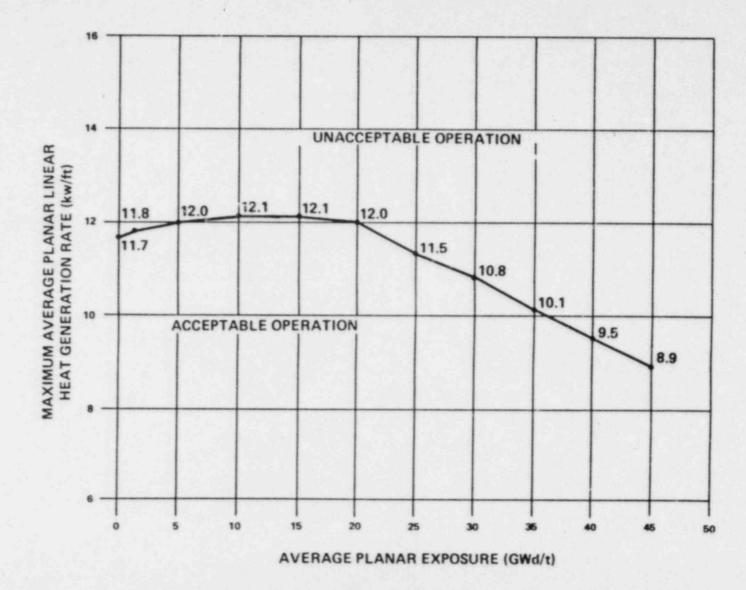
FUEL TYPES P8DRB284LA AND BP8DRB284LA 100 MIL CHANNELS MAXIMUM AVERAGE PLANAR LINEAR HEAT GENERATION RATE (MAFLHGR) VERSUS PLANAR EXPOSURE FIGURE 3.2.1-4
