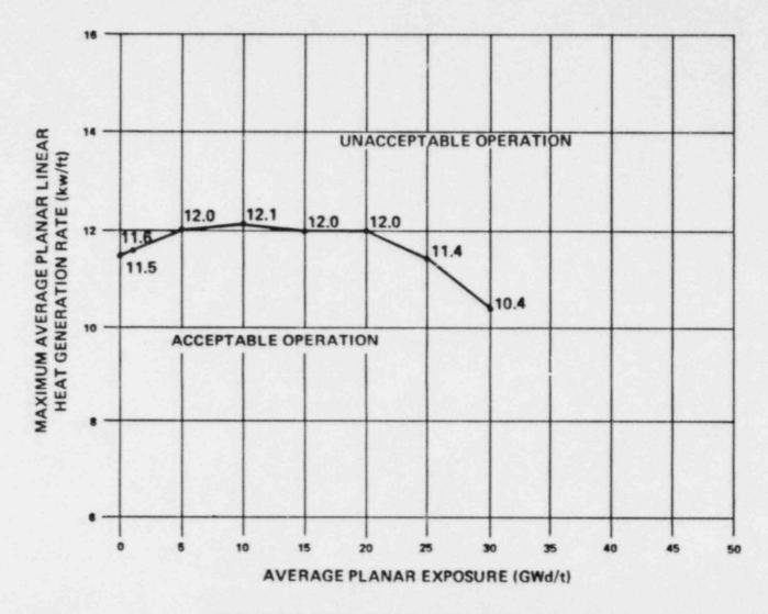
FUEL TYPE 8DIB175 (8DRL183) 100 MIL CHANNELS MAXIMUM AVERAGE PLANAR LINEAR HEAT GENERATION RATE (MAPLHGR) VERSUS AVERAGE PLANAR EXPOSURE FIGURE 3.2.1-1
