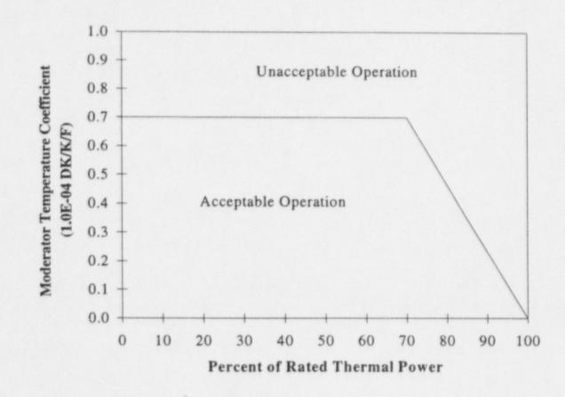
NOTE: Compliance with Technical Specification 3.1.3 may require rod withdrawal limits. Refer to the Unit 1 ROD manual for details.
