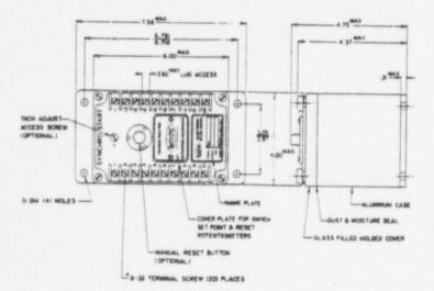
The model ESSB Electronic Speed Switch has many years of proven service. It is engineered to provide a wide variety of features and options including up to four switch points, adjustable reset, a selection of voltage inputs and DC current for tachometers.
