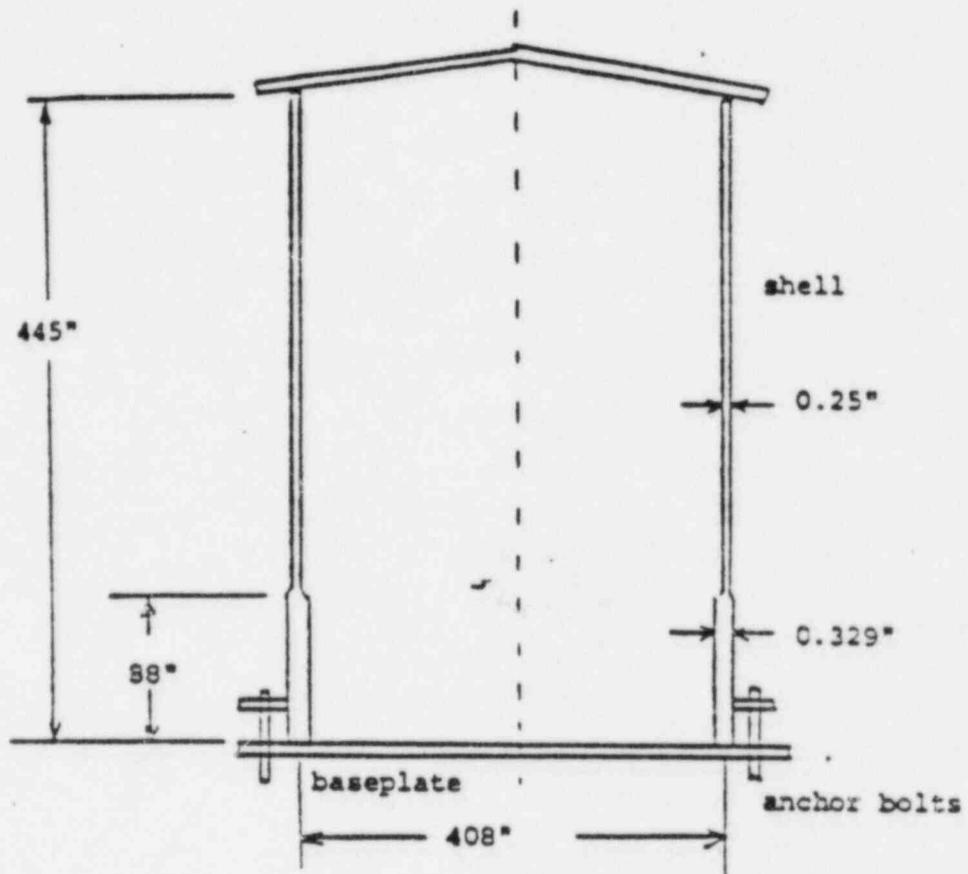
Figure 1. The refueling water storage tank.
