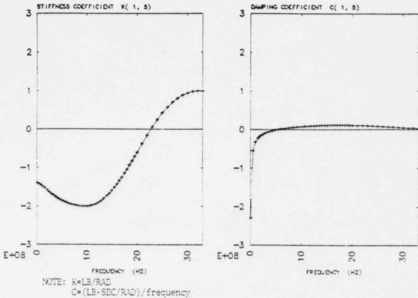
Figure 7. Translation/Rocking coupling impedances K(1,5) and C(1,5).
