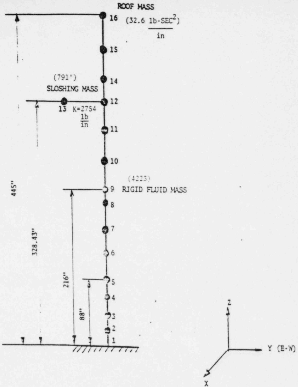
Figure 3. Mathematical model of the refueling water storage tank.
