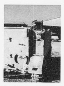
The ACADA mounted on a Bradley at Yuma, Arizona and tested in temperatures of up to 120°F.
